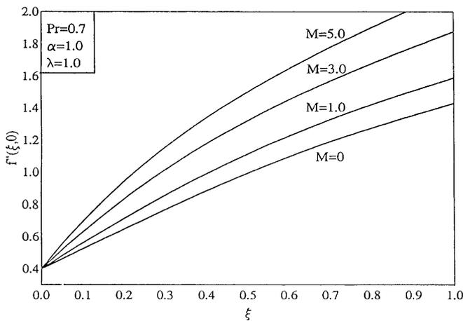
Fig. 2. Effect of the magnetic parameter  $M$  on the surface shear stress in the  $x$  direction,  $f''(\xi, 0)$
