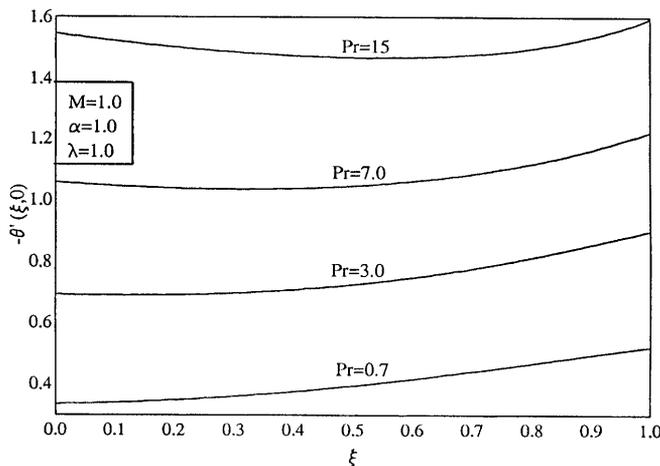
Fig. 13. Effect of the Prandtl number Pr on the surface heat transfer,  $-\theta'(\xi, 0)$
