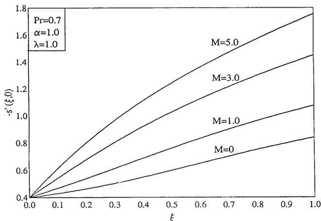
Fig. 3. Effect of the magnetic parameter  $M$  on the surface shear stress in the  $y$  direction,  $-s'(\xi, 0)$
