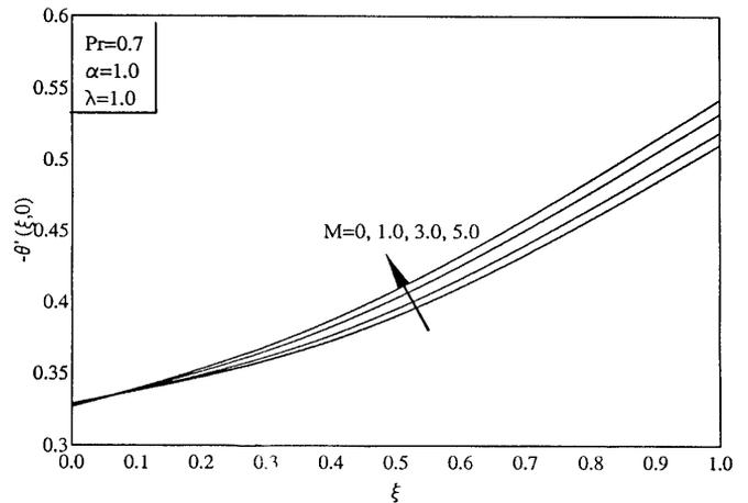
Fig. 4. Effect of the magnetic parameter  $M$  on the surface heat transfer,  $-\theta'(\xi, 0)$
