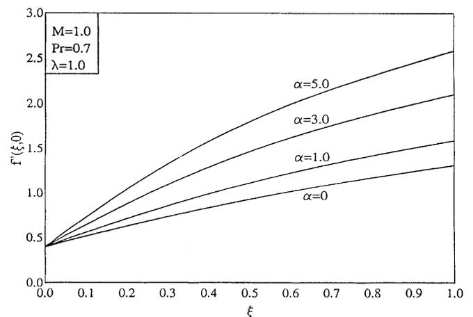
Fig. 5. Effect of the buoyancy parameter  $\alpha$  on the surface shear stress in the  $x$  directions,  $f''(\xi, 0)$
