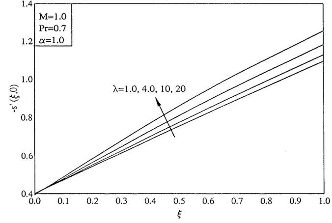
Fig. 9. Effect of the rotation parameter  $\lambda$  on the surface shear stress in the  $y$  direction,  $-s'(\xi, 0)$
