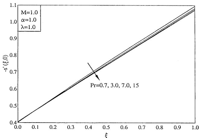
Fig. 12. Effect of the Prandtl number Pr on the surface shear stress in the  $y$  direction,  $-s'(\xi, 0)$
