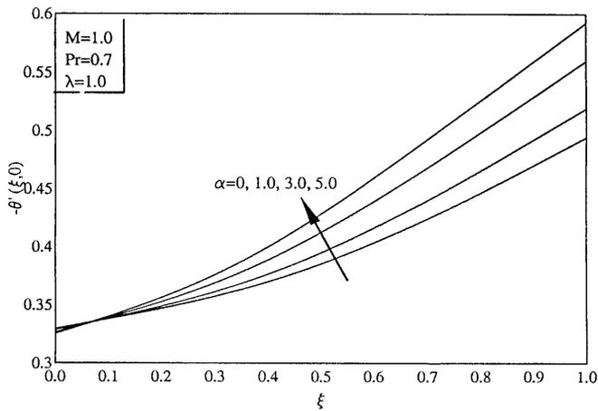
Fig. 7. Effect of the buoyancy parameter  $\alpha$  on the surface heat transfer,  $-\theta'(\xi, 0)$
