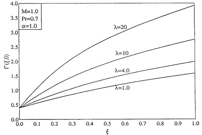
Fig. 8. Effect of the rotation parameter  $\lambda$  on the surface shear stress in the  $x$  direction,  $f''(\xi, 0)$
