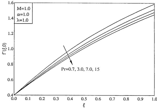
Fig. 11. Effect of the Prandtl number Pr on the surface shear stress in the  $x$  direction,  $f''(\xi, 0)$
