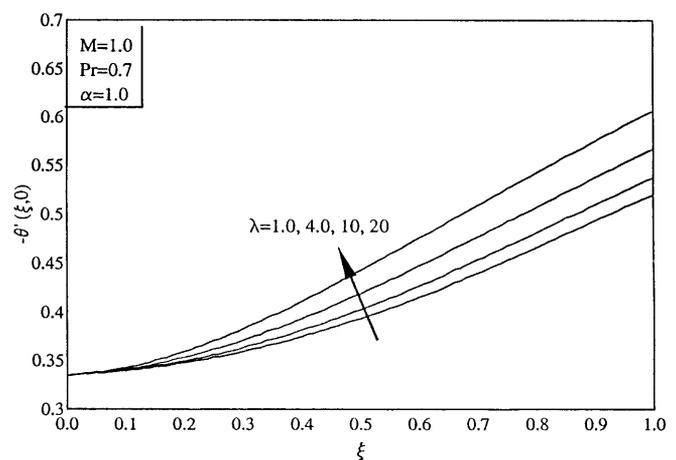
Fig. 10. Effect of the rotation parameter  $\lambda$  on the surface heat transfer,  $-\theta'(\xi, 0)$
