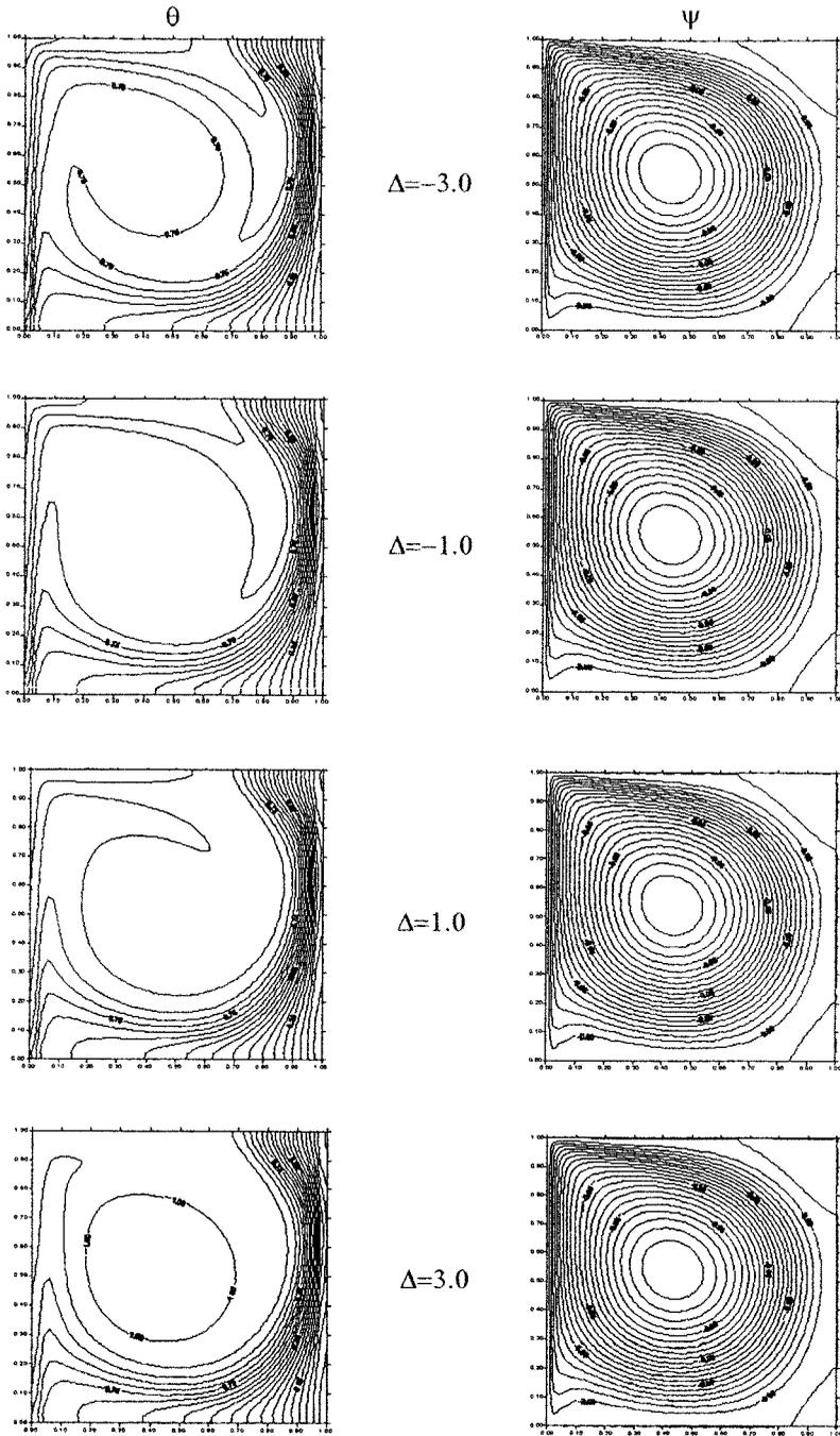
Figure 5. Effects of  $\Delta$  on the streamlines and isotherms for aiding flow (Case 2),  $Gr = 100$ ,  $Ha = 0$ ,  $Pr = 0.71$ , and  $Re = 1000$ .
