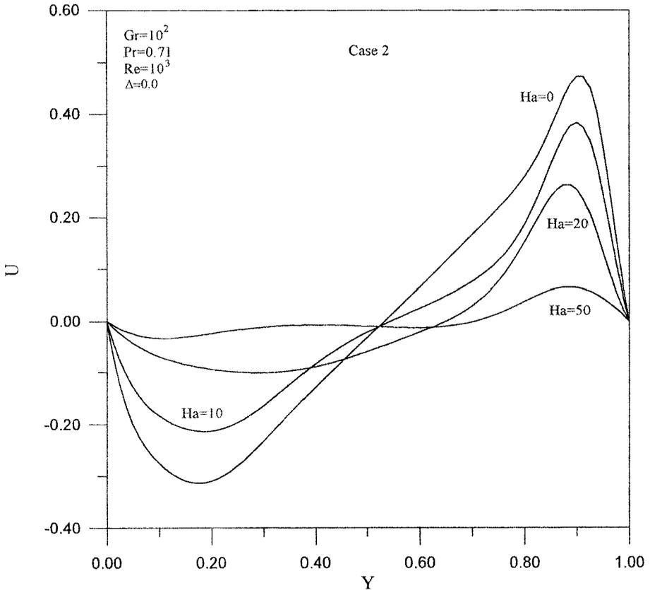
Figure 6. Effects of  $Ha$  on horizontal velocity profiles at enclosure midsection.
