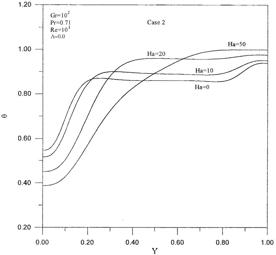
**Figure 8.** Effects of  $Ha$  on temperature profiles at enclosure midsection.
