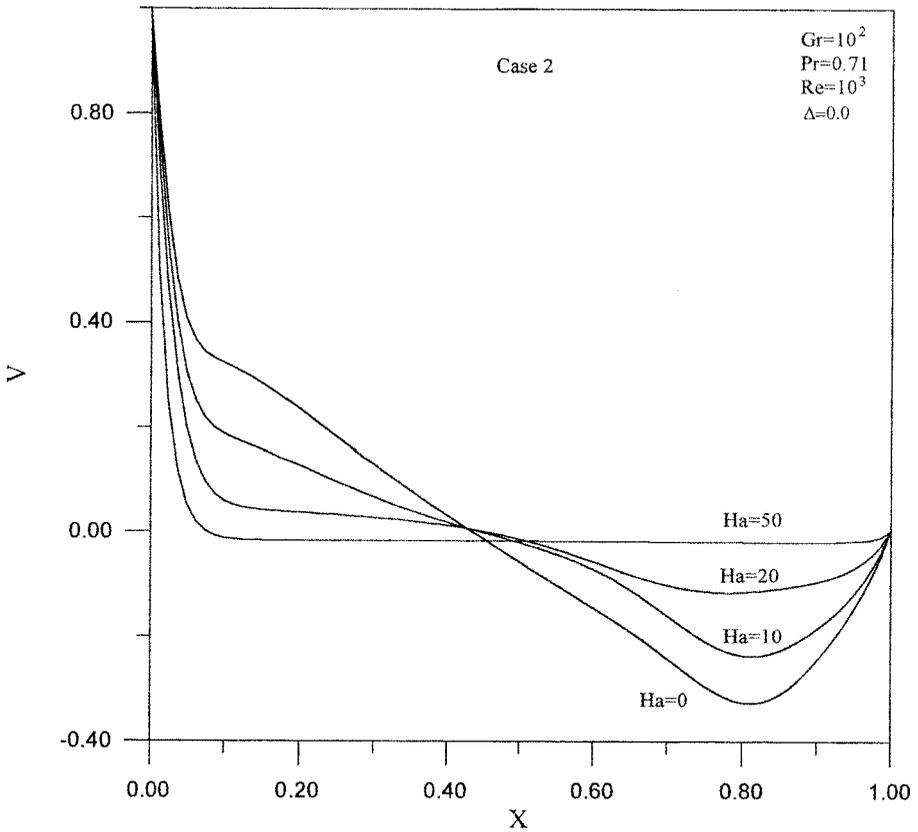
Figure 7. Effects of  $Ha$  on vertical velocity profiles at enclosure midsection.
