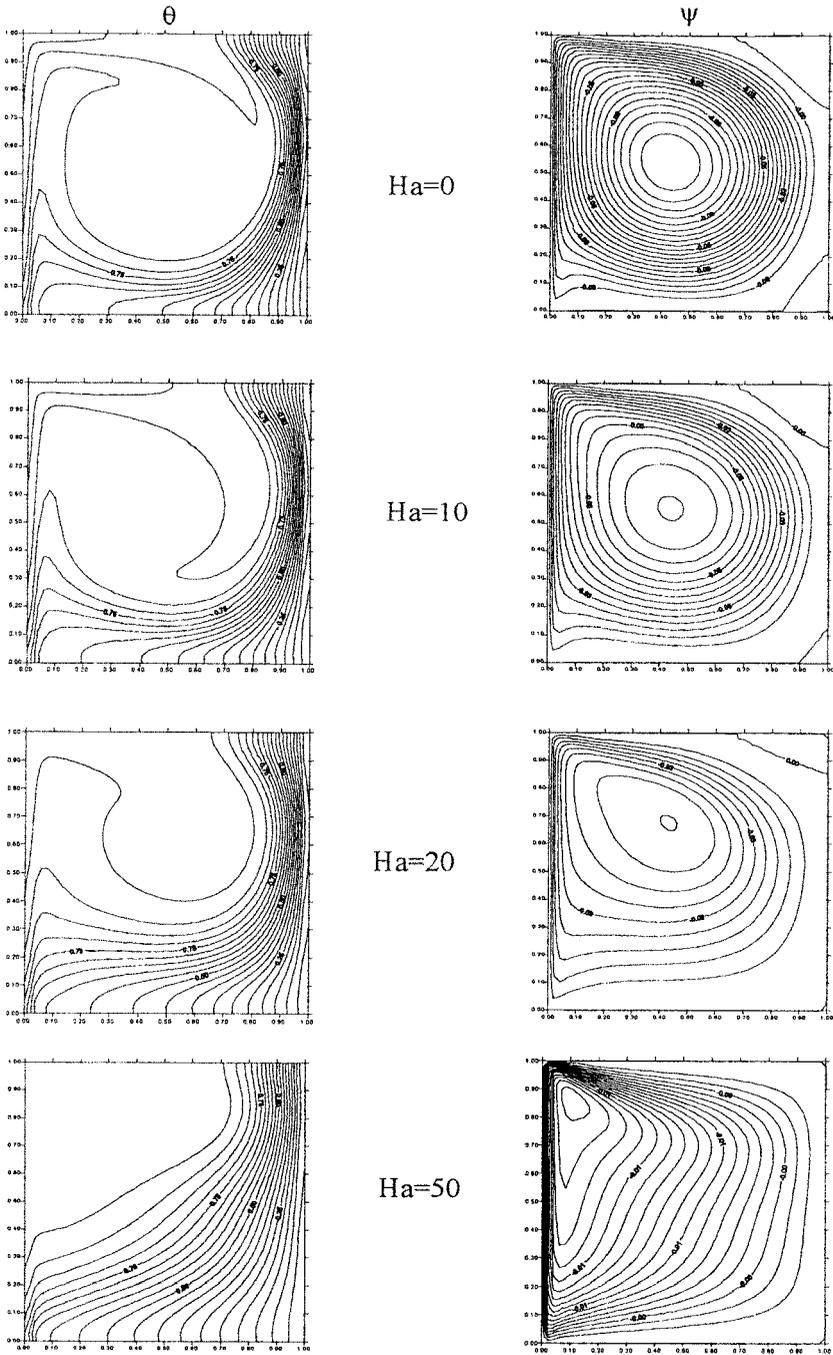
Figure 4. Effects of  $Ha$  on the streamlines and isotherms for aiding flow (Case 2),  $Gr = 100$ ,  $Pr = 0.71$ ,  $Re = 1000$ , and  $\Delta = 0$ .
