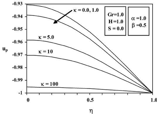
Fig. 11. Effects of  $\kappa$  on particle-phase velocity profiles
