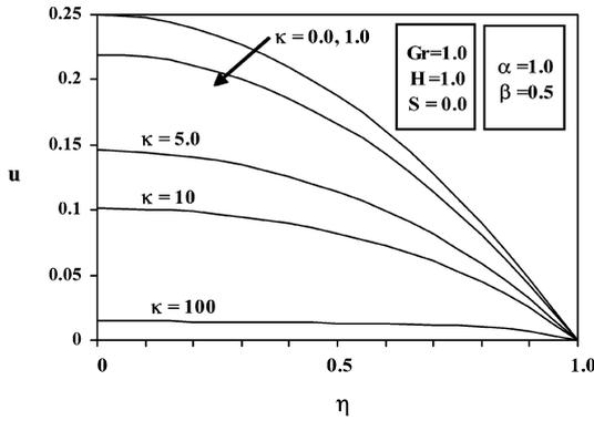
Fig. 10. Effects of  $\kappa$  on fluid-phase velocity profiles
