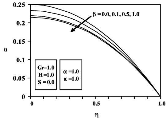
Fig. 4. Effects of  $\beta$  on fluid-phase velocity profiles
