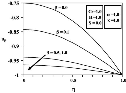
Fig. 5. Effects of  $\beta$  on particle-phase velocity profiles
