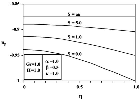
Fig. 7. Effects of  $S$  on particle-phase velocity profiles
