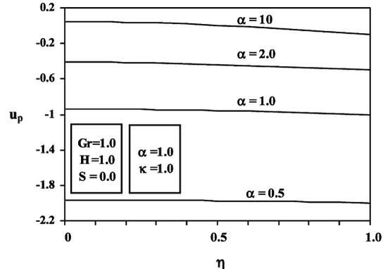
Fig. 9. Effects of  $\alpha$  on particle-phase velocity profiles
