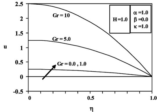
Fig. 2. Effects of  $Gr$  on fluid-phase velocity profiles
