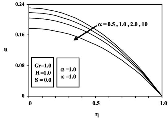
Fig. 8. Effects of  $\alpha$  on fluid-phase velocity profiles
