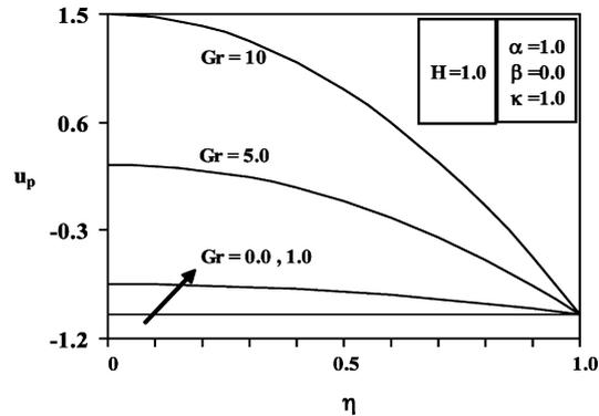
Fig. 3. Effects of  $Gr$  on particle-phase velocity profiles
