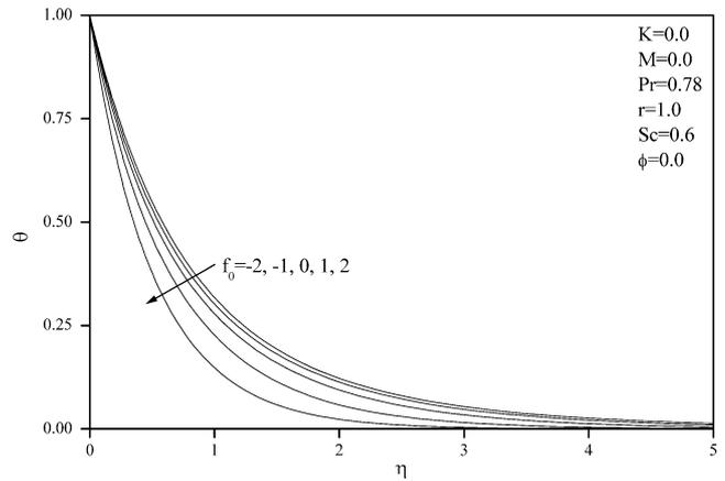
Fig. 5 Effects of  $f_0$  on temperature profiles
