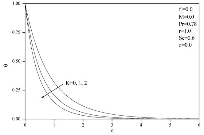
Fig. 11 Effects of  $K$  on temperature profiles
