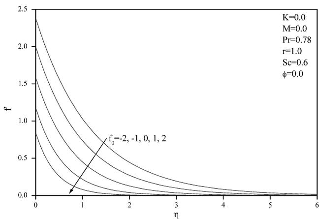
Fig. 4 Effects of  $f_0$  on velocity profiles
