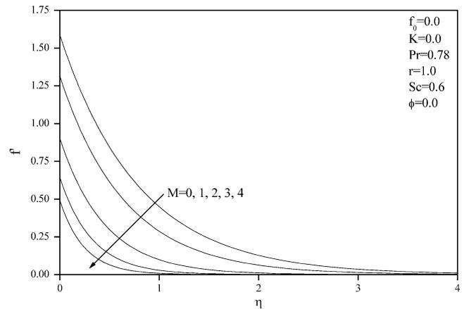
Fig. 1 Effects of  $M$  on velocity profiles
