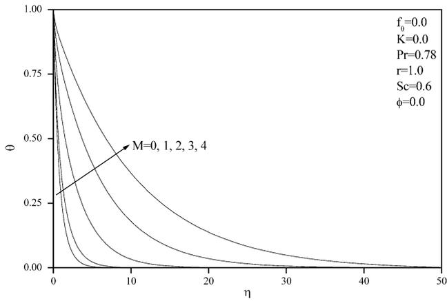
Fig. 2 Effects of  $M$  on temperature profiles
