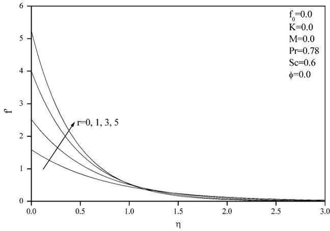
Fig. 8 Effects of  $r$  on velocity profiles
