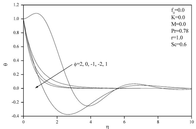
Fig. 7 Effects of  $\phi$  on temperature profiles
