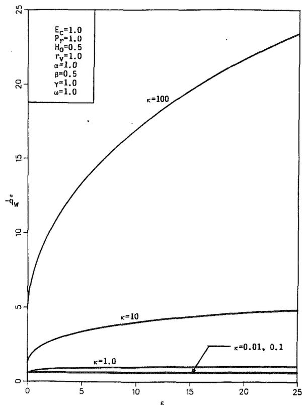
Fig. 4 Wall heat flux coefficient versus  $\epsilon$
