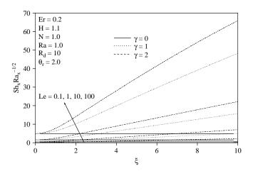
increase in the Lewis number decreases the heat transfer coefficient, where as it increases the mass transfer coefficient.
