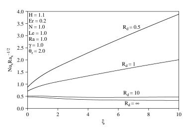
$\begin{array}{c} \textbf{Figure 16.} \\ \text{Effects of } R_d \text{ on local} \\ \text{Nusselt number} \end{array}$
