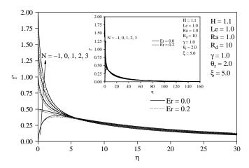
**Figure 10.** Effects of Er and N on velocity profiles
