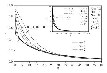
Figure 5. Effects of Le and  $\gamma$  on velocity profiles
