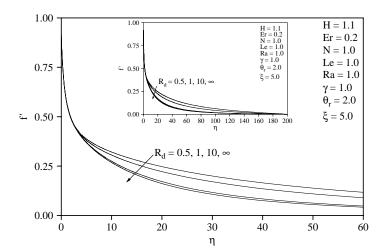
Figure 14. Effects of  $R_d$  on velocity profiles
