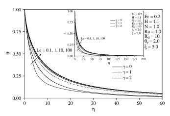
Figure 6. Effects of Le and  $\gamma$  on temperature profiles
