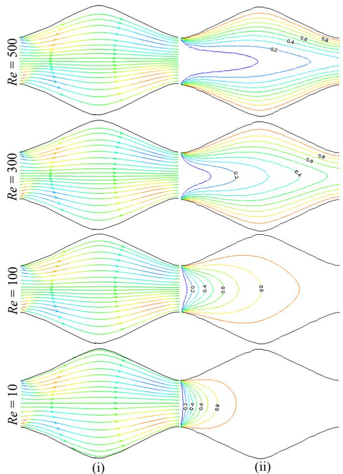
Fig. 4: Effect of  $Re$  on (i) streamlines and (ii) isotherms at  $\phi = 5\%$  and  $Da = 100$
