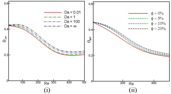
Fig. 6: Average bulk temperature for the effect of (i)  $Da$  and (ii)  $\phi$  with various  $Re$
