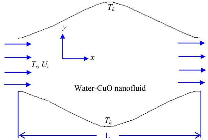
Fig. 1: Depiction of geometry and operation of the channel
