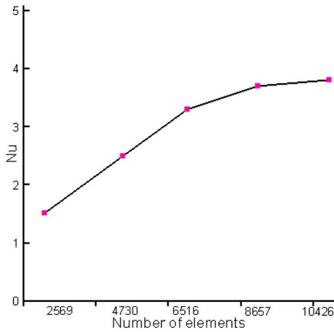
Fig. 2: Grid independency study for  $Da = 100$ ,  $Re = 100$  and  $\phi = 5\%$
