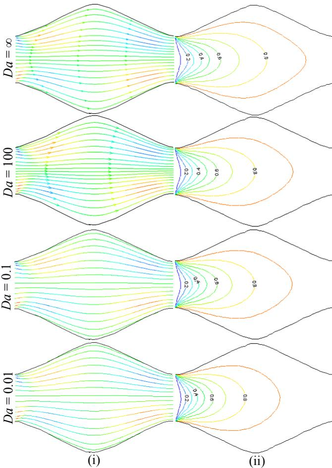
Fig. 5: Effect of  $Da$  on (i) streamlines and (ii) isotherms at  $Re = 100$  and  $\phi = 5\%$
