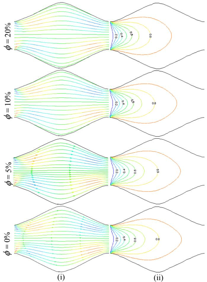
Fig. 7: Effect of  $\phi$  on (i) streamlines and (ii) isotherms at  $Re = 100$  and  $Da = 100$
