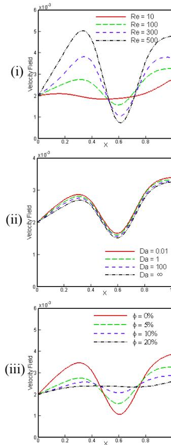
Fig. 9: Mid height velocity for different (i)  $Re$ , (ii)  $Da$  and (iii)  $\phi$  along  $X$  direction
