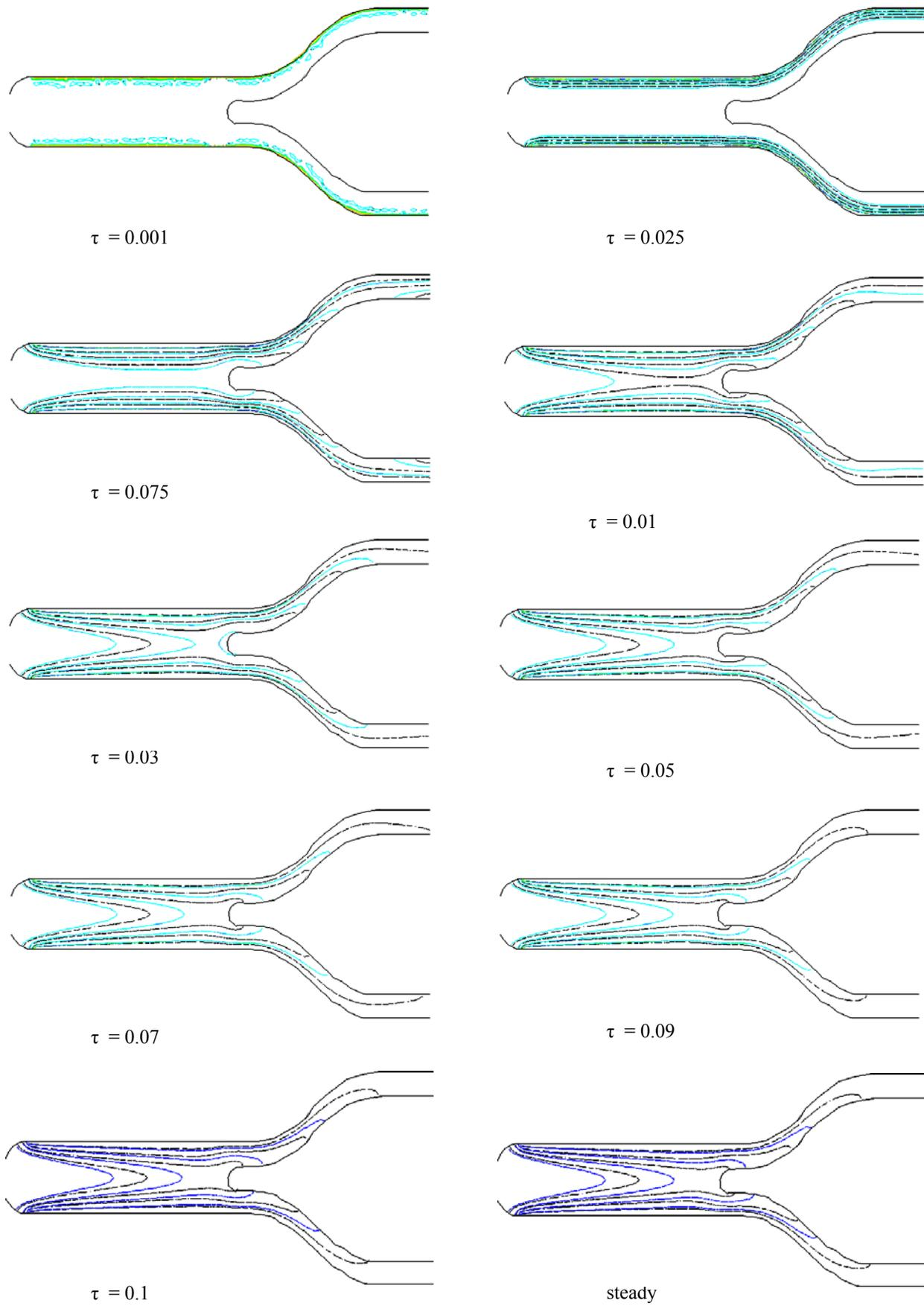
**Fig. 7: Transient behavior of isotherms at  $Pr = 1.47$  (solid lines for nanofluid and dashed lines for base fluid)**
