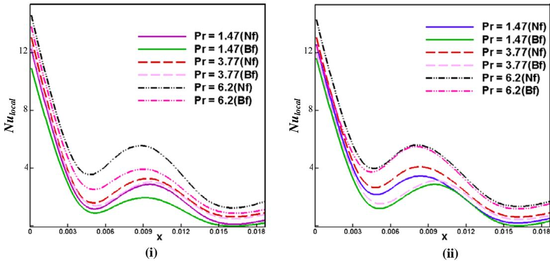
Fig. 10: Effect of  $Pr$  on local Nusselt number at (i) upper phase and (ii) lower phase (Nf = nanofluid, Bf = base fluid)
