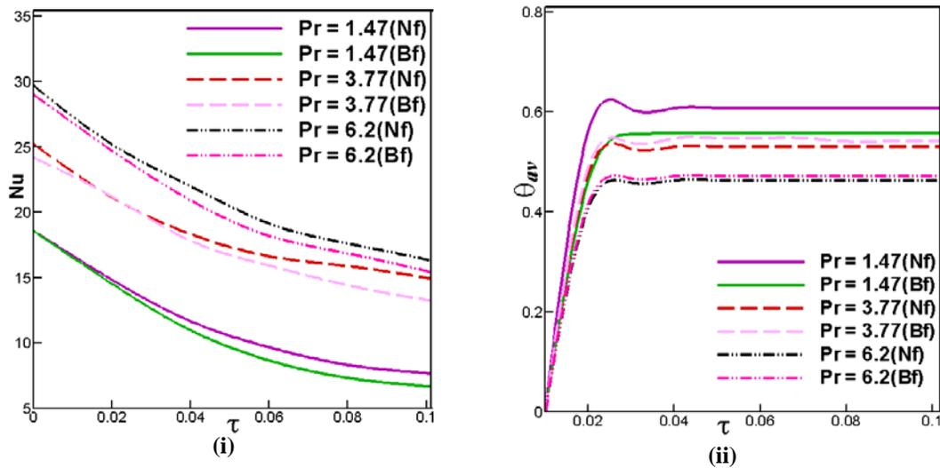
Fig. 11: Effect of  $Pr$  on (i)  $Nu$  and (ii)  $\theta_{av}$  (Nf = nanofluid, Bf = base fluid)
