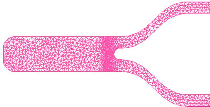
**Fig. 2: Mesh generation of the fluid valve**
