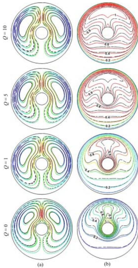
Fig. 5. Effect of  $Q$  on (a) streamlines and (b) isotherms with  $Dp = 5$ ,  $D = 0.2$  (colored lines for Pak and Cho model and black lines for Brinkman model). [Color figure can be viewed in the online issue, which is available at [wileyonlinelibrary.com/journal/htj](http://wileyonlinelibrary.com/journal/htj).]
