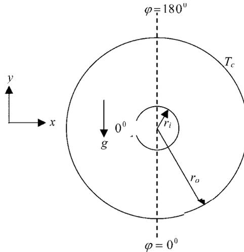
Fig. 1. Schematic diagram of the annulus and coordinate system.
