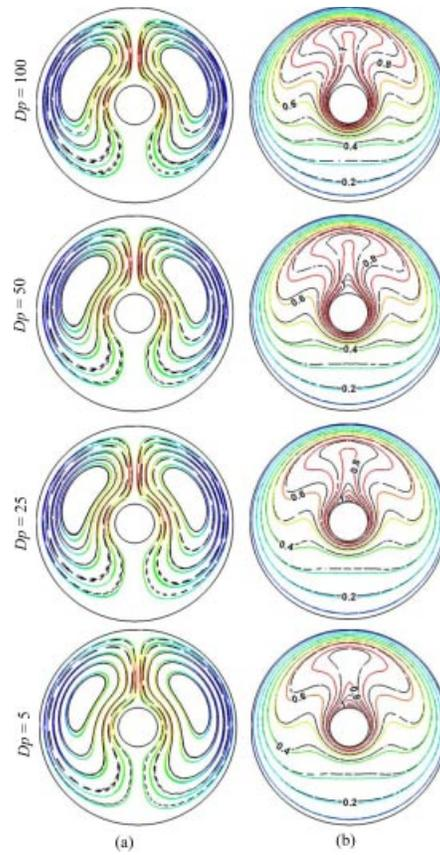
Fig. 6. Effect of  $Dp$  on (a) streamlines and (b) isotherms with  $Q = 1$ ,  $D = 0.2$  (colored lines for Pak and Cho model and black lines for Brinkman model). [Color figure can be viewed in the online issue, which is available at [wileyonlinelibrary.com/journal/htj](http://wileyonlinelibrary.com/journal/htj).]
