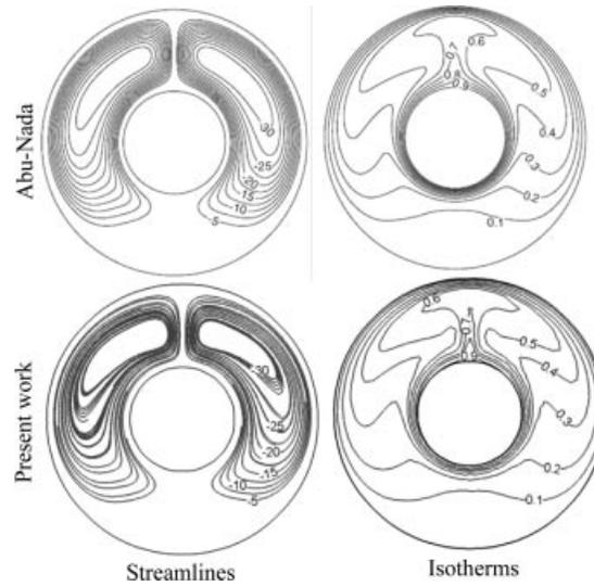
Fig. 4. Comparison between present work and Abu-Nada [21] for  $Ra = 10^5$ ,  $L/D = 0.8$ ,  $\phi = 4\%$ , and  $Pr = 0.7$ .
