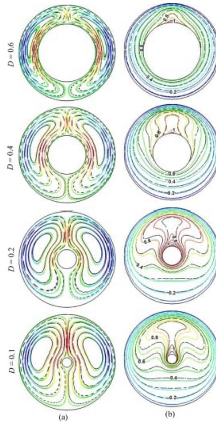
Fig. 7. Effect of  $D$  on (a) streamlines and (b) isotherms with  $Q = 1$ ,  $Dp = 5$  (colored lines for Pak and Cho model and black lines for Brinkman model). [Color figure can be viewed in the online issue, which is available at [wileyonlinelibrary.com/journal/htj](http://wileyonlinelibrary.com/journal/htj).]
