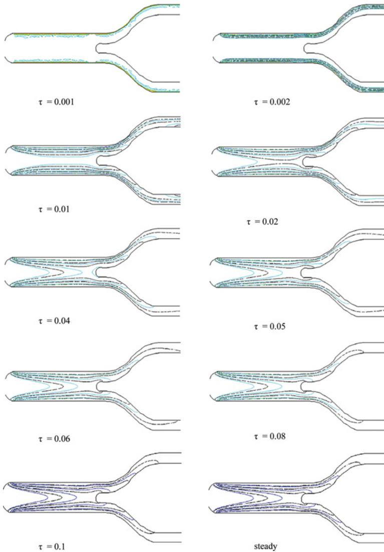
**Figure 4.** Transient behavior of isotherms at  $Re = 100$  and  $Pr = 6.62$ . (Solid lines for nanofluid and dashed lines for base fluid.) (color figure available online).
