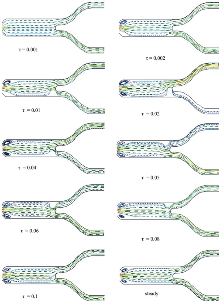
**Figure 3.** Transient behavior of streamlines at  $Re=100$  and  $Pr=6.62$ . (Solid lines for nanofluid and dashed lines for base fluid.) (color figure available online).
