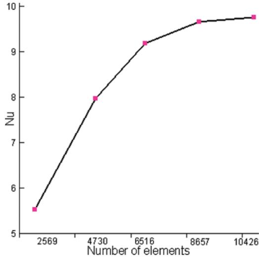
**Figure 2.** Grid independency study for  $Pr = 6.62$ ,  $Re = 100$ , and  $\phi = 5\%$  (color figure available online).
