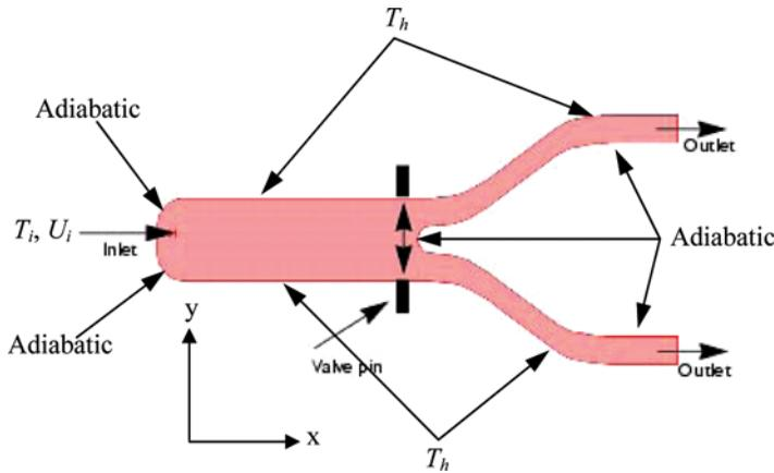
**Figure 1.** Depiction of the geometry and the operation of the fluid valve (color figure available online).
