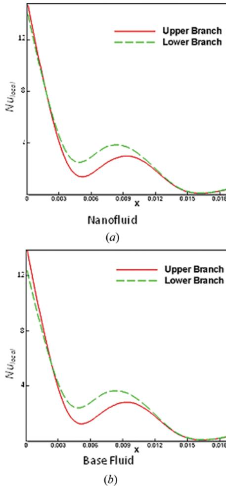
**Figure 7.** Plots of (a)  $Nu_{local}$  for nanofluid, and (b)  $Nu_{local}$  for base fluid (color figure available online).
