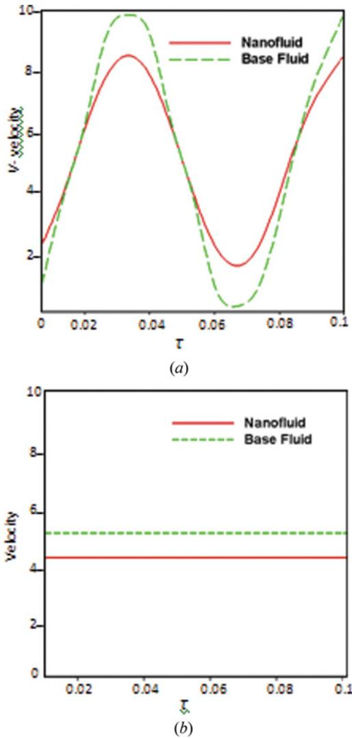
**Figure 6.** Plots of (a)  $V$ -velocity at the point (0.006, 0) in the valve, and (b) velocity as a function of time (color figure available online).
