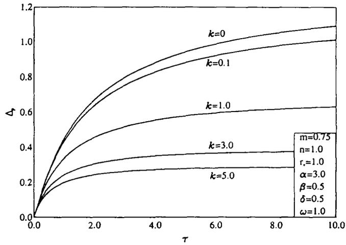
Figure 2. Effects of  $k$  on the Particle-Phase Displacement Thickness
