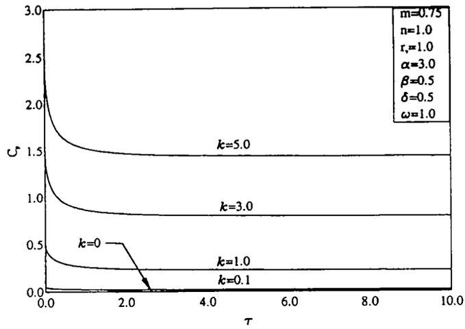
Figure 4. Effects of  $k$  on the Particle-Phase Skin-Friction Coefficient
