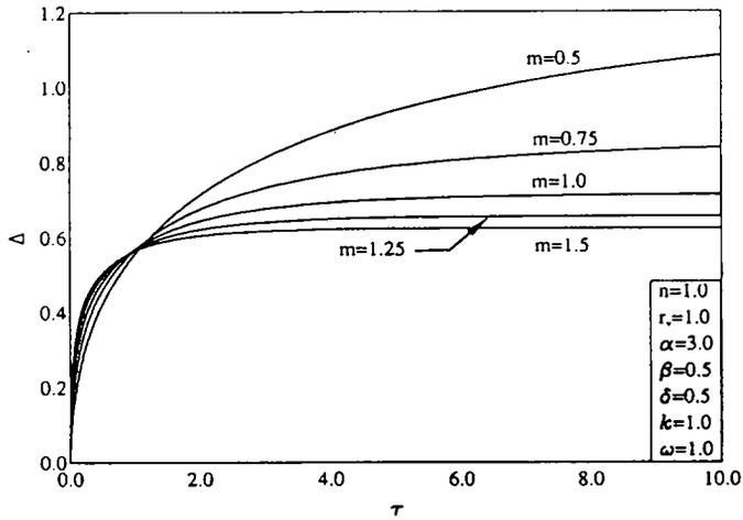
Figure 5. Effects of  $m$  on the Fluid-Phase Displacement Thickness
