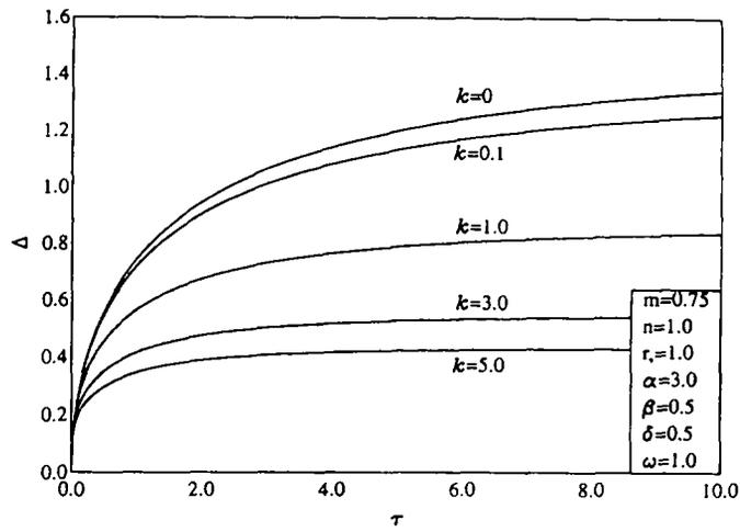
Figure 1. Effects of  $k$  on the Fluid-Phase Displacement Thickness
