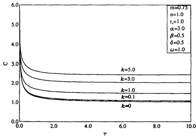
Figure 3. Effects of  $k$  on the Fluid-Phase Skin-Friction Coefficient
