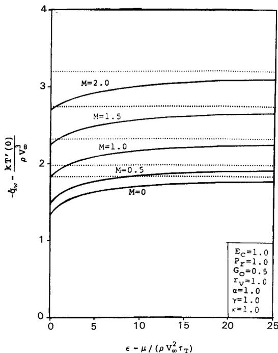
Fig. 2 Wall heat transfer vs  $\epsilon$ .
