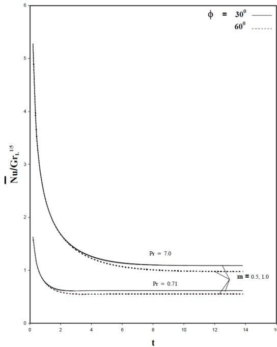
**Fig. 16.** Average Nusselt number for different values of  $m$ ,  $\phi$  and  $Pr$  in transient state
