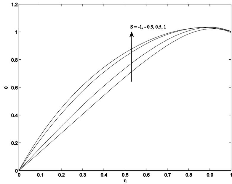
Figure 5: Temperature profiles for different  $S$  when  $K^2 = 2$ ,  $Pr = 0.71$  and  $Br = 0.5$
