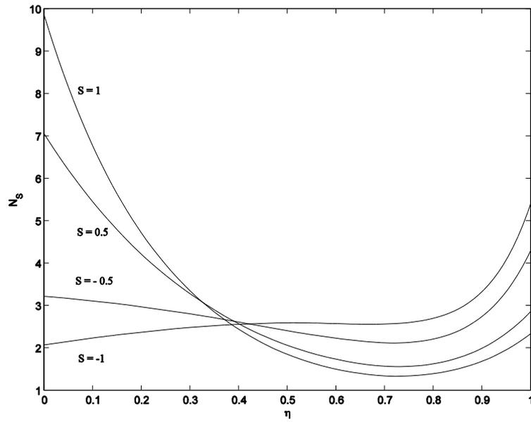
Figure 8:  $N_s$  for different  $S$  when  $K^2 = 2$ ,  $Pr = 0.71$ ,  $Br\Omega^{-1} = 1$  and  $Br = 0.5$
