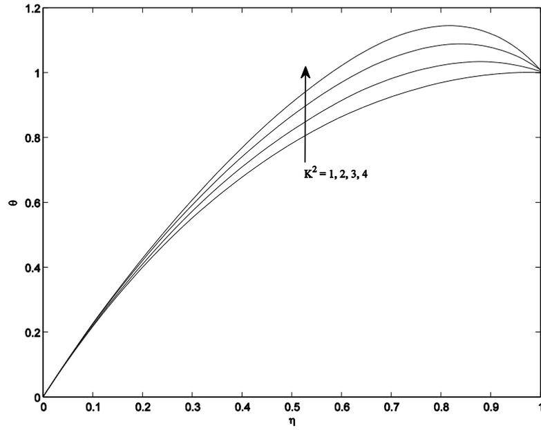
Figure 4: Temperature profiles for different  $K^2$  when  $S = 0.5$ ,  $Pr = 0.71$  and  $Br = 0.5$
