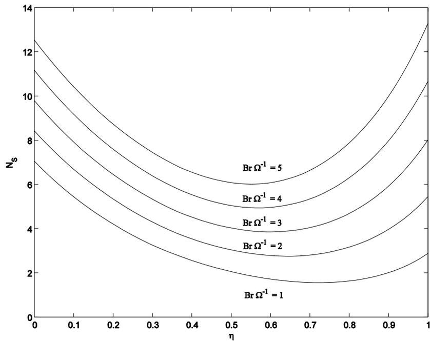
Figure 12:  $N_s$  for different  $Br\Omega^{-1}$  when  $K^2 = 2$ ,  $Pr = 0.71$ ,  $S = 0.5$  and  $Br = 0.5$
