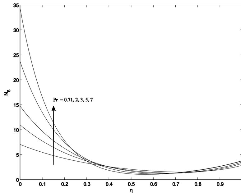
Figure 11:  $N_S$  for different  $Pr$  when  $K^2 = 2$ ,  $S = 0.5$ ,  $Br\Omega^{-1} = 1$  and  $Br = 0.5$
