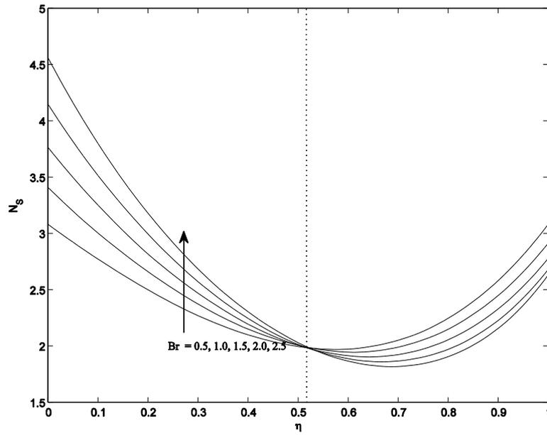
Figure 10:  $N_S$  for different  $Br$  when  $K^2 = 2$ ,  $Pr = 0.71$ ,  $Br\Omega^{-1} = 1$  and  $S = 0.5$
