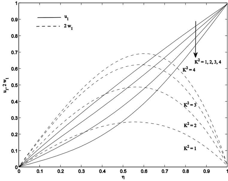
Figure 2: Velocity profiles for different  $K^2$  when  $S = 0.5$
