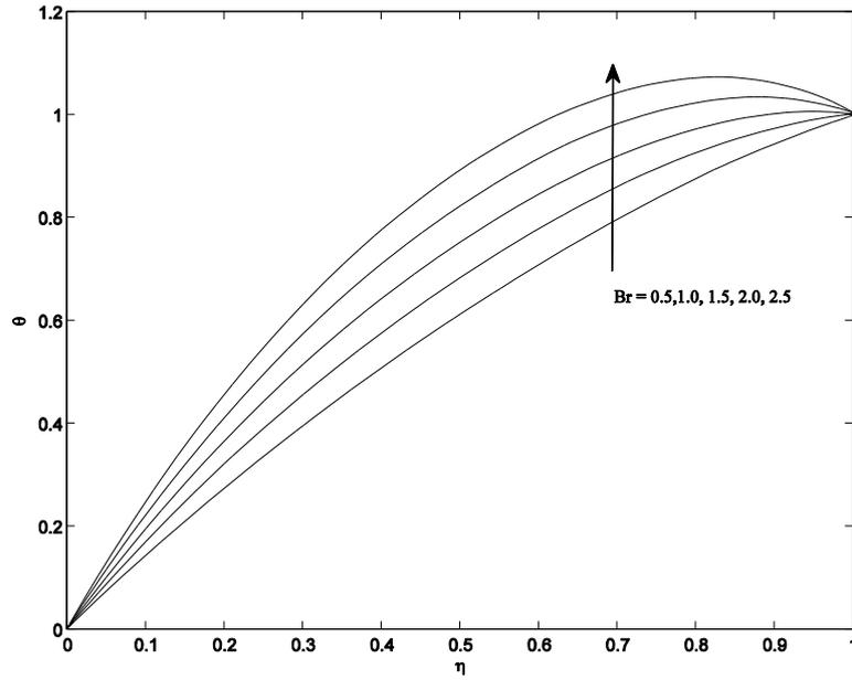
Figure 6: Temperature profiles for different Br when  $K^2 = 2$ ,  $Pr = 0.71$  and  $S = 0.5$
