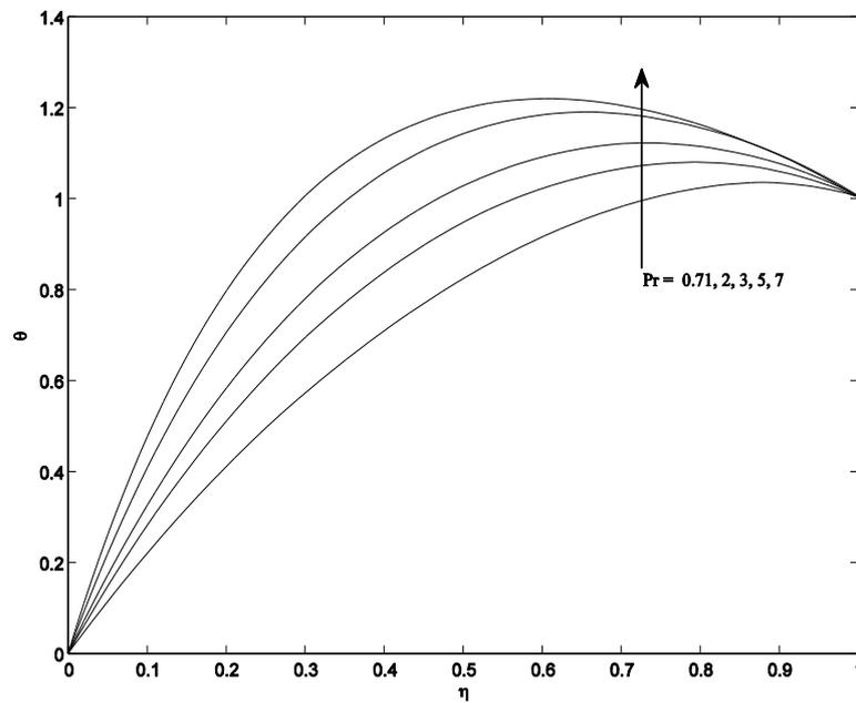
Figure 7: Temperature profiles for different Pr when  $K^2 = 2$ ,  $S = 0.5$  and  $Br = 0.5$
