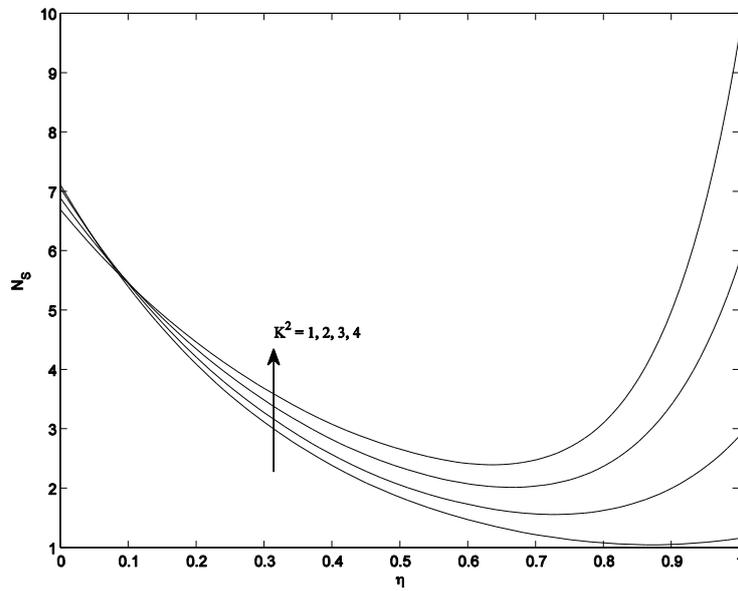
Figure 9:  $N_s$  for different  $K^2$  when  $S = 0.5$ ,  $Pr = 0.71$ ,  $Br\Omega^{-1} = 1$  and  $Br = 0.5$
