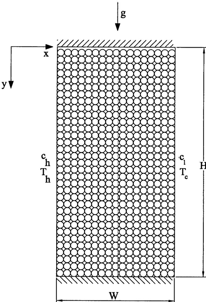
Figure 1. Schematic diagram of the porous enclosure.
