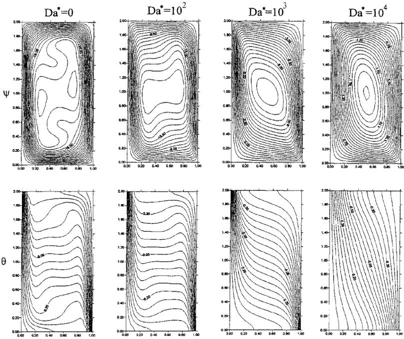
**Figure 3.** Effects of  $Da^*$  on the contours of the streamlines, temperature, and concentration for  $Le = 1.0$ ,  $N = 1.0$ ,  $Pr = 0.7$ ,  $Ra = 10^5$ , and  $\phi = 0$ .
