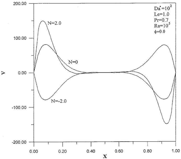
Figure 13. Effects of  $N$  on vertical velocity profiles at enclosure midsection.
