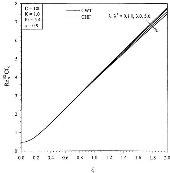
Fig. 4. Effect of  $\lambda$  or  $\lambda^*$  on  $Re_x^{1/2}Cf_x$  for CWT and CHF cases.
