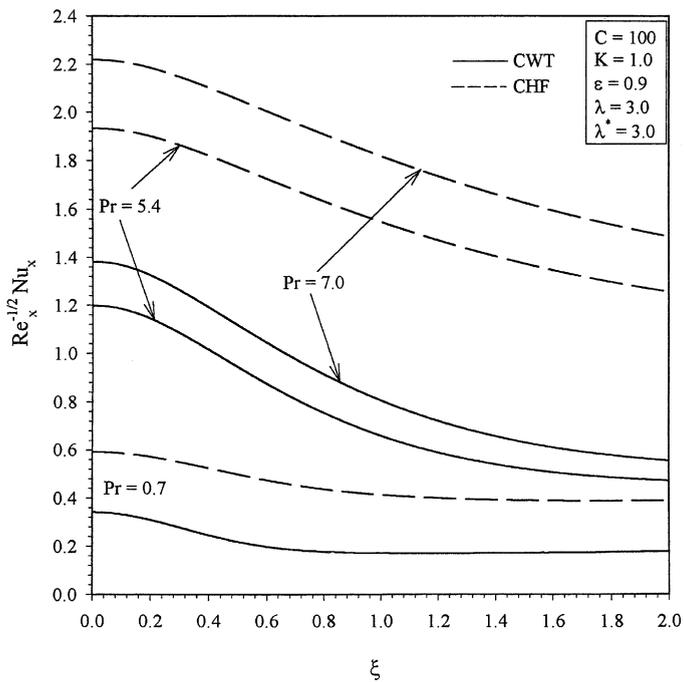
Fig. 14. Effect of  $Pr$  on  $Re_x^{-1/2} Nu_x$  for CWT and CHF cases.
