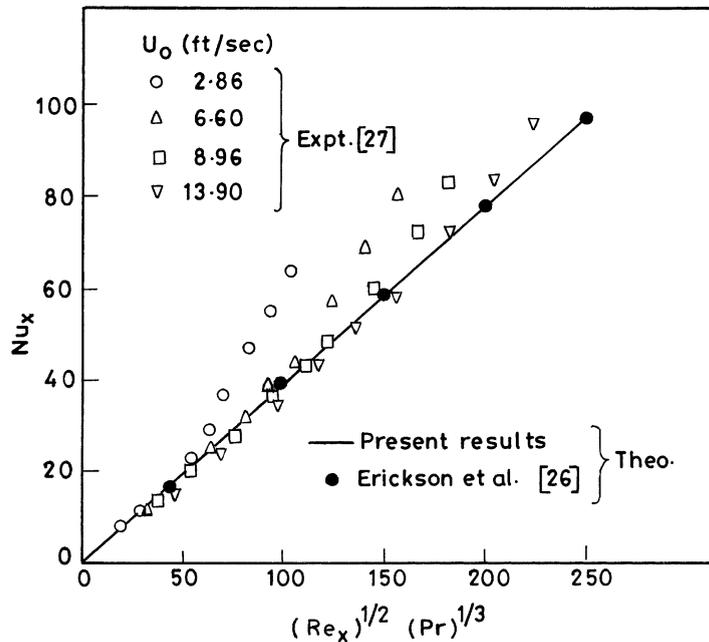
Fig. 3. Comparison of the Nusselt number  $Nu_x$  for the CWT case when  $\xi = \lambda = K^{-1} = C = 0$ ,  $\varepsilon = 1$  with that of Erickson et al. [26] and Griffin and Thorne [27].
