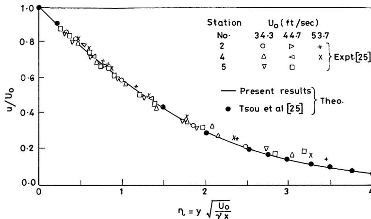
Fig. 2. Comparison of the velocity profile  $u/U_0$  for  $\xi = \lambda = K^{-1} = C = 0$ ,  $\varepsilon = 1$  with that of Tsou et al. [25].
