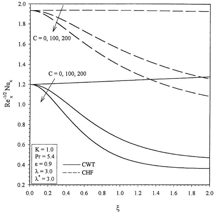
Fig. 13. Effect of  $C$  on  $Re_x^{-1/2} Nu_x$  for CWT and CHF cases.
