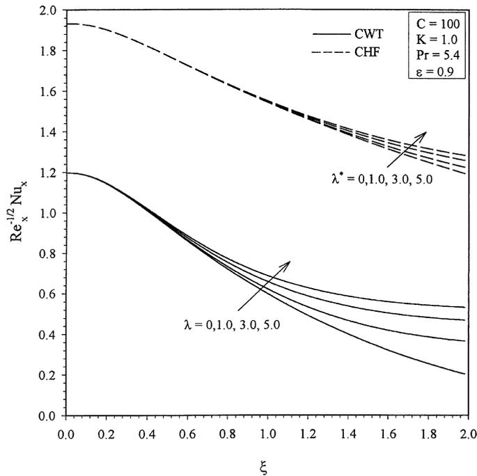
Fig. 5. Effect of  $\lambda$  or  $\lambda^*$  on  $Re_x^{-1/2}Nu_x$  for CWT and CHF cases.
