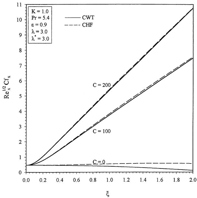
Fig. 12. Effect of  $C$  on  $Re_x^{1/2} Cf_x$  for CWT and CHF cases.
