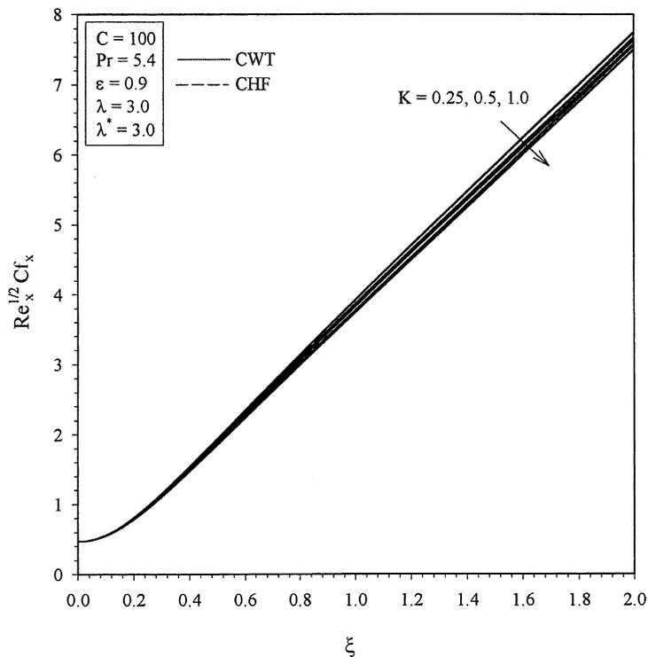
Fig. 10. Effect of  $K$  on  $Re_x^{1/2}Cf_x$  for CWT and CHF cases.
