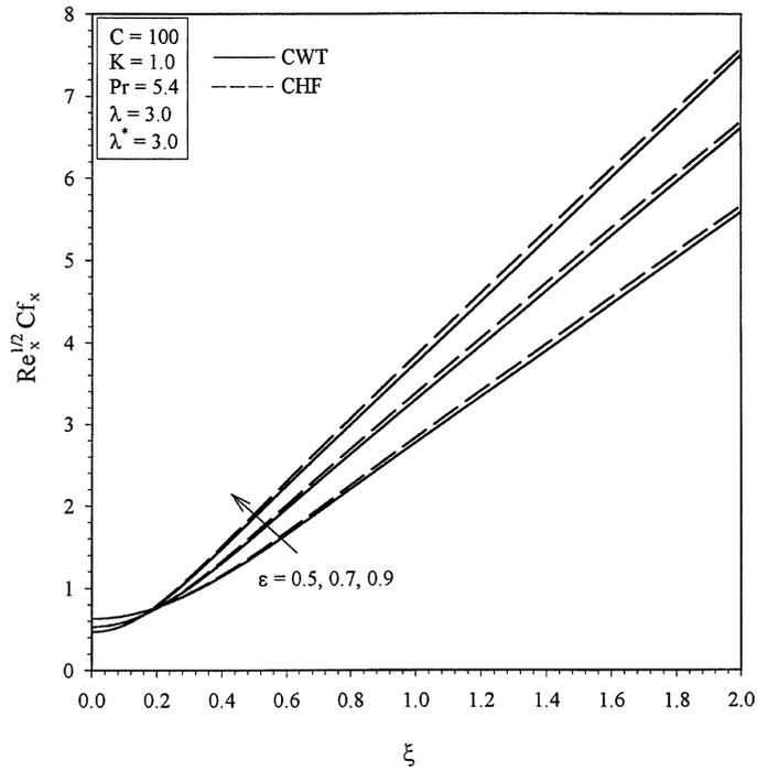
Fig. 8. Effect of  $\varepsilon$  on  $Re_x^{1/2} Cf_x$  for CWT and CHF cases.
