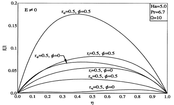
Fig. 12. Flow fields for electrically-insulating walls
