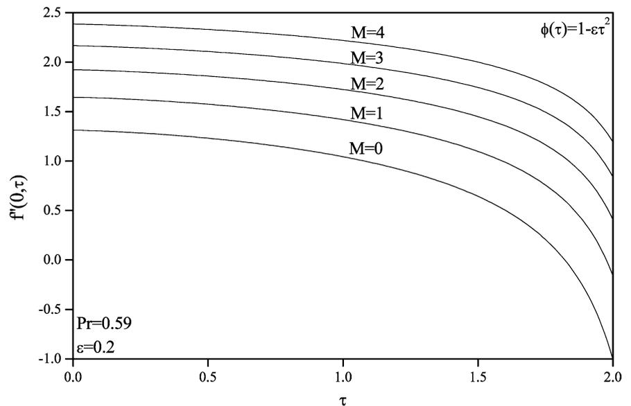
**Fig. 11** Effect of magnetic parameter  $M$  on the surface shear stress in the secondary flow,  $s'(0, \tau)$ , for decelerating flow
