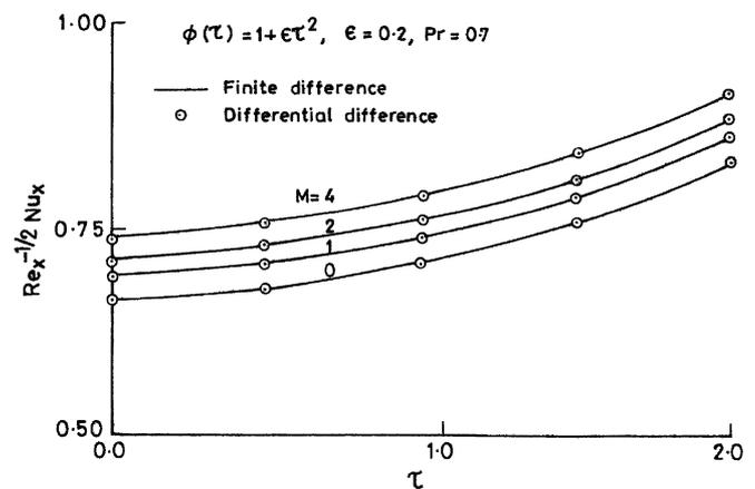
Fig. 2 Comparison of the Nusselt number  $Re_x^{-1/2} Nu_x$ , for the CWT case, obtained by finite-difference and differential-difference methods
