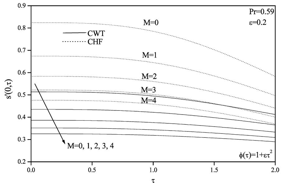
**Fig. 9** Effect of magnetic parameter  $M$  on the Nusselt number,  $Re_x^{-1/2} Nu_x$ , for accelerating flow
