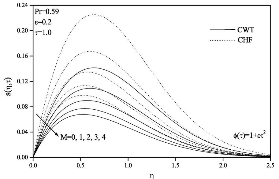
**Fig. 5** Effect of magnetic parameter  $M$  on the temperature profiles,  $\theta(\eta, \tau)$
