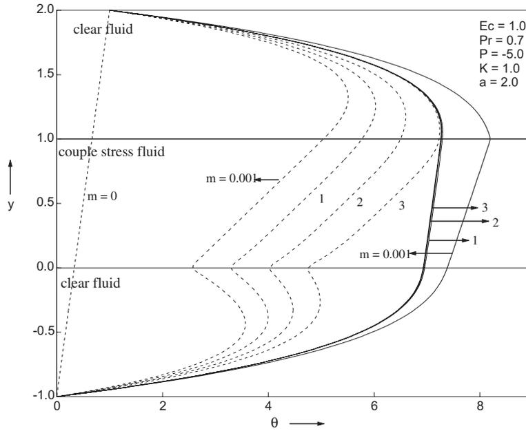
**Fig. 6.** Temperature profiles for different values of the ratio of the thermal conductivity  $K$ .
