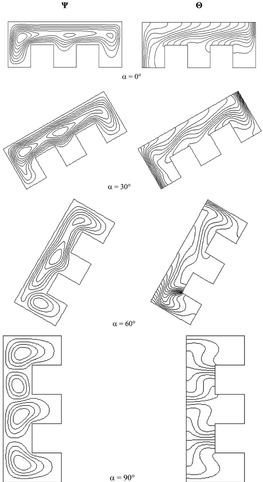
increase and the secondary vortices within the partitioned enclosure starts to separate. For example, when  $\alpha=60^\circ$ , a separated cell is predicted close to the heated
