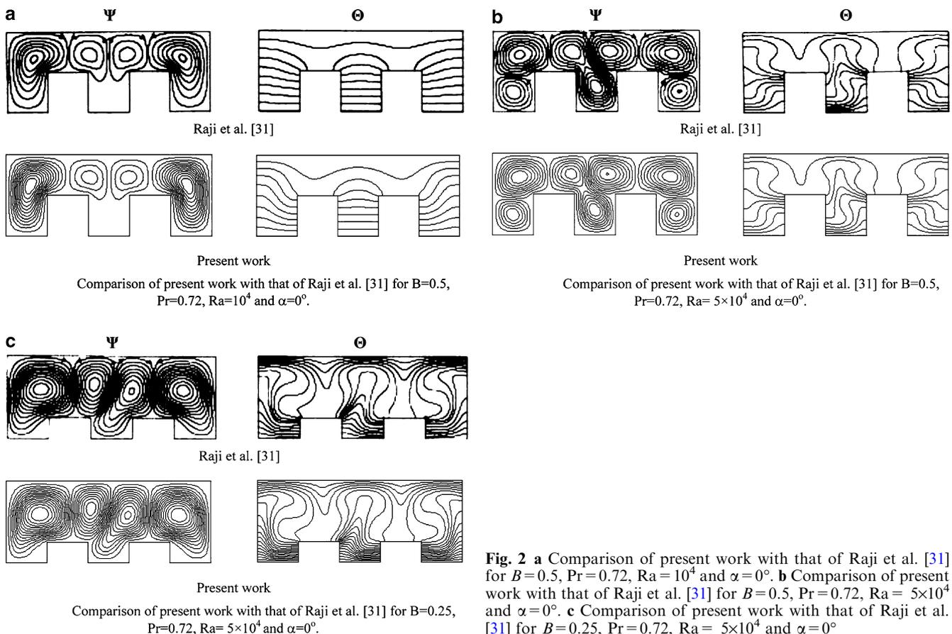
**Fig. 2** **a** Comparison of present work with that of Raji et al. [31] for  $B=0.5$ ,  $Pr=0.72$ ,  $Ra=10^4$  and  $\alpha=0^\circ$ . **b** Comparison of present work with that of Raji et al. [31] for  $B=0.5$ ,  $Pr=0.72$ ,  $Ra=5 \times 10^4$  and  $\alpha=0^\circ$ . **c** Comparison of present work with that of Raji et al. [31] for  $B=0.25$ ,  $Pr=0.72$ ,  $Ra=5 \times 10^4$  and  $\alpha=0^\circ$
