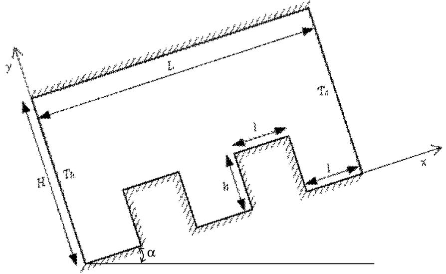
walls are assumed to be adiabatic. Figure 1 shows the schematic and coordinate system of the problem under consideration. The fluid is assumed to be incompressible, Newtonian and viscous has constant thermo-physical properties except the density in the buoyancy term of the momentum equations. The effect due to viscous dissipation is assumed to be negligible.
