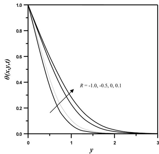
**Figure 3** Steady state dimensionless fluid concentration profiles at the midpoint of the plate as a function of transverse direction  $y$  ( $Pr = 11$ ,  $Sc = 800$ ,  $q = 1.8$ ,  $Gr^* = 1$ )
