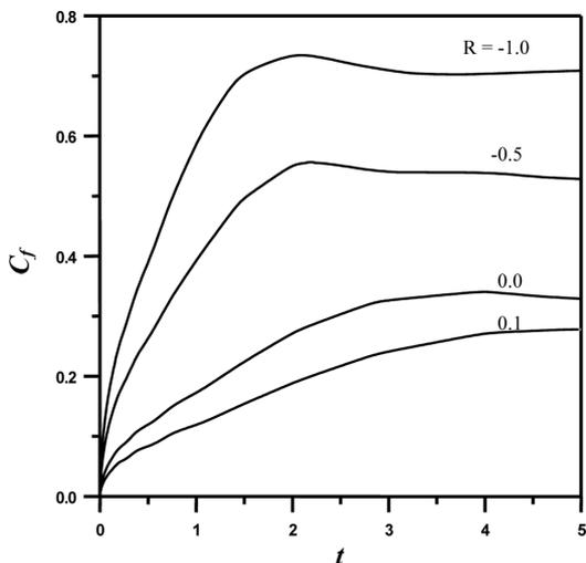
**Figure 7** Skin-friction coefficient variations at the midpoint of the plate as a function of the dimensionless time  $t$  ( $Pr = 11$ ,  $Sc = 800$ ,  $q = 1.8$ ,  $R = 0.1$ )
