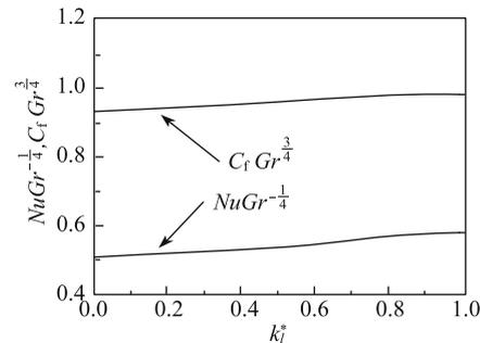
**Fig. 5** Steady state local coefficients of friction  $C_f Gr^{3/4}$  and local Nusselt number  $NuGr^{-1/4}$  via  $k_i^*$  for  $Pr=7$  at  $x=0.5$  (midpoint)
