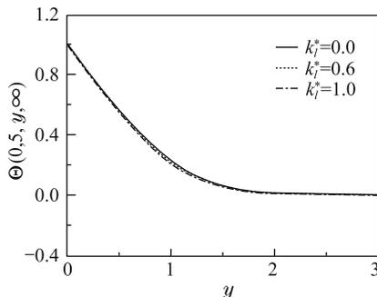
**Fig. 3** Steady state temperature profiles for  $Pr=7$  at  $x=0.5$  (midpoint)
