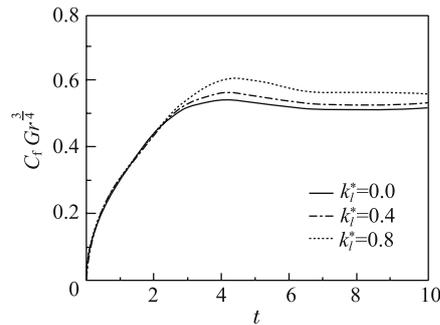
**Fig. 4** Transient friction coefficient  $C_f Gr^{\frac{3}{4}}$  for  $Pr=7$  at  $x=0.5$  (midpoint)
