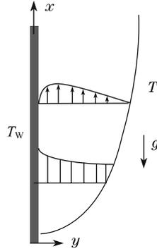
**Fig. 1** Transient free convection model for a viscoelastic fluid near a vertical wall
