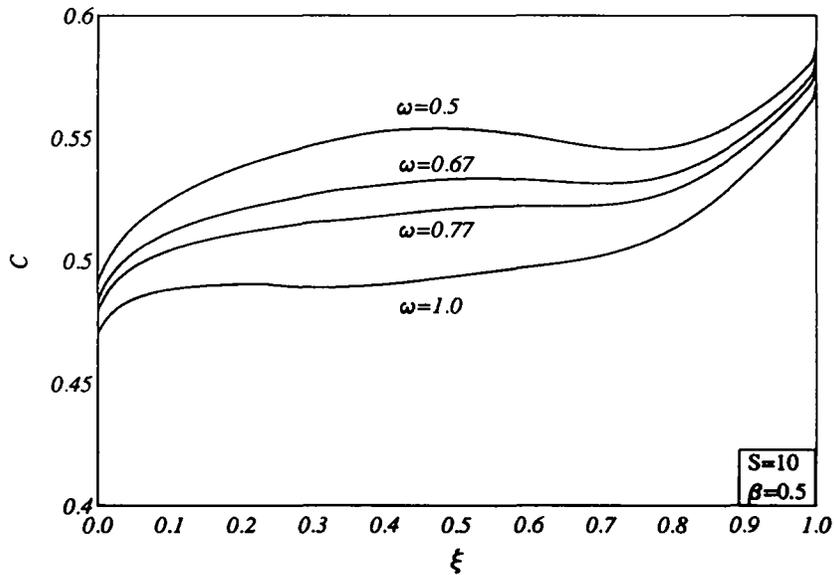
Fig. 16. Fluid-phase skin friction coefficient profiles.
