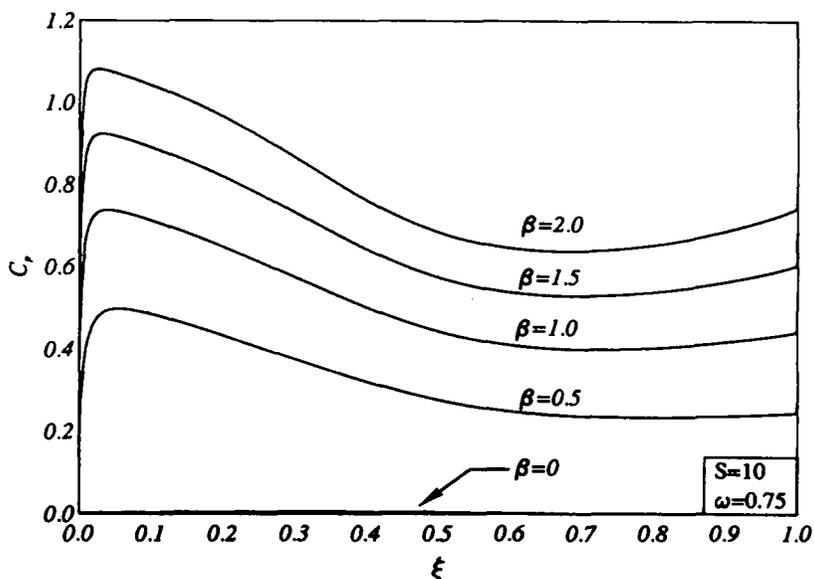
Fig. 12. Particle-phase skin friction coefficient profiles.
