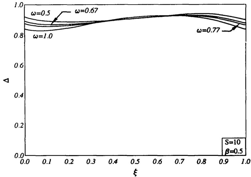
Fig. 14. Fluid-phase displacement thickness profiles.
