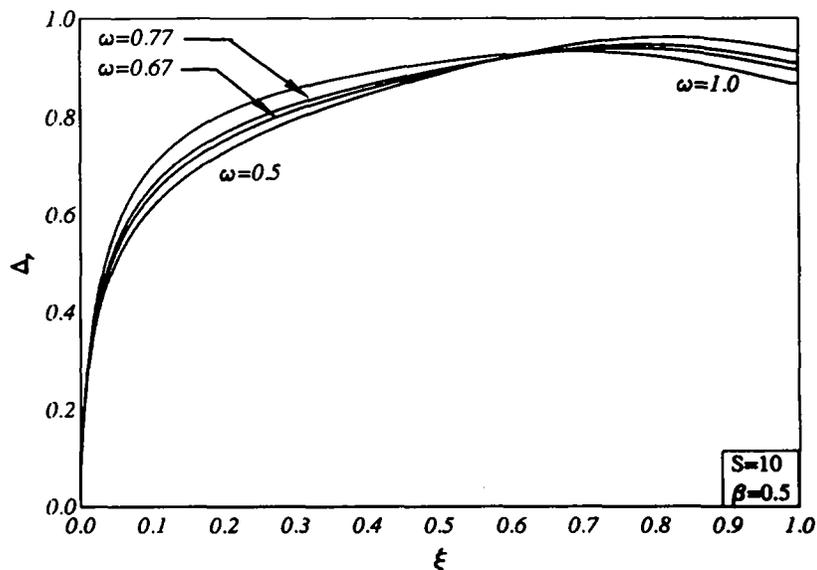
Fig. 15. Particle-phase displacement thickness profiles.
