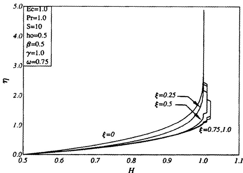
Fig. 7. Fluid-phase temperature profiles.
