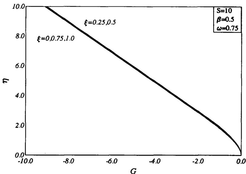
Fig. 4. Fluid-phase normal velocity profiles.
