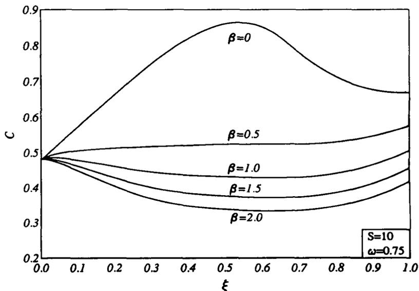
Fig. 11. Fluid-phase skin friction coefficient profiles.
