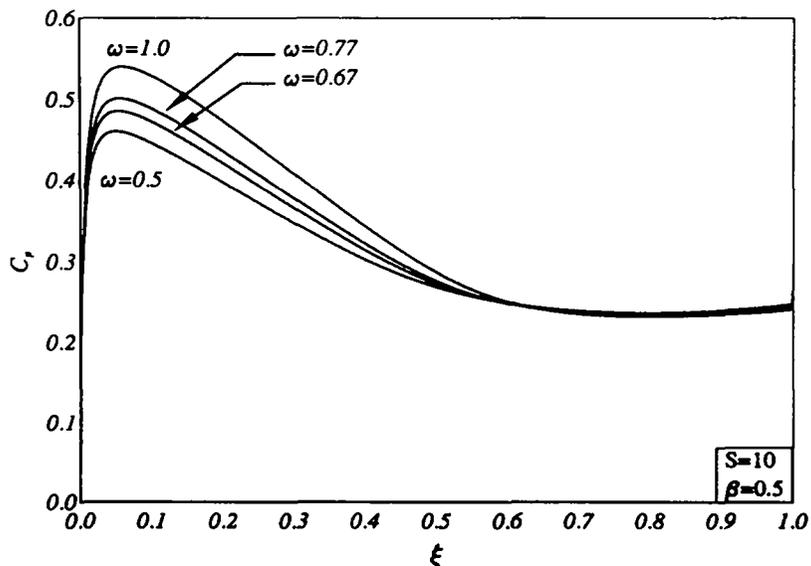
Fig. 17. Particle-phase skin friction coefficient profiles.
