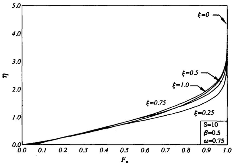
Fig. 3. Particle-phase tangential velocity profiles.
