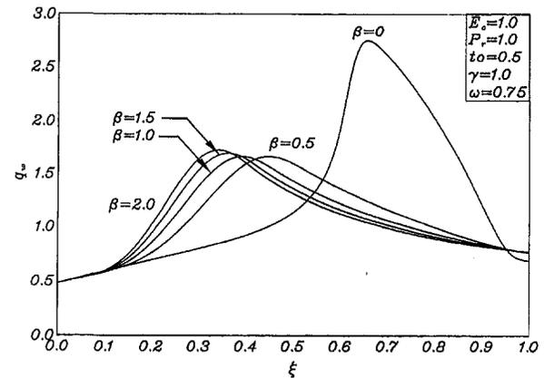
Fig. 10 Wall heat transfer coefficient profiles
