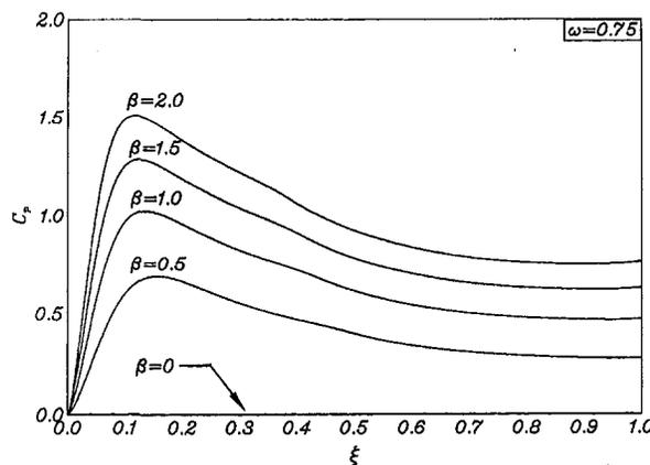
Fig. 7 Particle-phase skin friction coefficient profiles
