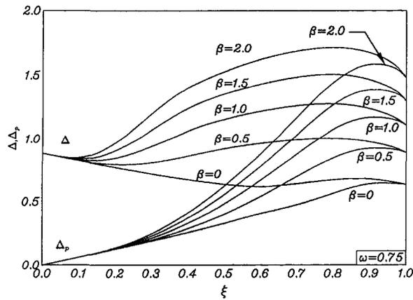
Fig. 5 Fluid and particle-phase displacement thicknesses profiles
