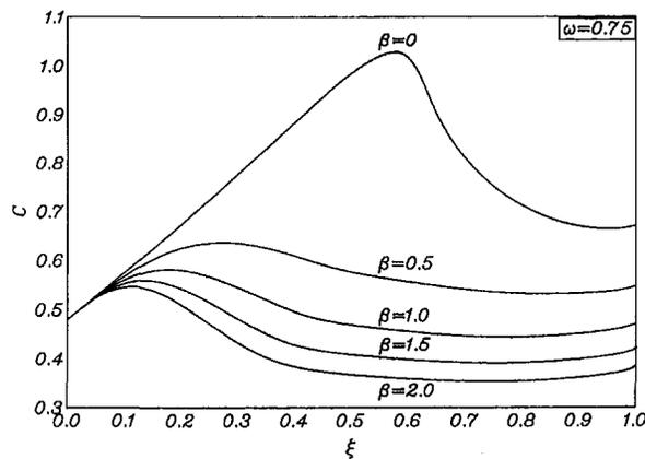
Fig. 6 Fluid-phase skin friction coefficient profiles
