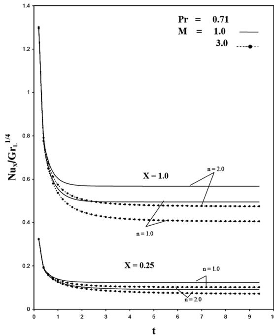
Figure 7. Local Nusselt number at  $X = 0.25$  and  $1.0$  for various values of  $n$  and  $M$  in transient period.
