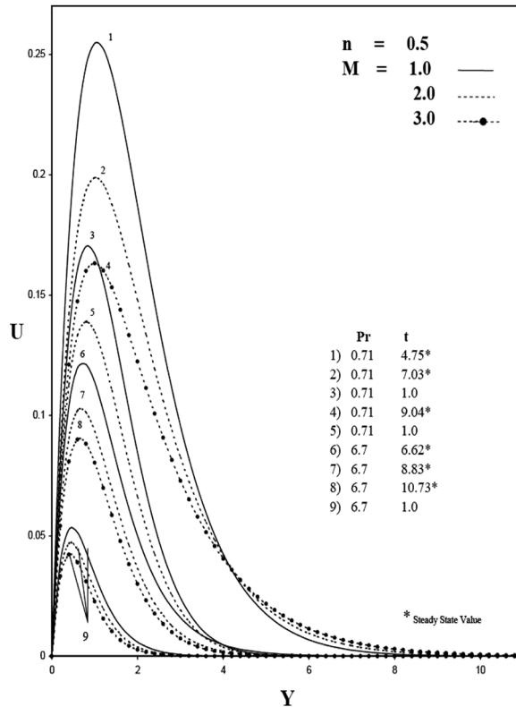
**Figure 2.** Transient velocity profiles at  $X = 1.0$  for various values of Pr and  $M$ .
