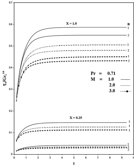
Figure 6. Local skin friction at  $X = 0.25$  and  $1.0$  for various values of  $n$  and  $M$  in transient period.
