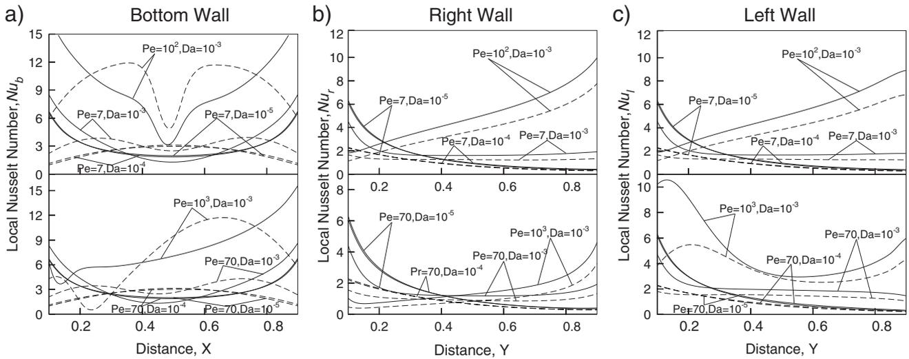
**Fig. 5.** Variation of Local Nusselt Number with the distance at the (a) bottom wall (b) right wall and (c) left wall for uniform heating (—) and non-uniform heating (...) of bottom wall for  $Gr = 10^5$ . In each plot, upper panel corresponds to  $Re = 10$  and lower panel represents  $Re = 10^2$ .
