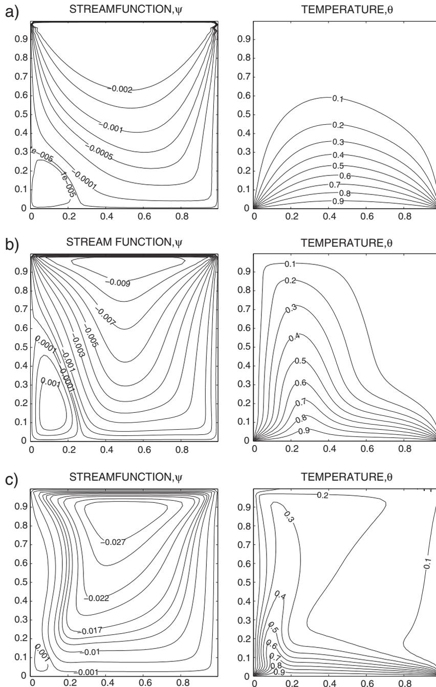
Fig. 2. Streamfunction and temperature contours for uniform heating of bottom wall with  $Pr = 10$ ,  $Re = 100$ ,  $Pe = 10^3$ ,  $Gr = 10^5$ : (a)  $Da = 10^{-5}$  (b)  $Da = 10^{-4}$  and (c)  $Da = 10^{-3}$ .
