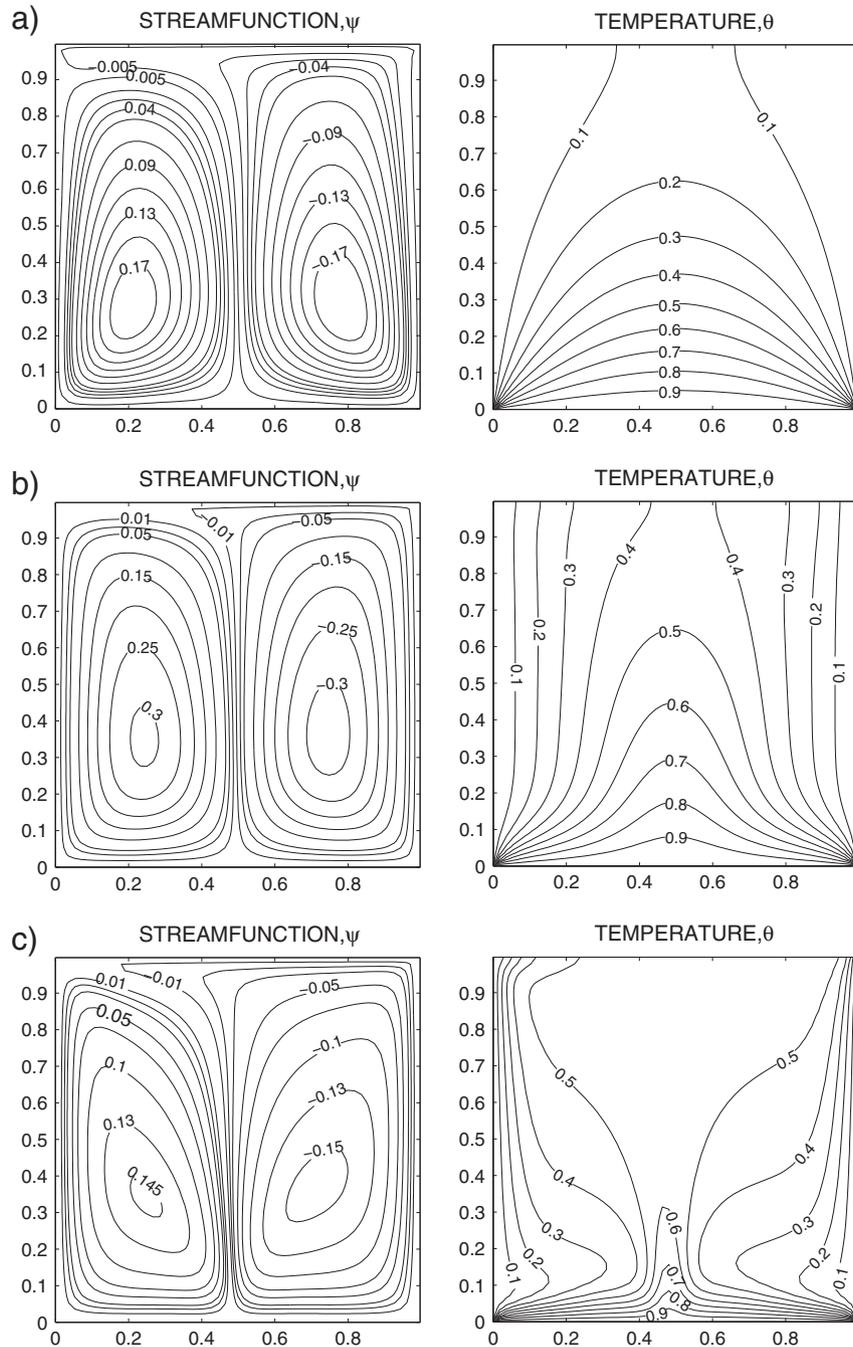
**Fig. 3.** Streamfunction and temperature contours for uniform heating bottom wall with  $Re = 10$ ,  $Gr = 10^5$ ,  $Da = 10^{-3}$ : (a)  $Pr = 0.026$  ( $Pe = 0.26$ ) (b)  $Pr = 0.7$  ( $Pe = 7$ ) and (c)  $Pr = 10$  ( $Pe = 10^2$ ).
