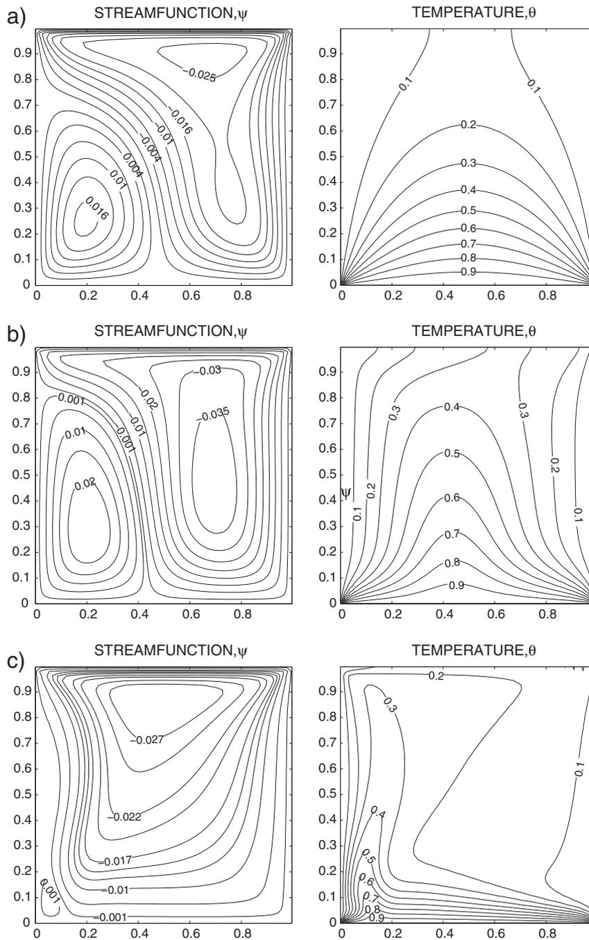
**Fig. 4.** Streamfunction and temperature contours for uniform heating of bottom wall with  $Re=100$ ,  $Gr=10^5$ ,  $Da=10^{-3}$ : (a)  $Pr=0.026$  ( $Pe=2.6$ ) (b)  $Pr=0.7$  ( $Pe=70$ ) and (c)  $Pr=10$  ( $Pe=10^3$ ).
