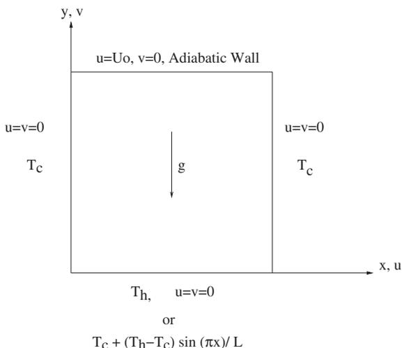
Fig. 1. Schematic diagram of the physical system.
