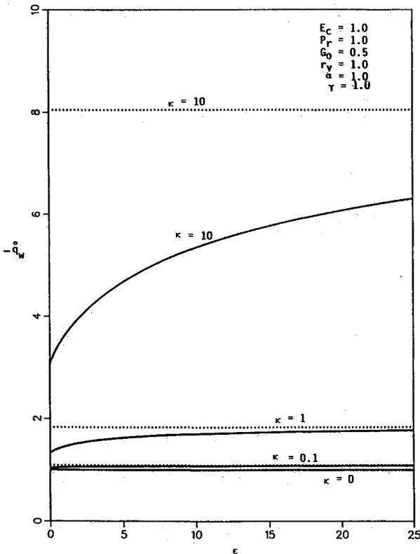
Fig. 3 Wall heat transfer coefficient vs  $\epsilon$ .
