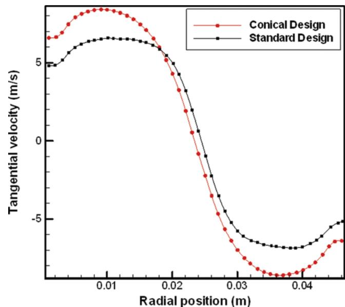
FIG. 12. Radial tangential velocity profile for two entrance chamber design at 150 mm from the top wall of standard and conical hydrocyclone ( $\alpha_{in} = 0.5\%$ ,  $d_{d_{sd},50,in} = 200 \mu\text{m}$ ,  $V_{in} = 3.2 \text{ m/s}$ ). (Color figure available online)
