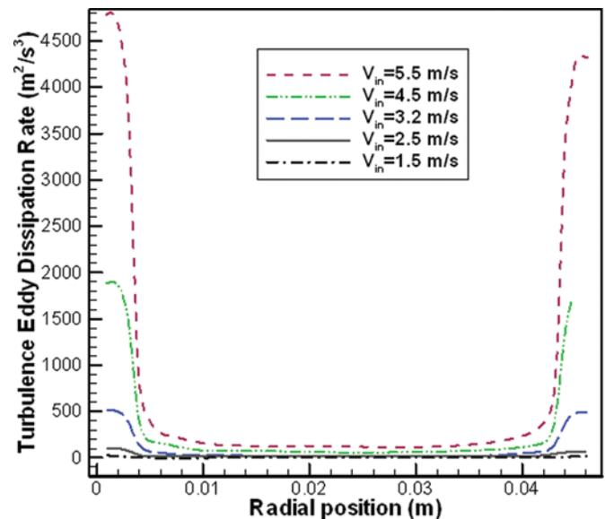
FIG. 9. Radial distribution of turbulence eddy dissipation rate in different inlet velocities at 150 mm from the top wall of standard hydrocyclone ( $\alpha_{in} = 0.5\%$ ,  $d_{d_{sd},50,in} = 150 \mu\text{m}$ ). (Color figure available online)
