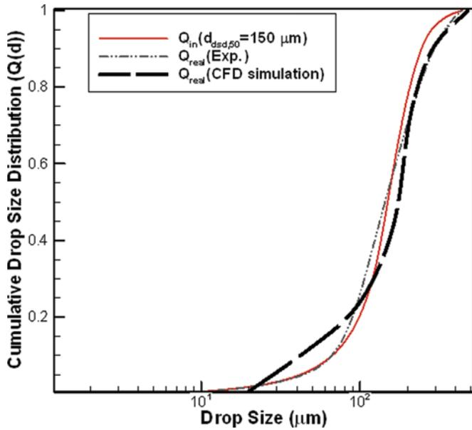
FIG. 4. Comparison the real droplet size distribution obtaining with CFD and experimental work [15],  $d_{d_{sd},50,in} = 150 \mu\text{m}$ ,  $\alpha_{in} = 0.5\%$ ,  $V_{in} = 3.2 \text{ m/s}$ . (Color figure available online)
