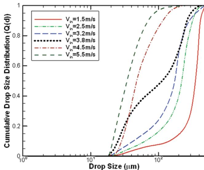
FIG. 10. Real cumulative size distribution for six different entrance velocities ( $\alpha_{in} = 0.5\%$ ,  $d_{d_{sd},50,in} = 150 \mu\text{m}$ ). (Color figure available online)
