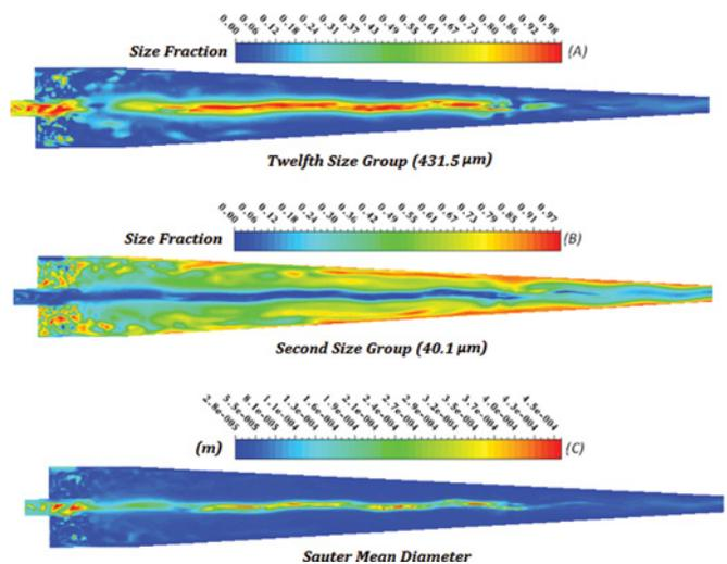
FIG. 6. Distribution of dispersed phase A) Twelfth size group, B) Second size group, and C) Droplets Sauter mean diameter ( $d_{d_{sd},50,in} = 150 \mu\text{m}$ ,  $\alpha_{in} = 0.5\%$ ,  $V_{in} = 3.2 \text{ m/s}$ ). (Color figure available online)
