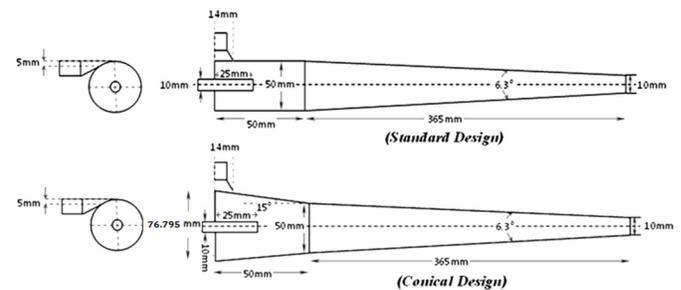
FIG. 2. Geometry details of two de-oiling hydrocyclones with different feed chamber.
