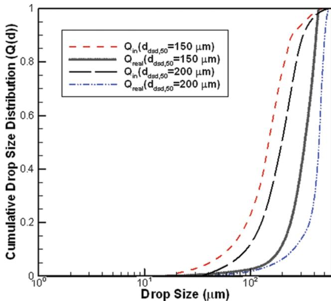
FIG. 7. Real cumulative size distribution for two different entrance size distributions in high volume fraction ( $\alpha_{in} = 15\%$  oil) versus the inlet droplet size distribution ( $V_{in} = 3.2 \text{ m/s}$ ). (Color figure available online)
