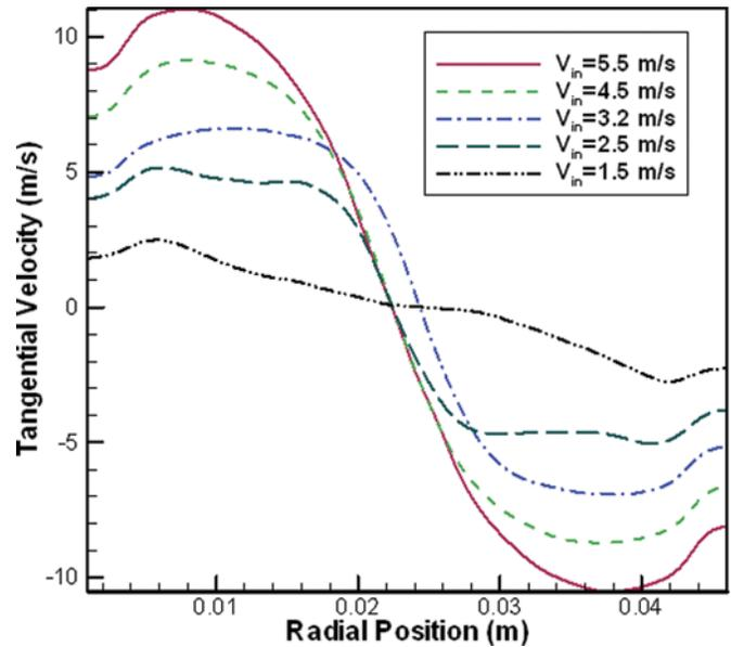
FIG. 8. Radial tangential velocity distribution in different inlet velocities at 150 mm from the top wall of standard hydrocyclone ( $\alpha_{in} = 0.5\%$ ,  $d_{d_{sd},50,in} = 150 \mu\text{m}$ ). (Color figure available online)
