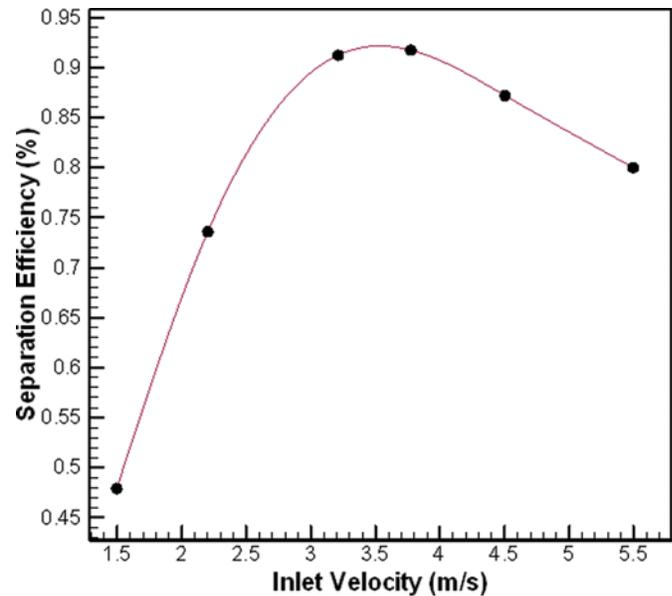
FIG. 11. Separation efficiency versus entrance velocity for standard design ( $\alpha_{in} = 0.5\%$ ,  $d_{d_{sd},50,in} = 150 \mu\text{m}$ ). (Color figure available online)
