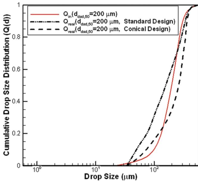
FIG. 13. Real cumulative size distribution for two different designs ( $\alpha_{in} = 0.5\%$ ,  $d_{dsd,50,in} = 200 \mu\text{m}$ ,  $V_{in} = 3.2 \text{ m/s}$ ). (Color figure available online)
