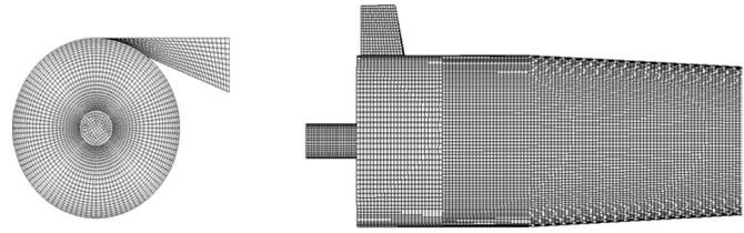
FIG. 3. Cross section of structured grid for hydrocyclone CFD simulation.
