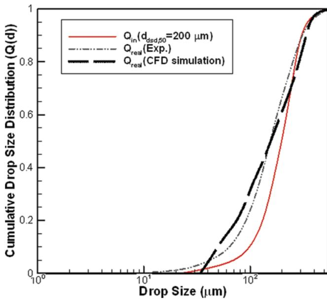
FIG. 5. Comparison the real droplet size distribution obtaining with CFD and experimental work [15],  $d_{d_{sd},50,in} = 200 \mu\text{m}$ ,  $\alpha_{in} = 0.5\%$ ,  $V_{in} = 3.2 \text{ m/s}$ . (Color figure available online)
