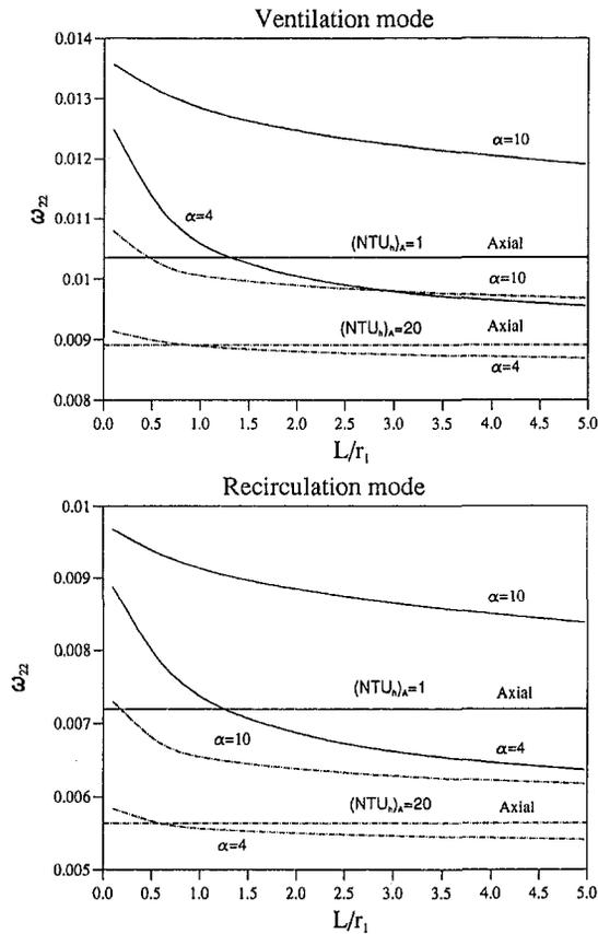
**Fig. 9 Comparison of performance of radial and axial exchangers for  $(NTU)_A = 1.0$  and  $20.0$  for various values of  $L/r_1$  and  $\alpha$  for both ventilation and recirculation modes**
