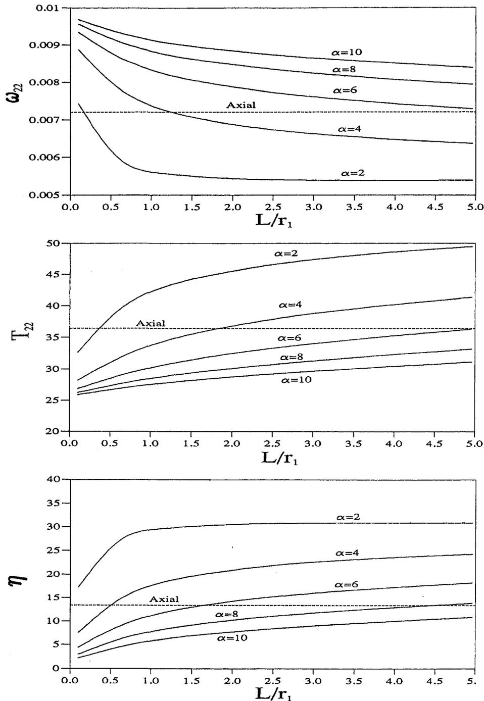
Fig. 8 Comparison of performance of radial exchanger with axial exchanger at recirculation mode for  $(NTU_h)_A = 1.0$  and various values of  $\alpha$  and  $L/r_1$
