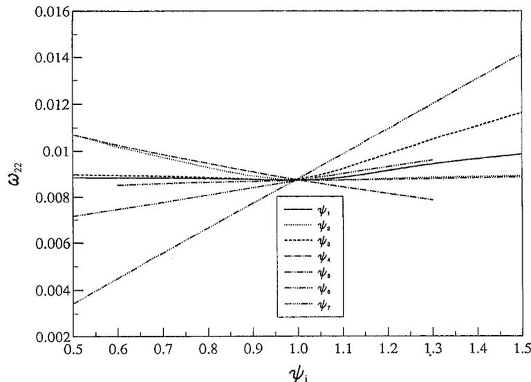
**Fig. 2 Dependence of  $\omega_{22}$  of an ideal radial exchanger on the inlet air condition and the operational parameters for flow configuration 2 at ventilation mode**
