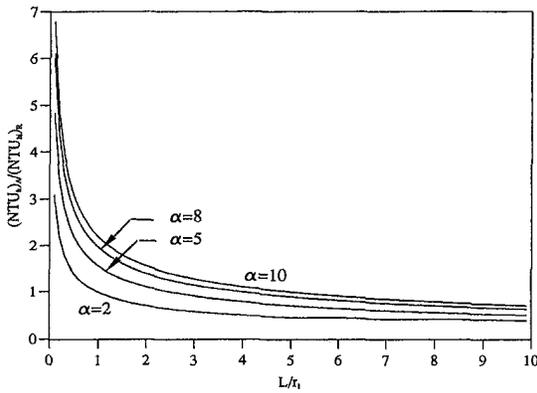
Fig. 6 Variation of the ratio of  $(NTU_h)_A / (NTU_h)_B$  with  $\alpha$  and  $L/r_1$
