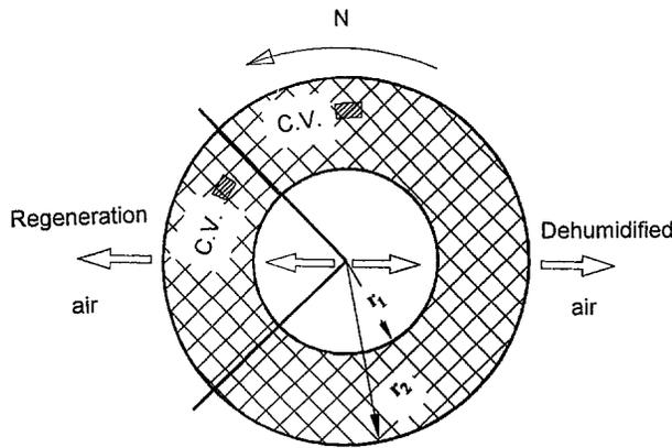
Fig. 1 Radial flow desiccant wheel
