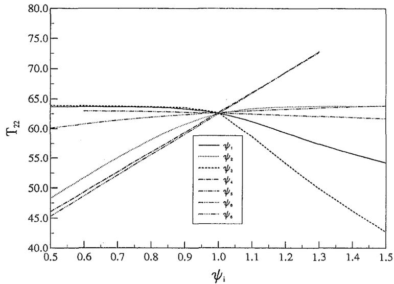
Fig. 3 Dependence of  $T_{22}$  of an ideal radial exchanger on the inlet air condition and the operational parameters for flow configuration 2 at ventilation mode
