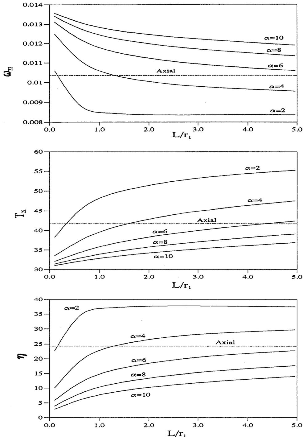
Fig. 7 Comparison of performance of radial exchanger at ventilation mode for  $(NTU_h)_A = 1.0$  and various values of  $\alpha$  and  $L/r_1$
