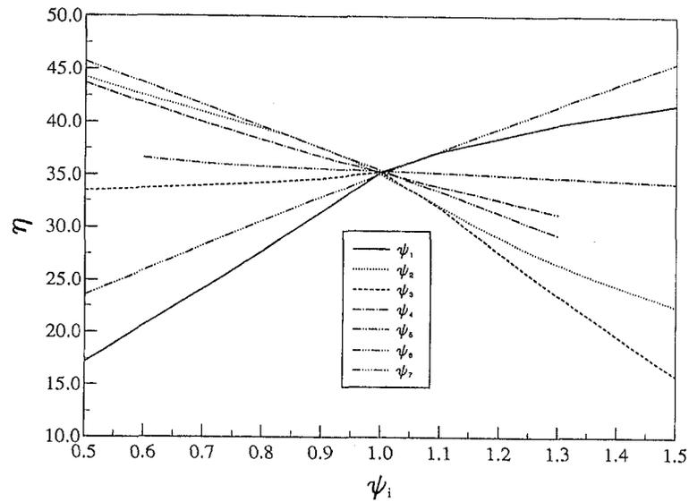
Fig. 4 Dependence of  $\eta_{22}$  of an ideal radial exchanger on the inlet air condition and the operational parameters for flow configuration 2 at ventilation mode
