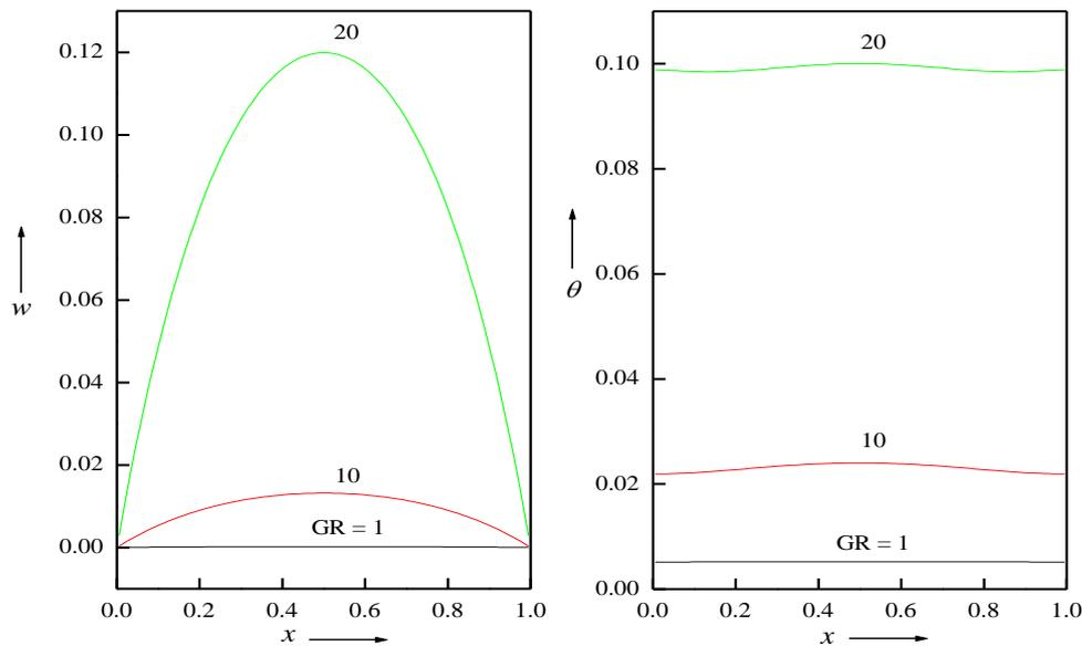
Figure 2b. Velocity and temperature profiles for different values of Grashof number  $GR$  for  $BR = 2$  and  $A = 1$ .
