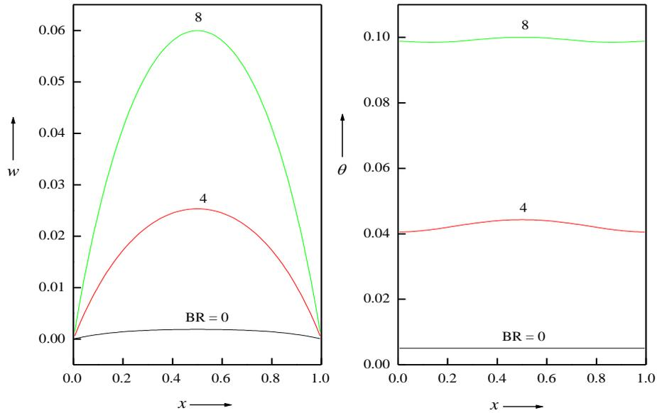
Figure 3b. Velocity and temperature profiles for different values of Brinkman number  $BR$  for  $GR = 10$  and  $A = 1$ .
