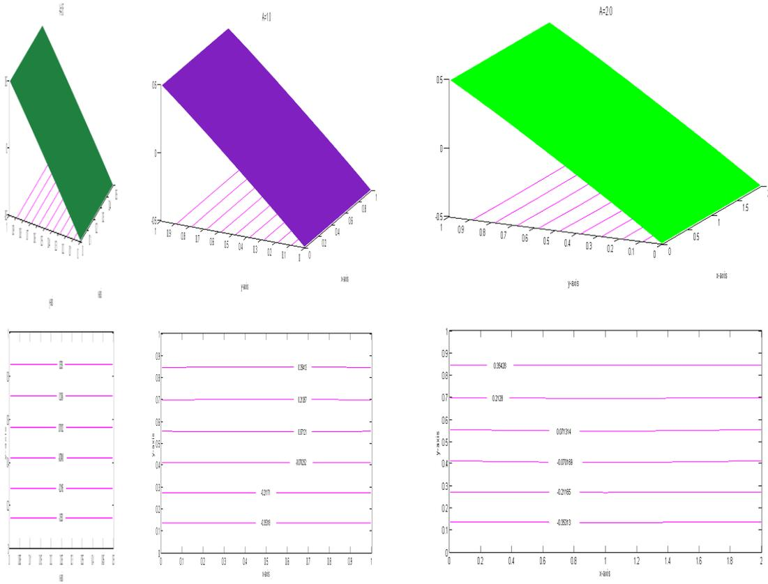
Figure 4a. Velocity and temperature contours for different values of Aspect ratio  $A$  for  $GR = 20$  and  $BR = 2$ .
