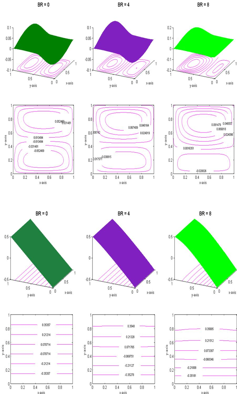
Figure 3a. Velocity and temperature contours for different values of Brinkman number  $BR$  for  $GR = 10$  and  $A = 1$ .
