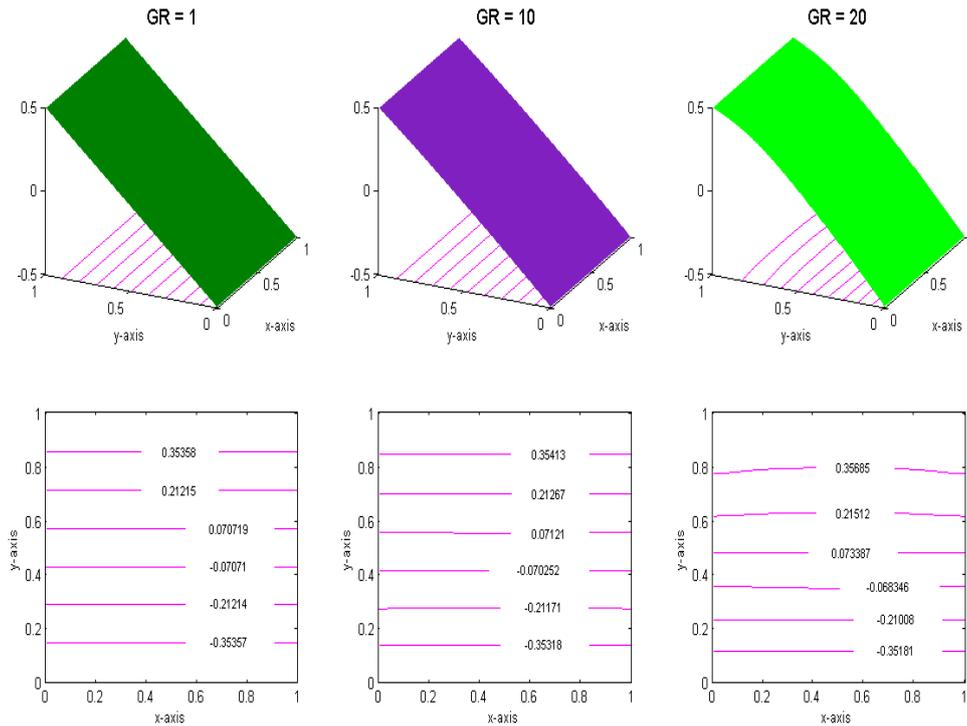
Figure 2a. Velocity and temperature contours for different values of Grashof number  $GR$  for  $BR = 2$  and  $A = 1$ .
