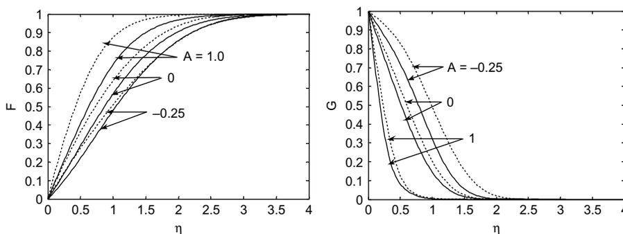
**Figure 5.** Effect of mass transfer parameter ( $A$ ) on (a) velocity profile and (b) temperature profile for  $t^* = 0$  (—) and  $t^* = 2$  (.....) with  $\varphi(t^*) = 1 + \varepsilon(t^*)^2$ ,  $\varepsilon = 0.25$ ,  $Ec = 0$ ,  $\bar{x} = 1.75$ ,  $T_\infty = 18.7^\circ\text{C}$ ,  $\Delta T_w = 10.0^\circ\text{C}$ ,  $w^* = 2\pi$ , variable viscosity and Prandtl number
