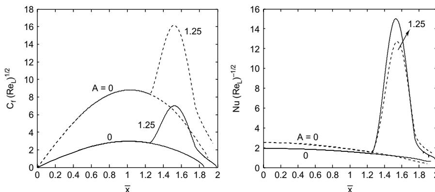
**Figure 6.** Effect of mass transfer parameter ( $A > 0$ ) on (a) skin friction coefficient and (b) heat transfer coefficient at times  $t^* = 0$  (—) and  $t^* = 2$  (----) with  $\varphi(t^*) = 1 + \varepsilon(t^*)^2$ ,  $\varepsilon = 0.25$ ,  $Ec = 0$ ,  $T_\infty = 18.7^\circ\text{C}$ ,  $\Delta T_w = 10.0^\circ\text{C}$ ,  $w^* = 2\pi$ , variable viscosity and Prandtl number
