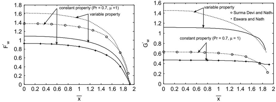
**Figure 4.** Effect of time on skin friction (—) and heat transfer (-----) coefficients for  $A = Ec = 0$ ,  $\bar{x} = 0.5, 1.0, 1.5, T_\infty = 18.7, \Delta T_w = 10$
