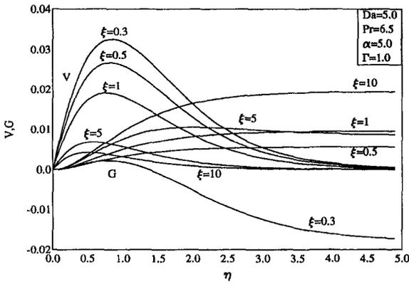
Fig. 8 Effects of  $\xi$  on tangential and normal velocity profiles
