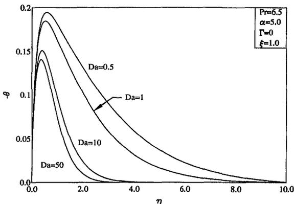
Fig. 13 Effects of  $Da$  on temperature profiles
