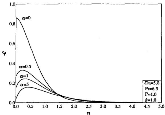
Fig. 5 Effects of  $\alpha$  on temperature profiles
