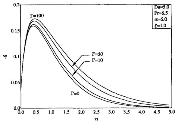
Fig. 17 Effects of  $\Gamma$  on temperature profiles
