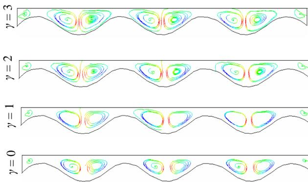
Fig. 5: Effect of  $\gamma$  on streamlines lines at  $\eta = 0$
