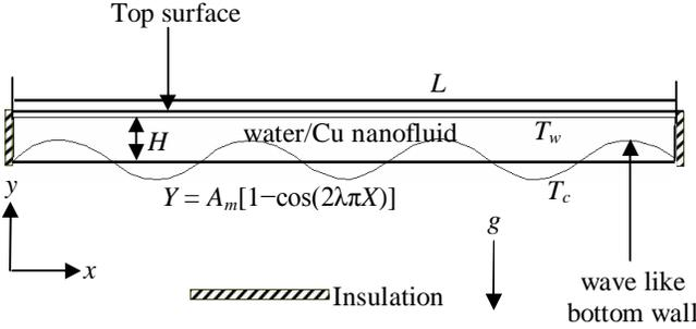
Fig. 1: Schematic diagram of the nanofluid layer
