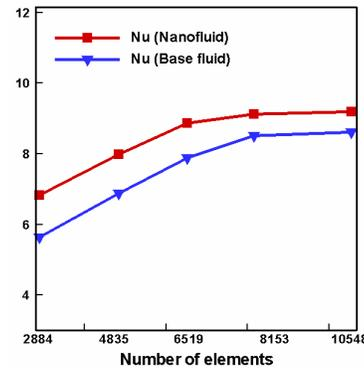
Fig. 3: Grid test for the current geometry
