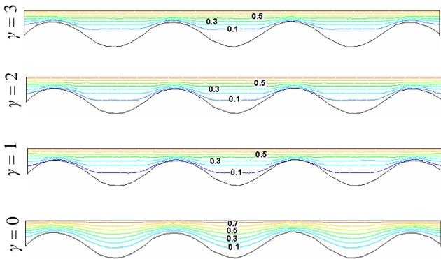
Fig. 4: Effect of  $\gamma$  on isothermal lines at  $\eta = 0$
