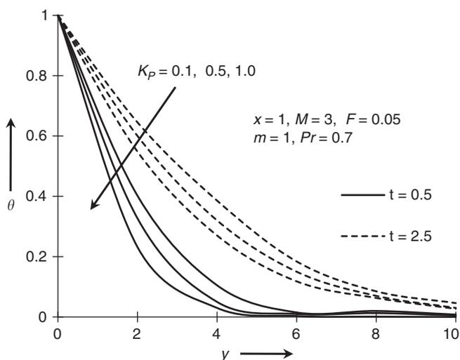
**Figure 10.** Spatial temperature distribution ( $\theta$ ) for the effect of Darcian drag force ( $K_P$ ) at  $t = 0.5$  and  $t = 2.5$
