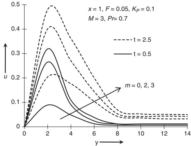
increasing power-law exponents in the plate surface temperature variations serve to accelerate the flow in the boundary layer. Here velocity overshoot has been observed at  $t = 2.5$  and  $m = 3$ .
