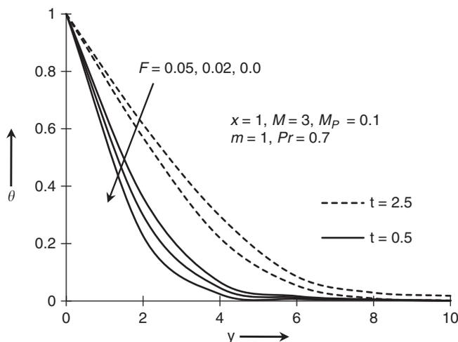
**Figure 6.** Spatial temperature distribution ( $\theta$ ) for the effect of radiation-conduction parameter ( $F$ ) at  $t = 0.5$  and  $t = 2.5$
