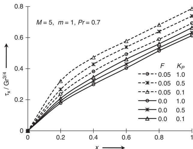
**Figure 11.** The effect of radiation-conduction and Darcian drag force on local skin friction
