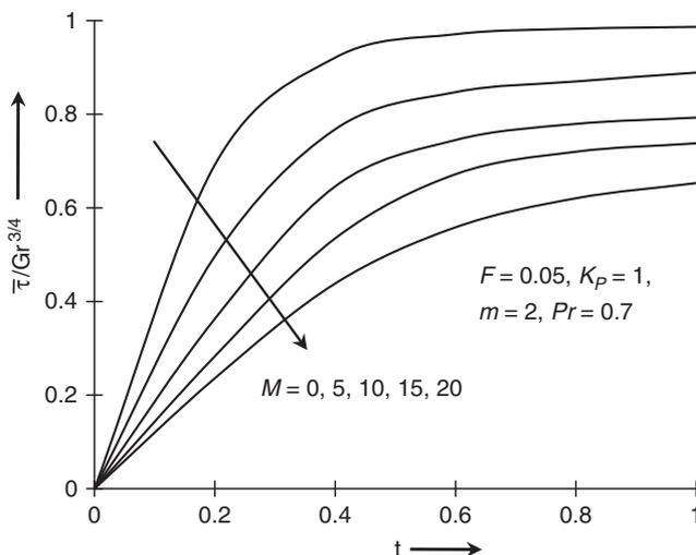
**Figure 3.** Average skin friction distribution for the effect of Hartmann hydromagnetic parameter
