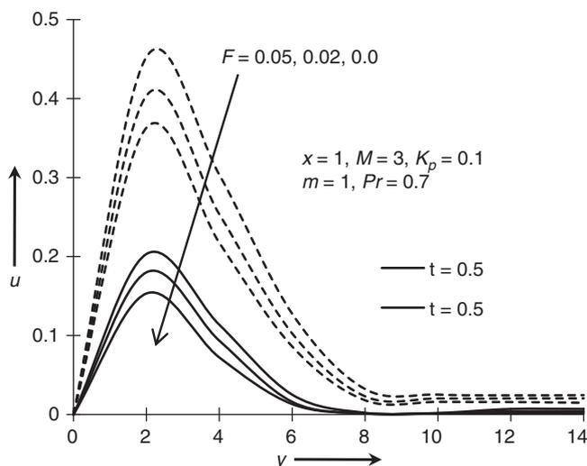
**Figure 7.** Spatial velocity distribution ( $u$ ) for the effect of radiation-conduction parameter ( $F$ )
