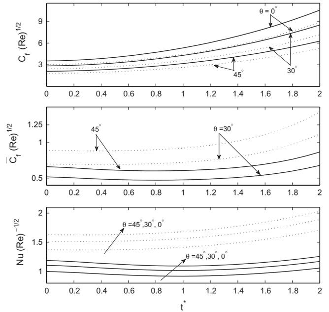
Fig. 5 Effects of time ( $t^*$ ) and yaw angle ( $\theta$ ) on skin friction coefficients (directions) and heat transfer coefficient at different positions  $\bar{x} = 0.5$  (-----) and  $\bar{x} = 1.4$  (—) with  $\phi(t^*) = 1 + \epsilon t^{*2}$ ,  $\epsilon = 0.25$ ,  $Ec = 0$ ,  $A = 0$ ,  $T_w = 18.7^\circ\text{C}$ ,  $\Delta T_w = 10.0^\circ\text{C}$ .
