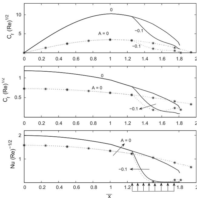
Fig. 7 Effect of injection ( $A < 0$ ) on skin friction coefficients (directions) and heat transfer coefficient for different times  $t^* = 0$  (-----) and  $t^* = 2$  (—) with  $\varphi(t^*) = 1 + \varepsilon t^{*2}$ ,  $\varepsilon = 0.25$ ,  $Ec = 0$ ,  $\theta = 30^\circ$ ,  $T_w = 18.7^\circ\text{C}$ ,  $\Delta T_w = 10.0^\circ\text{C}$ ,  $\omega^* = 2\pi$ . Slot  $[1.25 - \bar{x}_0^* = 1.75]$ .
