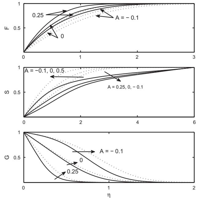
**Fig. 3** Effect of non-uniform mass transfer ( $A$ ) on velocity profiles ( $x, z$  directions) and temperature profile for different times  $t^* = 0$  (-----) and  $t^* = 2$  (—) at the point  $\bar{x} = 1.4$  with  $\varphi(t^*) = 1 + \varepsilon t^{*2}$ ,  $\varepsilon = 0.25$ ,  $Ec = 0$ ,  $\theta = 30^\circ$ ,  $T_w = 18.7^\circ\text{C}$ ,  $\Delta T_w = 10.0^\circ\text{C}$ ,  $\omega^* = 2\pi$ . Slot [ $\bar{x}_0 = 0.8 - \bar{x}_0^* = 1.3$ ].
