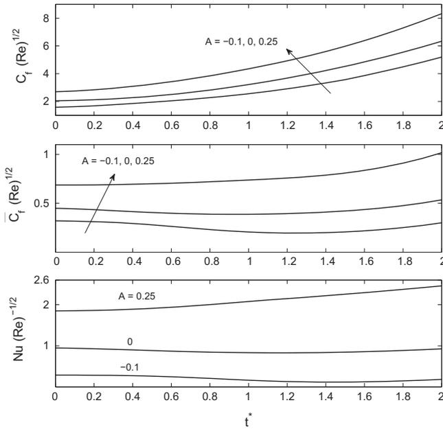
Fig. 4 Effects of time ( $t^*$ ) and mass transfer ( $A$ ) on skin friction coefficients (directions) and heat transfer coefficient at the point  $\bar{x} = 1.6$  with  $\phi(t^*) = 1 + \epsilon t^{*2}$ ,  $\epsilon = 0.25$ ,  $Ec = 0$ ,  $\theta = 30^\circ$ ,  $T_w = 18.7^\circ\text{C}$ ,  $\Delta T_w = 10.0^\circ\text{C}$ ,  $\omega^* = 2\pi$ . Slot  $[\bar{x}_0 = 1.0 - \bar{x}_0^* = 1.5]$ .
