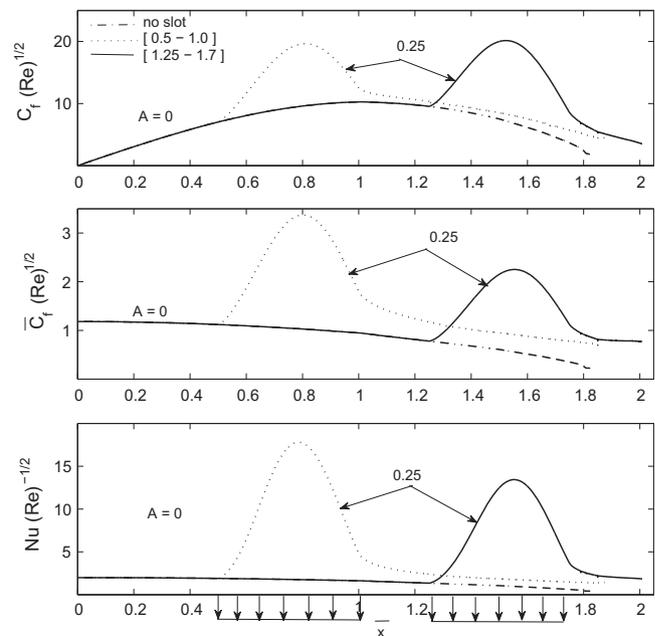
Fig. 8 Effect of slot location on skin friction coefficients (directions) and heat transfer coefficient at time  $t^* = 2$  with  $\varphi(t^*) = 1 + \varepsilon t^{*2}$ ,  $\varepsilon = 0.25$ ,  $Ec = 0$ ,  $\theta = 30^\circ$ ,  $T_w = 18.7^\circ\text{C}$ ,  $\Delta T_w = 10.0^\circ\text{C}$ ,  $\omega^* = 2\pi$ . Slot is placed at  $[\bar{x}_0^* = 0.5 - \bar{x}_0^* = 1.0]$  and  $[\bar{x}_0^* = 1.25 - \bar{x}_0^* = 1.75]$ .
