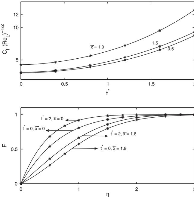
**Fig. 2** Comparison of skin friction and velocity profile with particular case of flow over cylinder for  $Ec = 0$ ,  $\theta = 0^\circ$ ,  $A = 0$ ,  $T_w = 18.7^\circ\text{C}$ ,  $\Delta T_w = 10.0^\circ\text{C}$ ,  $\varphi(t^*) = 1 + \varepsilon t^{*2}$ ,  $\varepsilon = 0.25$ . — present results, \* Eswara and Nath [9].
