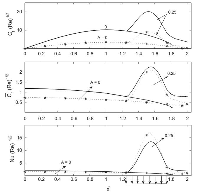
Fig. 6 Effect of suction ( $A > 0$ ) on skin friction coefficients (directions) and heat transfer coefficient for different times  $t^* = 0$  (-----) and  $t^* = 2$  (—) with  $\phi(t^*) = 1 + \epsilon t^{*2}$ ,  $\epsilon = 0.25$ ,  $Ec = 0$ ,  $\theta = 30^\circ$ ,  $T_w = 18.7^\circ\text{C}$ ,  $\Delta T_w = 10.0^\circ\text{C}$ ,  $\omega^* = 2\pi$ . Slot  $[\bar{x}_0 = 1.25 - \bar{x}_0^* = 1.75]$ .
