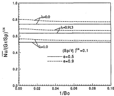
Fig. 4 Effect of surface tension on dimensionless mean heat transfer coefficient
