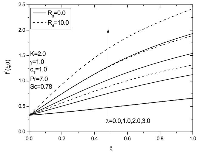
**Figure 12** Effects of  $\lambda$  and  $R_d$  on temperature profiles
