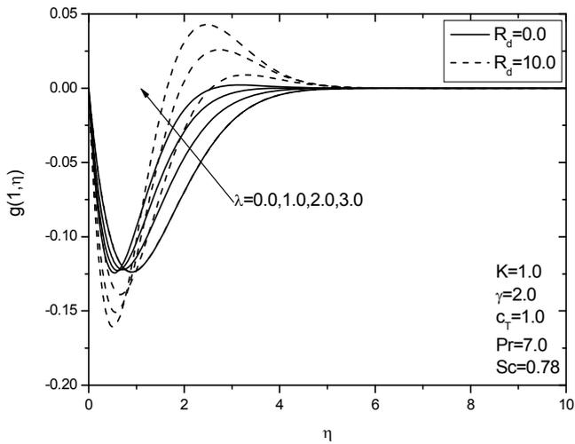
**Figure 14** Effects of  $\lambda$  and  $R_d$  on the skin-friction coefficient
