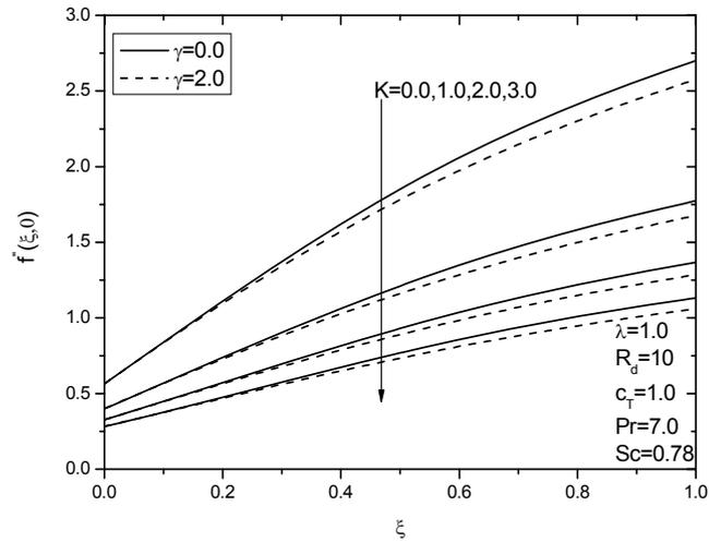
**Figure 7** Effects of  $K$  and  $\gamma$  on the wall couple stress
