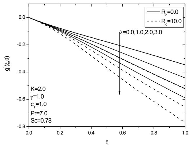
**Figure 13** Effects of  $\lambda$  and  $R_d$  on concentration profiles
