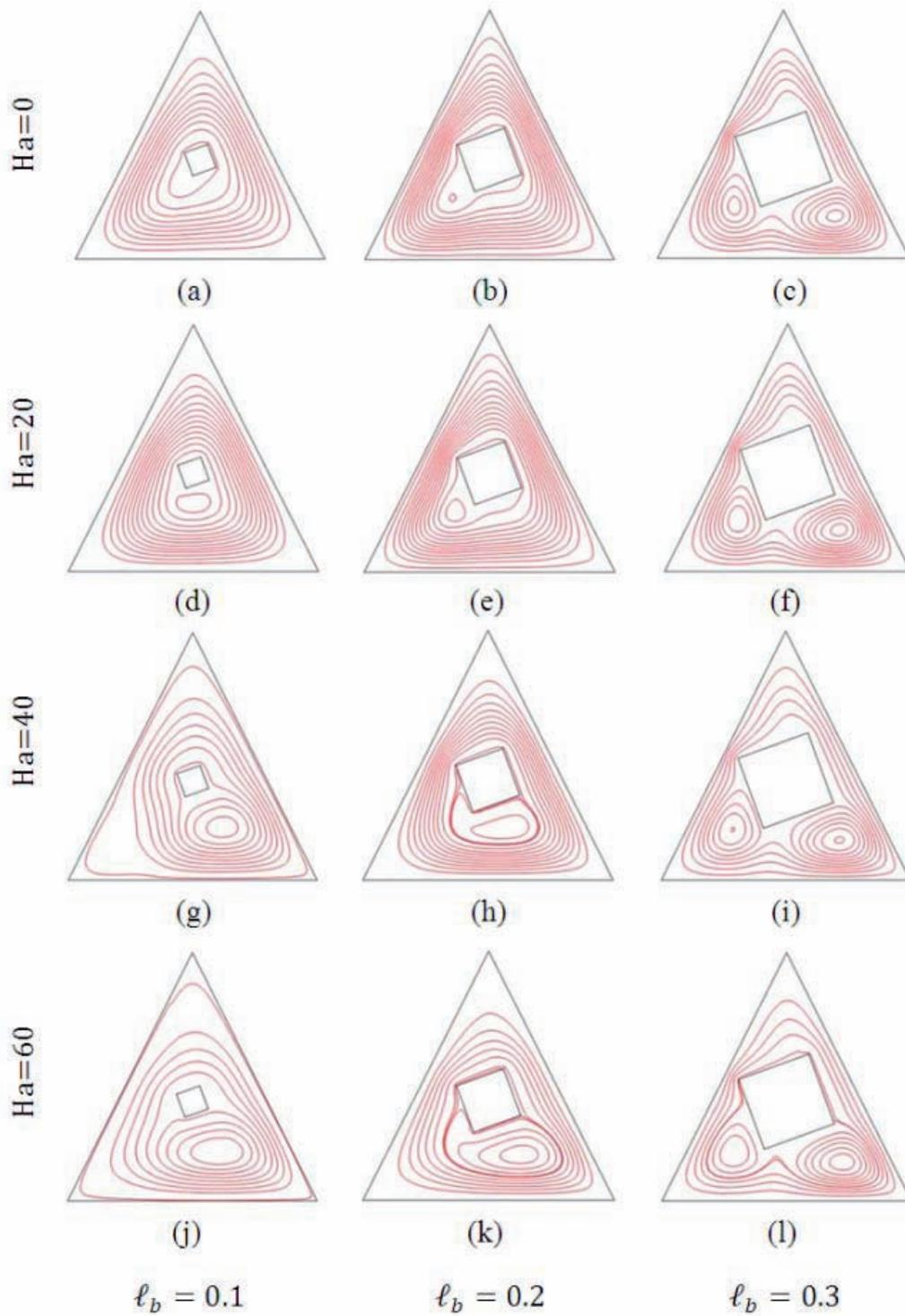
**FIG. 5:** Streamlines for different sizes of the square cavity  $l_b$  and Hartmann number  $Ha$  with  $Ra = 10^5$ ,  $Pr = 0.7$ ,  $Da = 10^{-3}$ , and  $\lambda = 0$ .
