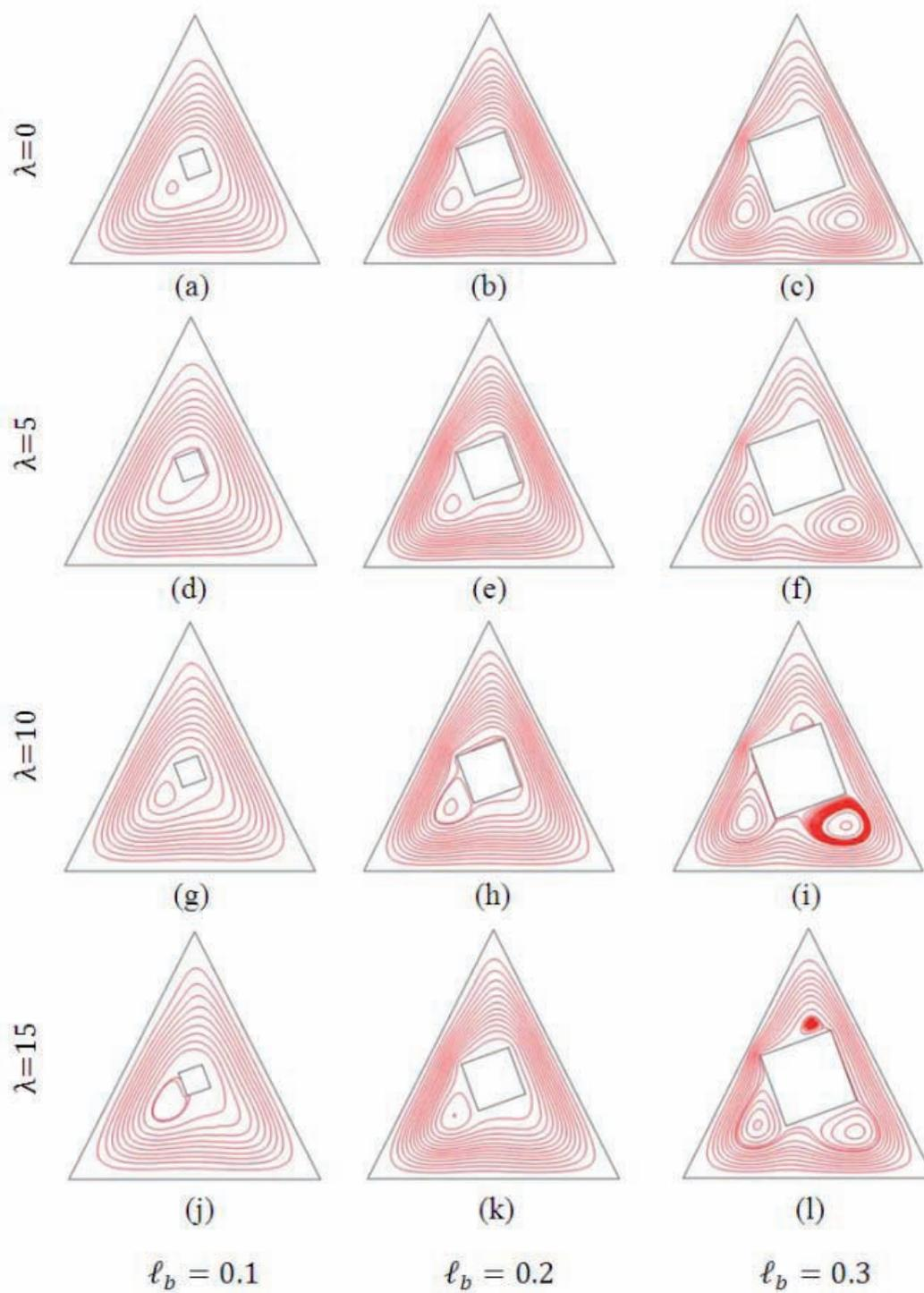
**FIG. 3:** Streamlines for different sizes of the square cavity  $\ell_b$  and heat generation parameter  $\lambda$  with  $Ra = 10^5$ ,  $Pr = 0.7$ ,  $Da = 10^{-3}$ , and  $Ha = 0$ .
