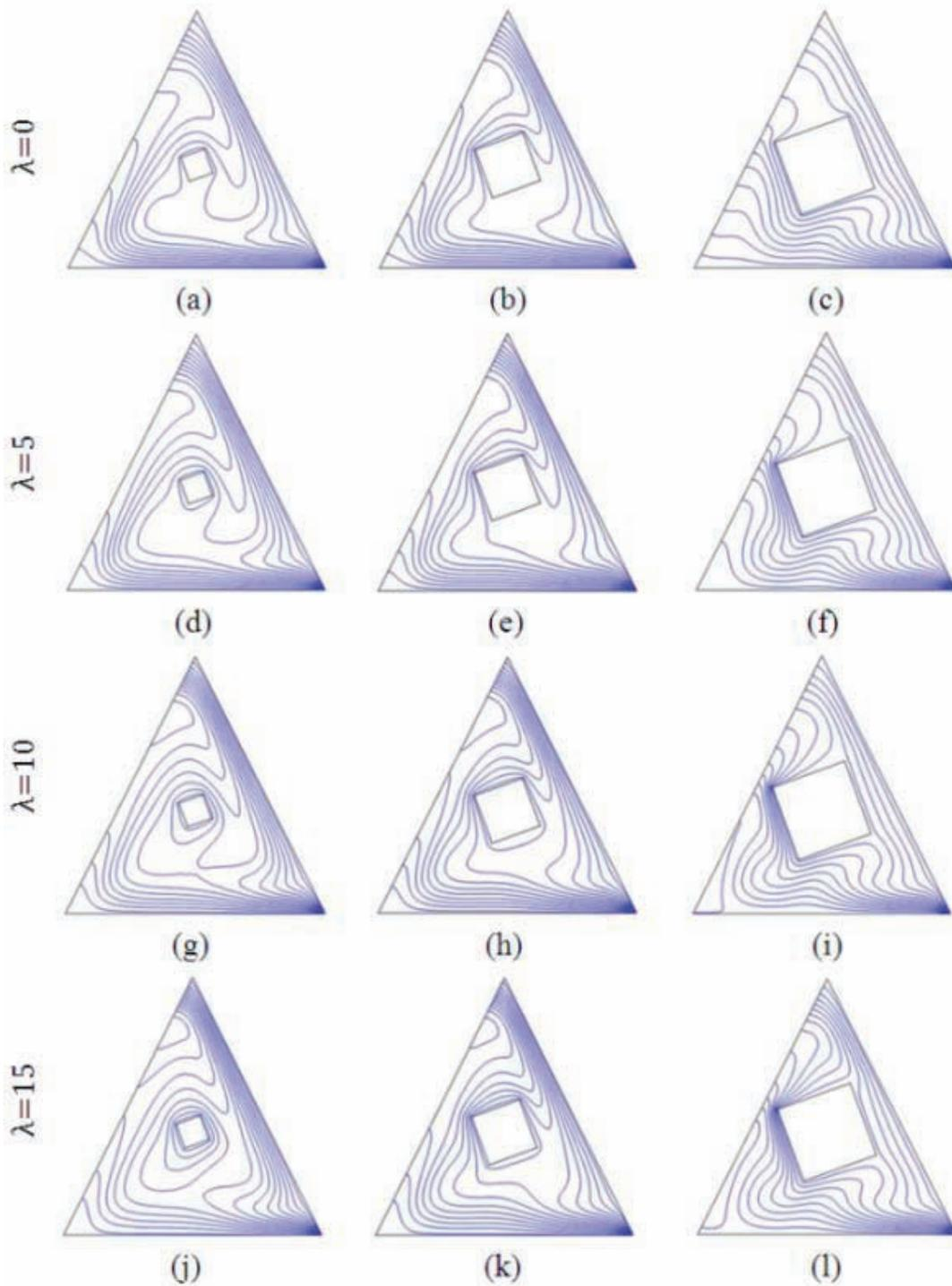
**FIG. 4:** Isotherms for different sizes of the square cavity  $l_b$  and heat generation parameter  $\lambda$  with  $Ra = 10^5$ ,  $Pr = 0.7$ ,  $Da = 10^{-3}$ , and  $Ha = 0$ .
