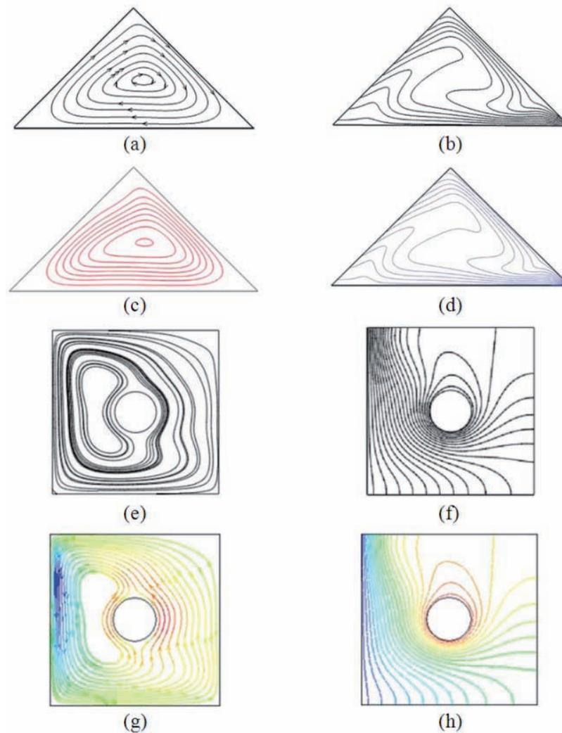
**FIG. 2:** A comparison for streamlines (left column) and isotherms (right column) with Saha and Gu (2012) (**a, b**) and present study (**c, d**) for  $Ra = 10^5$ ,  $Pr = 0.7$ ,  $Da = 10^{-3}$ ,  $\lambda = 0$  and  $Ha = 0$  and Parvin and Nasrin (2011) (**e, f**) and present study (**g, h**) for  $Ra = 10^5$ ,  $Pr = 0.7$  and  $Ha = 50$ .
