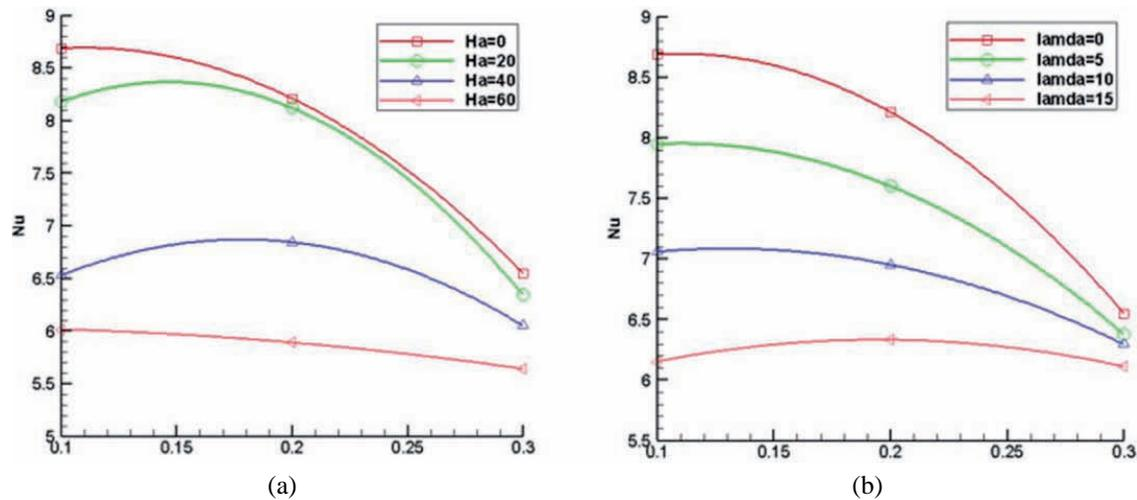
**FIG. 7:** Effect of size of the square body  $l_b$  on Nu with different values of (a) Hartmann number (Ha) and (b) heat generation parameter ( $\lambda$ ).
