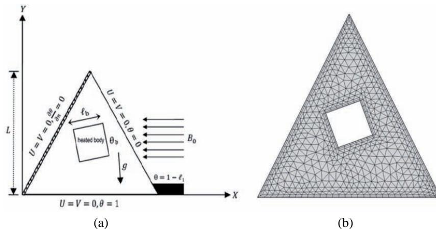
**FIG. 1:** (a) Schematic diagram of the enclosure with boundary conditions. (b) Mesh structure of elements for triangular enclosure.
