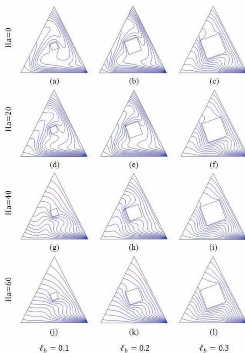
**FIG. 6:** Isotherms for different sizes of the square cavity  $l_b$  and Hartmann number  $Ha$  with  $Ra = 10^5$ ,  $Pr = 0.7$ ,  $Da = 10^{-3}$ , and  $\lambda = 0$ .
