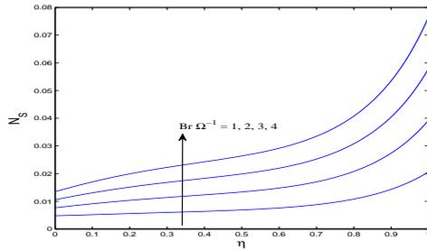
**Figure 14:**  $N_S$  for  $Br\Omega^{-1}$  when  $Pr = 0.71$ ,  $\beta_1 = 0.1$ ,  $\beta_2 = 0.1$ ,  $Ec = 0.5$ ,  $Bi_1 = 0.1$ ,  $Bi_2 = 0.1$ ,  $M^2 = 5$
