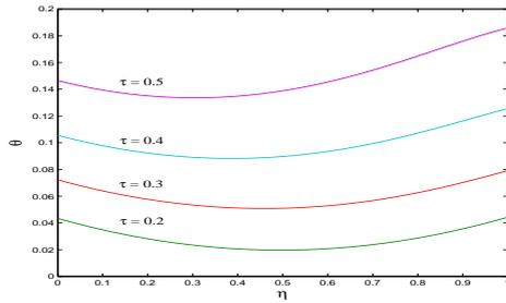
**Figure 10:** Temperature profiles for time  $\tau$  when  $Pr = 0.72, Bi_1 = 0.1, Bi_2 = 0.1, Ec = 0.5$
