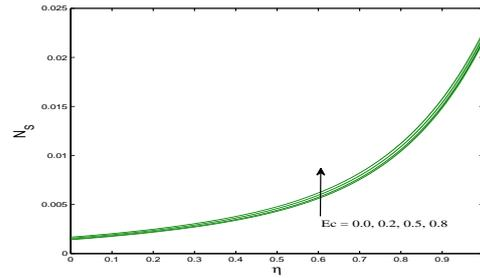
**Figure 12:**  $N_S$  for  $Ec$  when  $Pr = 0.71, \beta_1 = 0.1, \beta_2 = 0.1, M^2 = 5, Bi_1 = 0.1, Bi_2 = 0.1, Br\Omega^{-1} = 1$
