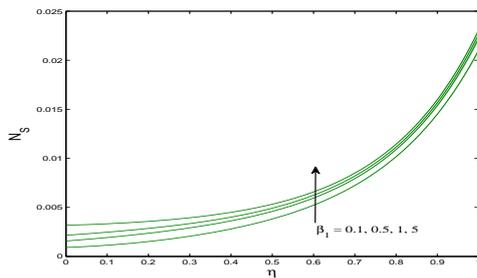
**Figure 15:**  $N_S$  for  $\beta_1$  when  $Pr = 0.71$ ,  $M^2 = 5$ ,  $\beta_2 = 0.1$ ,  $Ec = 0.5$ ,  $Bi_1 = 0.1$ ,  $Bi_2 = 0.1$ ,  $Br\Omega^{-1} = 1$
