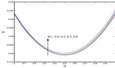
**Figure 6:** Temperature profiles for different  $Ec$  when  $Pr = 0.72, Bi_1 = 0.1, Bi_2 = 0.1, \tau = 0.2$
