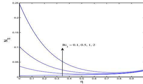
**Figure 17:**  $N_S$  for  $Bi_1$  when  $Pr = 0.71$ ,  $\beta_1 = 0.1$ ,  $\beta_2 = 0.1$ ,  $Ec = 0.5$ ,  $M^2 = 5$ ,  $Bi_2 = 0.1$ ,  $Br\Omega^{-1} = 1$
