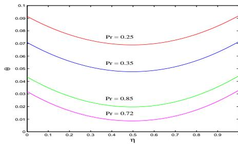
**Figure 7:** Temperature profiles for different  $Pr$  when  $Ec = 0.5, Bi_1 = 0.1, Bi_2 = 0.1, \tau = 0.2$
