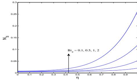
**Figure 18:**  $N_S$  for  $Bi_2$  when  $Pr = 0.71$ ,  $\beta_1 = 0.1$ ,  $\beta_2 = 0.1$ ,  $Ec = 0.5$ ,  $M^2 = 5$ ,  $Bi_2 = 0.1$ ,  $Br\Omega^{-1} = 1$
