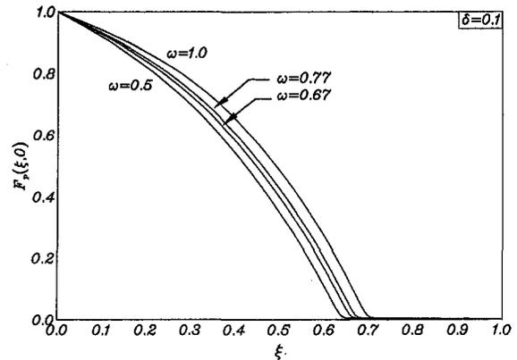
Fig. 8 Wall particle-phase tangential velocity profiles
