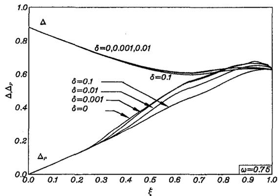
Fig. 1 Fluid and particle-phase displacement thicknesses profiles
