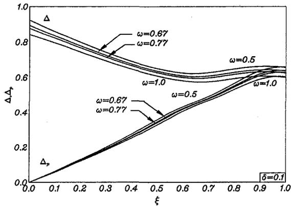
Fig. 6 Fluid and particle-phase displacement thicknesses profiles
