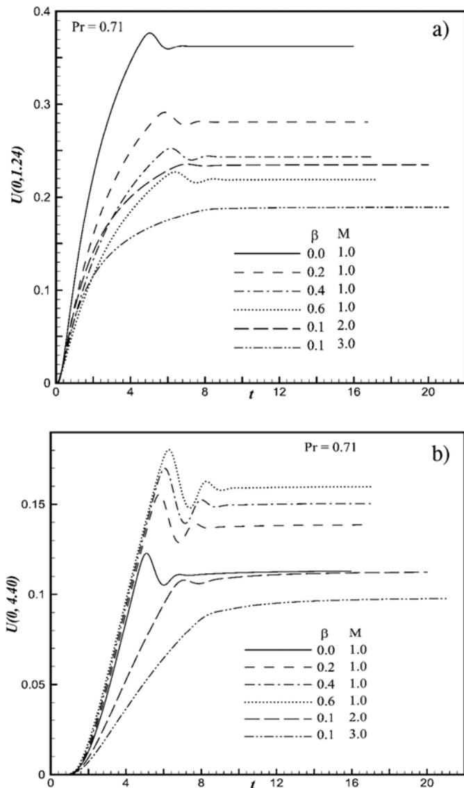
Fig. 3. Time-dependent velocity profile ( $U$ ) versus time ( $t$ ) for various values of  $\beta$  and  $M$  at the location (a) (0, 1.24); & (b) (0, 4.40).
