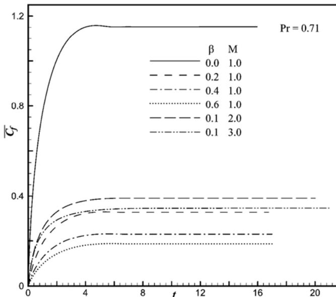
Fig. 7. Average momentum transport coefficient ( $\overline{C_f}$ ) for different values of  $\beta$  and  $M$ .
