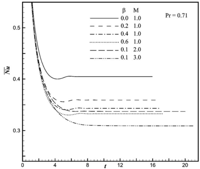
Fig. 8. Average heat transport coefficient ( $\overline{Nu}$ ) for different values of  $\beta$  and  $M$ .
