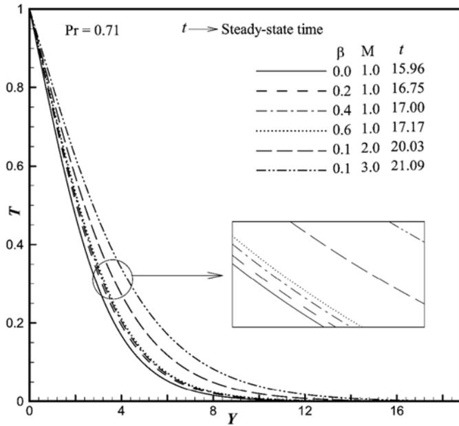
Fig. 6. Simulated time-independent temperature profile ( $T$ ) versus  $Y$  at  $X = 1.0$  for various values of  $\beta$  and  $M$ .
