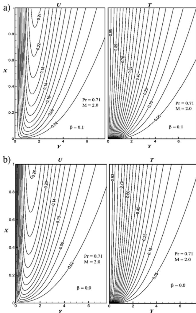
Fig. 13. Time-independent state contours of velocity ( $U$ ) and temperature ( $T$ ) for (a) couple stress fluid ( $\beta = 0.1$ ); & (b) Newtonian fluid ( $\beta = 0.0$ ).
