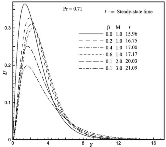
Fig. 4. Simulated time-independent state velocity profile ( $U$ ) versus  $Y$  at  $X = 1.0$  for various values of  $\beta$  and  $M$ .
