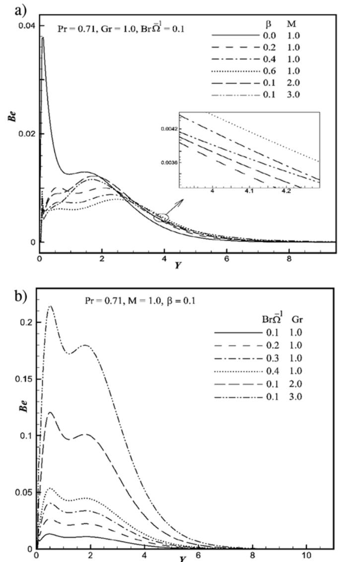
Fig. 11. Simulated steady-state Bejan profile ( $Be$ ) versus  $Y$  at  $X = 1.0$  for distinct values of (a)  $\beta$  and  $M$ ; & (b)  $Br\Omega^{-1}$  and  $Gr$ .
