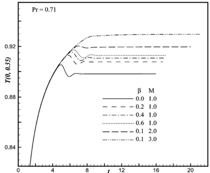
Fig. 5. Simulated time-dependent temperature profile ( $T$ ) versus time ( $t$ ) at the location (0, 0.35) for distinct values of  $\beta$  and  $M$ .
