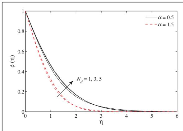
**Figure 13.** Concentration profile for different values of  $N_d$  when  $We = 2, m = 2, Nt = 0.2, Nb = 0.2, Q_w = 1.2, n = 1.5, Pr = 1, \beta = 2, E = 10, n_1 = \delta = 0.5, Sc = 1$ .
