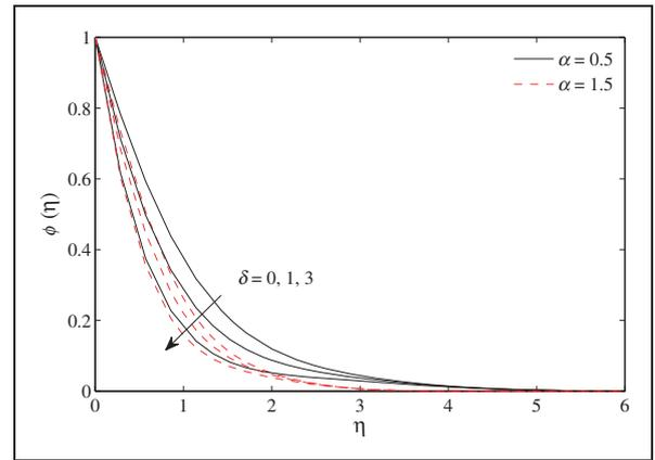
**Figure 15.** Concentration profile for different values of  $\delta$  when  $We = 2, m = 2, Nt = 0.5, Nb = 0.5, Q_w = 1.5, n = 1.5, Pr = 1, \beta = 5, E = 3, n_1 = 0.5, Sc = 1$ .
