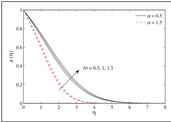
**Figure 7.** Temperature profile for different values of  $Nt$  when  $We = 2, m = 2, n = 1.5, Nb = 1, Q_w = 1.2, N_d = 1, Pr = 1$ .
