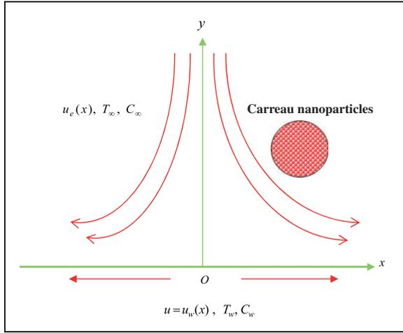
**Figure 1.** Flow diagram of the problem.
