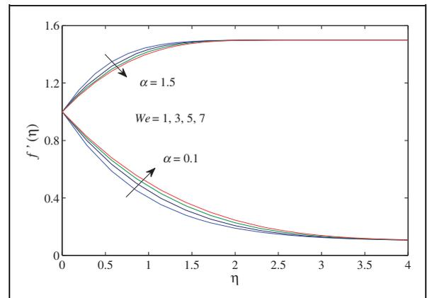
**Figure 6.** Velocity profile for different values of  $We$  when  $n = 0.5, m = 1.5$ .
