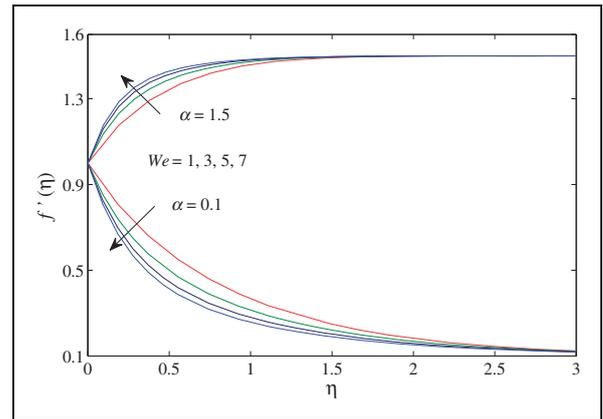
**Figure 5.** Velocity profile for different values of  $We$  when  $n = 1.5, m = 1.5$ .
