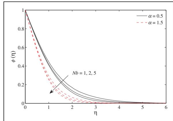
**Figure 10.** Concentration profile for different values of  $Nb$  when  $We = 2, m = 2, Nt = 0.5, Q_w = 1.2, N_d = 1, Pr = 1, \beta = 2, E = 10, n_1 = \delta = 0.5, Sc = 1$ .
