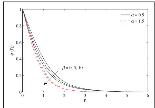
**Figure 16.** Concentration profile for different values of  $\beta$  when  $We = 2, m = 2, Nt = 0.5, Nb = 2.5, Q_w = 1.5, n = 1.5, Pr = 1, \delta = 0.5, E = 4, n_1 = 0.5, Sc = 1$ .
