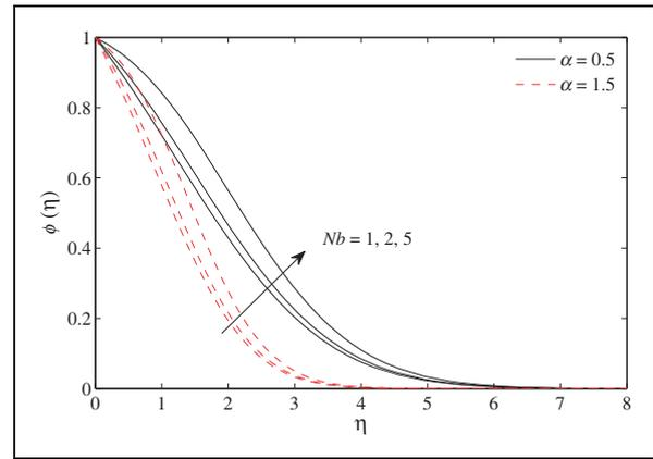
**Figure 9.** Temperature profile for different values of  $Nb$  when  $We = 2, m = 2, Nt = 0.5, Q_w = 1.2, N_d = 1, Pr = 1$ .
