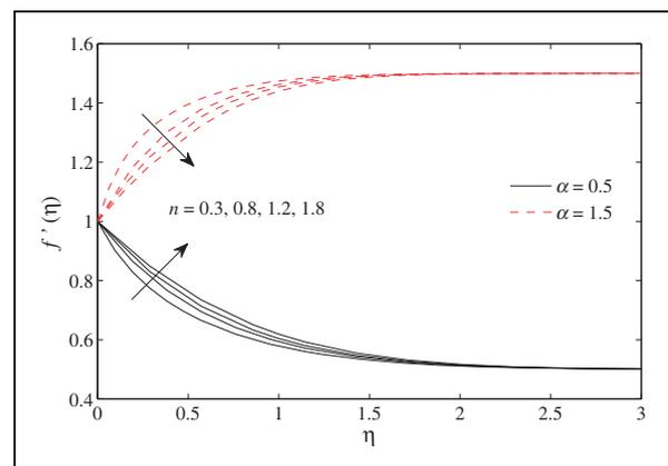
**Figure 11.** Velocity profile for different values of  $n$  when  $We = 2, m = 2$ .
