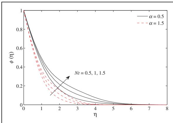
**Figure 8.** Concentration profile for different values of  $Nt$  when  $We = 2, m = 2, n = 1.5, Nb = 1.5, Q_w = 1.2, N_d = 1, Pr = 1, \beta = 2, E = 10, n_1 = \delta = 0.5, Sc = 1$ .
