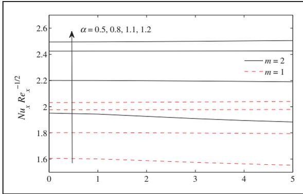
**Figure 18.** Nusselt number versus  $We$  for various values of  $\alpha$  when  $Nb = 1.2, n = 0.5, Nt = 0.5, Q_w = 1.2, N_d = 2, Pr = 1$ .
