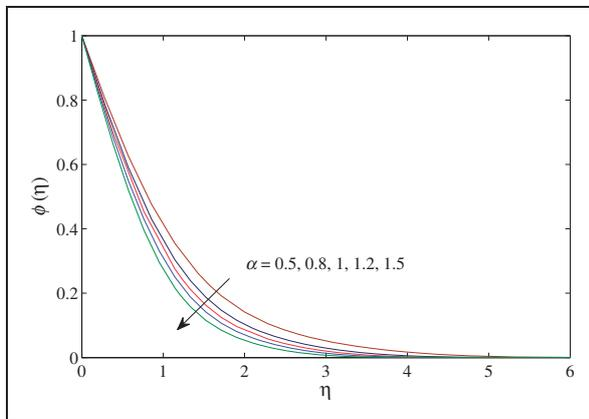
**Figure 4.** Concentration profile for different values of  $\alpha$  when  $We = 2, n = 0.8, m = 1.5, Nb = 1.5, Nt = 0.5, Q_w = 1.5, N_d = 2, Pr = 1, \beta = 3, E = 6, n_1 = \delta = 0.5, Sc = 1$ .
