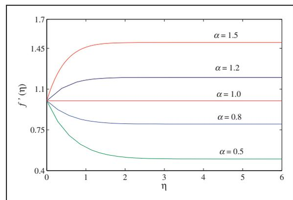
**Figure 2.** Velocity profile for different values of  $\alpha$  when  $We = 2, n = 0.8, m = 1.5$ .
