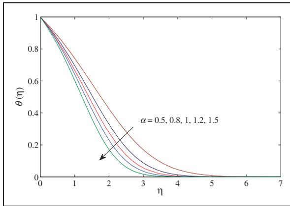
**Figure 3.** Temperature profile for different values of  $\alpha$  when  $We = 2, n = 0.8, m = 1.5, Nb = 1.5, Nt = 0.5, Q_w = 1.5, N_d = 2, Pr = 1$ .
