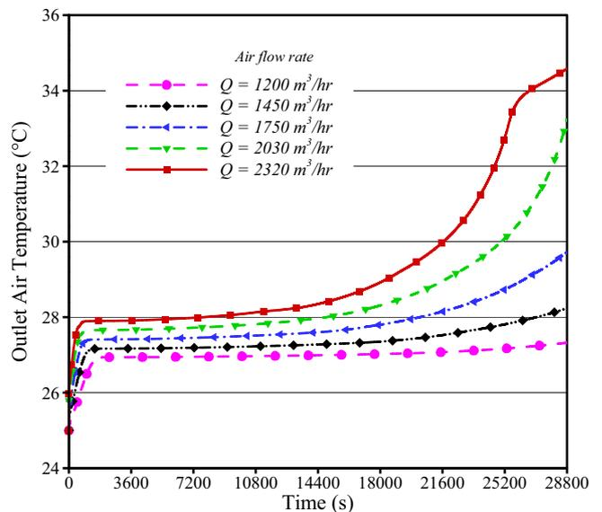
Fig. 7. The effect of air flow rate on the outlet air temperature.
