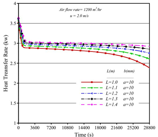
**Fig. 4.** The effect of PCM slab length on the heat transfer rate.
