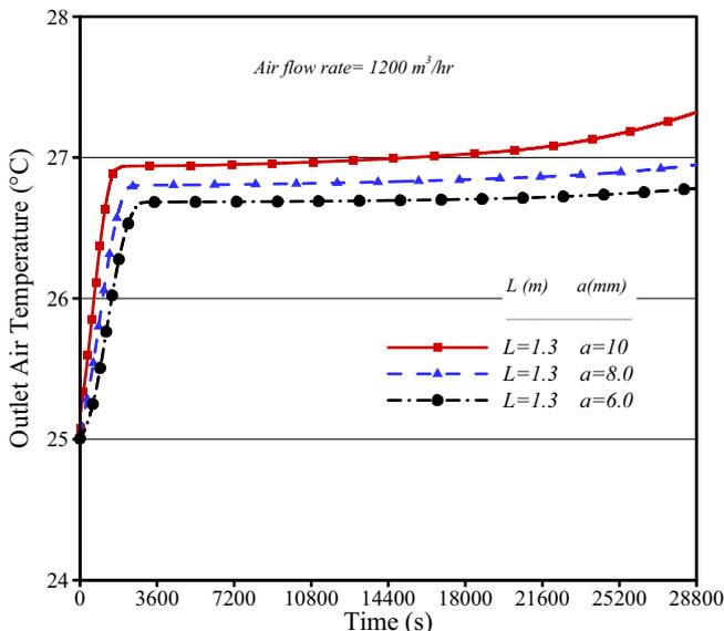
Fig. 5. The effect of PCM slab thickness on the outlet air temperature.
