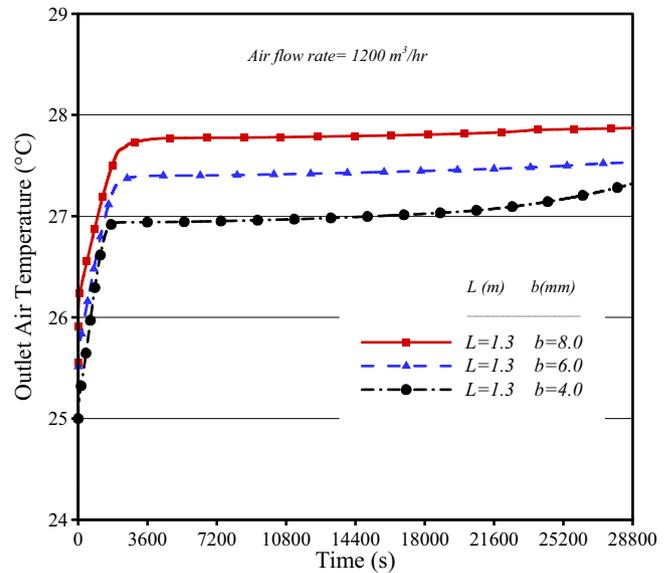
Fig. 6. The effect of air channel thickness on the outlet air temperature.
