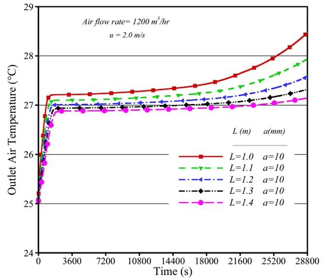
**Fig. 3.** The effect of PCM slab length on the outlet air temperature.
