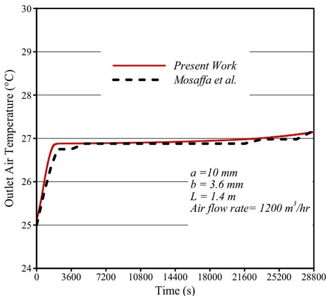
**Fig. 2.** Comparison of outlet air temperature time history by the effective heat capacity method and enthalpy method.
