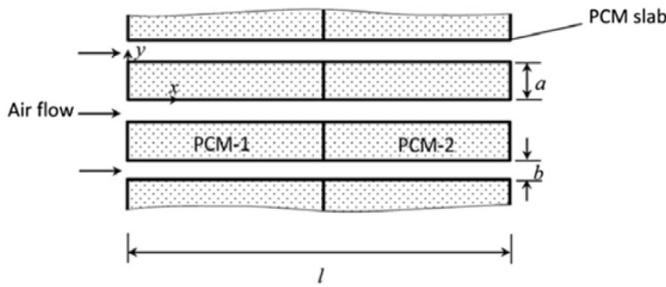
Fig. 1. Schematic diagram of the LHTS unit [16].
