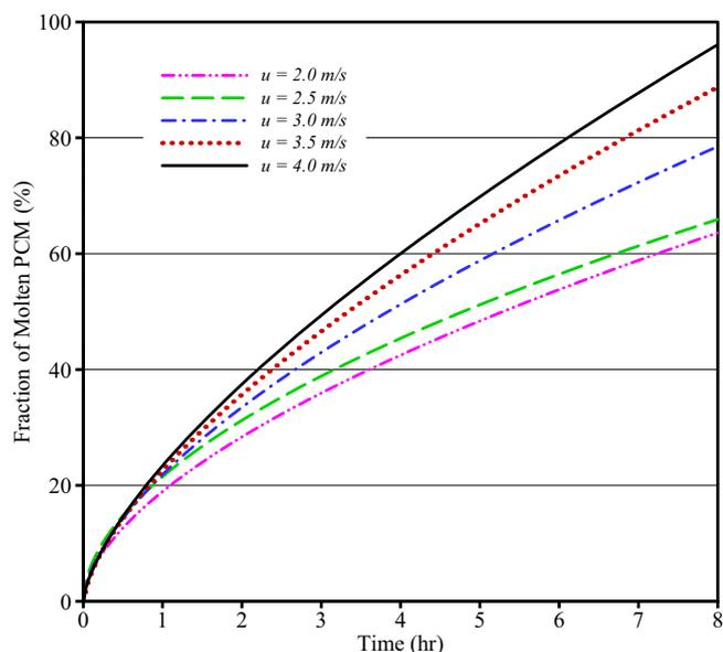
Fig. 8. The effect of air velocity on the fraction of molten PCM.
