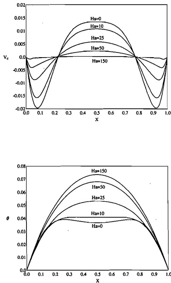
**Figure 6.** Vertical velocity and temperature profiles along the horizontal midheight of the vertical enclosure for various Hartmann numbers at  $Ra = 6.4 \times 10^5$  and  $Da = \infty$ .
