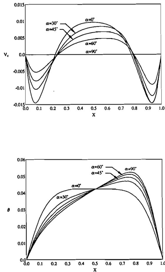
**Figure 8.** Vertical velocity and temperature profiles along the horizontal midheight of the enclosure for various inclination angles  $\alpha$  at  $Ra = 6.4 \times 10^5$ ,  $Da = 1 \times 10^{-2}$ , and  $Ha = 5$ .
