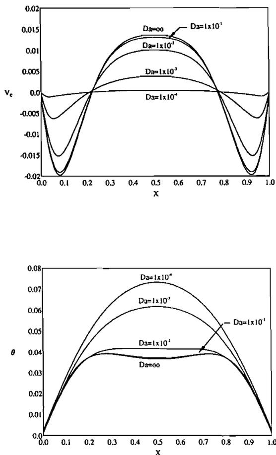
Figure 7. Vertical velocity and temperature profiles along the horizontal midheight of the vertical enclosure for various Darcy numbers at  $Ra = 6.4 \times 10^5$  and  $Ha = 0$ .
