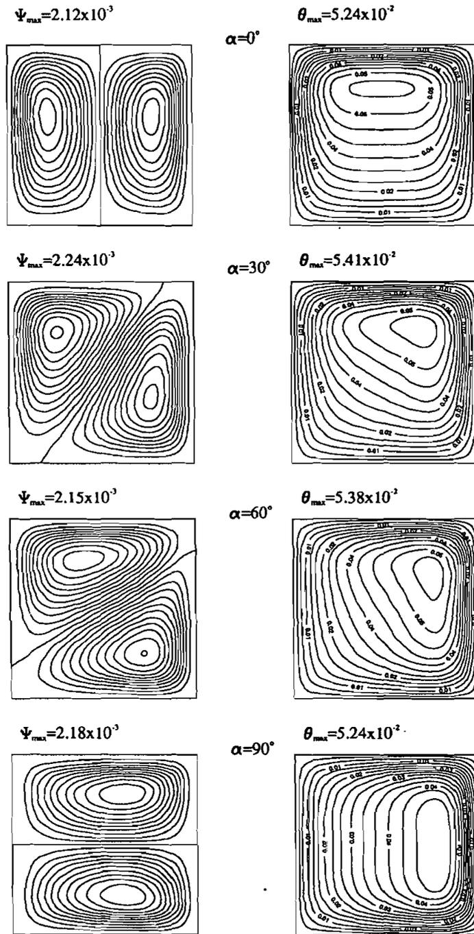
Figure 5. Steady state solution of flow patterns and isothermal field for various inclination angles at  $Ra = 6.4 \times 10^5$ ,  $Da = 1 \times 10^{-2}$ , and  $Ha = 5$ .
