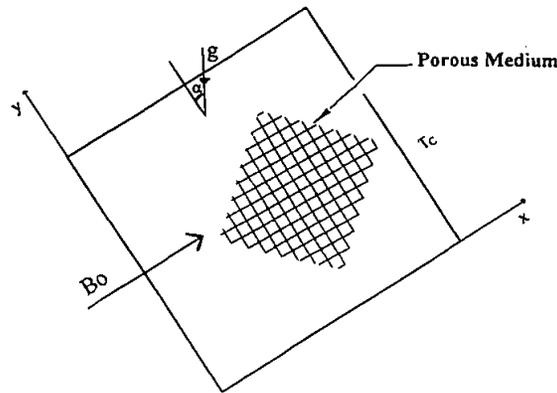
Figure 1. Schematic diagram of tilted porous-medium-filled square enclosure configuration with heat-generating fluid in the presence of a magnetic field effect.
