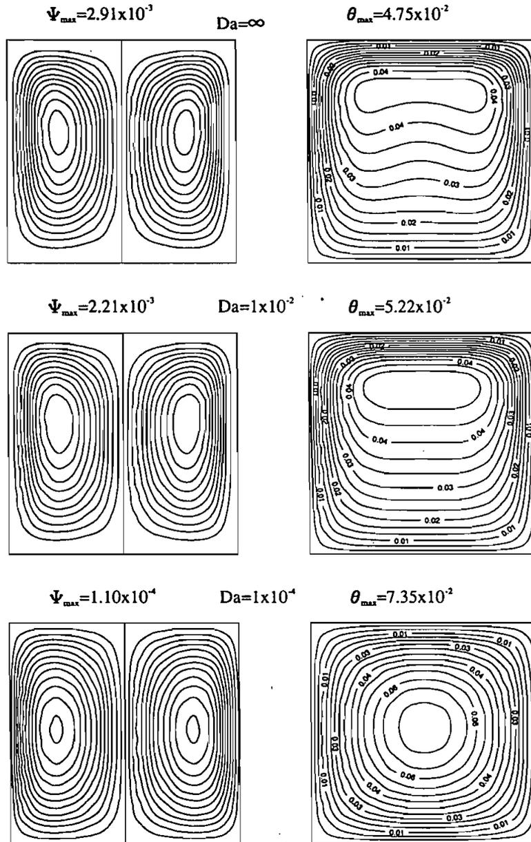
**Figure 4.** Steady state flow patterns and isothermal field of a vertical enclosure for various Darcy numbers at  $Ra = 6.4 \times 10^5$  and  $Ha = 0$ .
