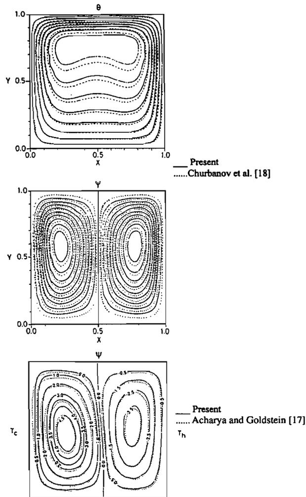
**Figure 2.** Comparison of steady state flow patterns and isothermal field of a vertical enclosure between the present prediction and other numerical results.
