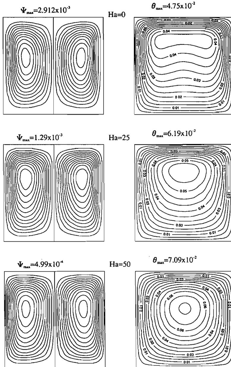
**Figure 3.** Steady state flow patterns and isothermal field of a vertical enclosure for various Hartmann numbers at  $Ra = 6.4 \times 10^5$  and  $Da = \infty$ .
