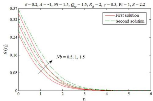
**Figure 9** The concentration profiles for different values of  $Nb$
