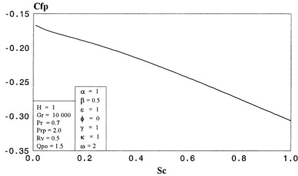
Fig. 15. Effect of  $Sc$  on the particle-phase coefficient of friction.
