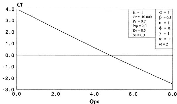
Fig. 14. Effect of  $Q_{p0}$  on the fluid-phase coefficient of friction.
