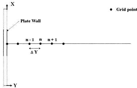
Fig. 2. Finite difference grid representation.
