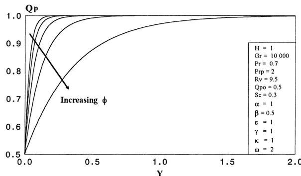
Fig. 7. Effect of the tilt angle on the particle-phase density profile.
