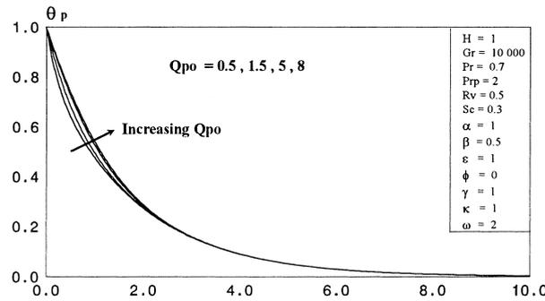
Fig. 6. Effect of  $Q_{p0}$  on the particle-phase temperature profile.
