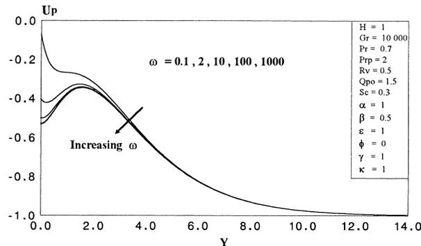
Fig. 11. Effect of  $\omega$  on the particle-phase velocity profile.
