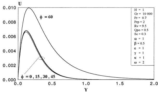
Fig. 8. Effect of the tilt angle on the fluid velocity profile.
