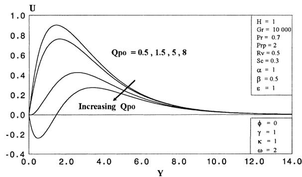
Fig. 4. Effect of  $Q_{p0}$  on the fluid velocity profile.
