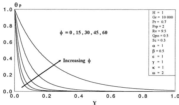
Fig. 9. Effect of the tilt angle on the particle-phase temperature profile.
