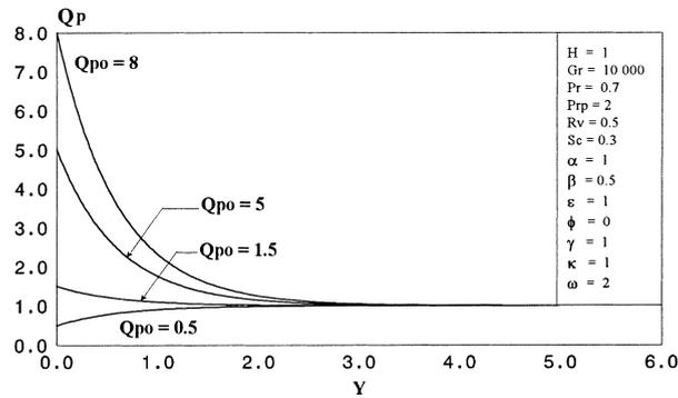
Fig. 3. Effect of  $Q_{p0}$  on the particle-phase density profile.
