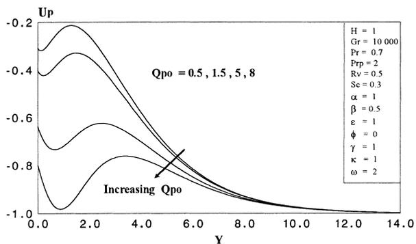
Fig. 5. Effect of  $Q_{p0}$  on the particle-phase velocity profile.
