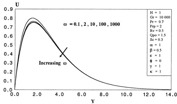
Fig. 10. Effect of  $\omega$  on the fluid velocity profile.
