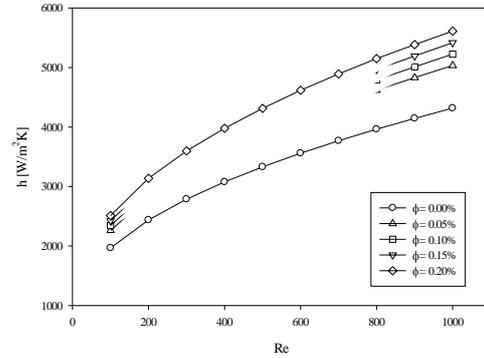
**Fig. 3. The convective heat transfer coefficients for diamond-Fe<sub>3</sub>O<sub>4</sub>/water hybrid nanofluid.**
