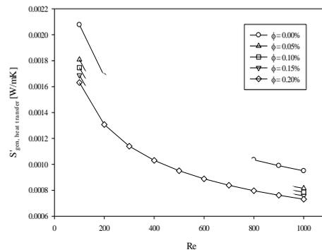
**Fig. 11.** The entropy generation rate due to heat transfer for diamond-Fe<sub>3</sub>O<sub>4</sub>/water hybrid nanofluid.
