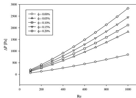
**Fig. 7. The pressure drop for diamond-Fe<sub>3</sub>O<sub>4</sub>/water hybrid nanofluid.**
