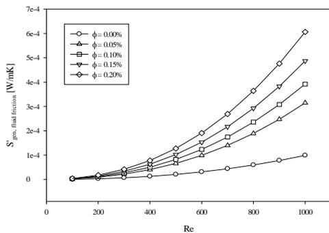
**Fig. 13.** The entropy generation rate due to fluid friction for diamond-Fe<sub>3</sub>O<sub>4</sub>/water hybrid nanofluid.
