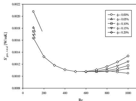
**Fig. 15.** The total entropy generation rate for diamond-Fe<sub>3</sub>O<sub>4</sub>/water hybrid nanofluid.
