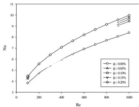
**Fig. 5. The Nusselt number for diamond-Fe<sub>3</sub>O<sub>4</sub>/water hybrid nanofluid.**
