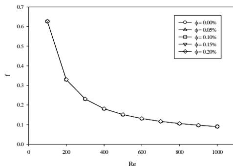
**Fig. 9.** The Darcy friction factor for diamond-Fe<sub>3</sub>O<sub>4</sub>/water hybrid nanofluid.
