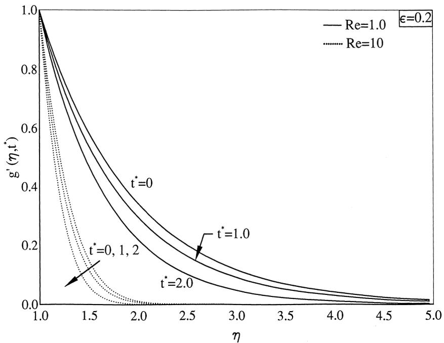
Fig. 7. Velocity profiles  $g'(\eta, t^*)$  for  $\phi(t^*) = 1 + \epsilon t^{*2}$ ,  $\epsilon = 0.2$ ,  $t^* = 0, 1, 2$ ,  $Re = 1.0, 10.0$ .
