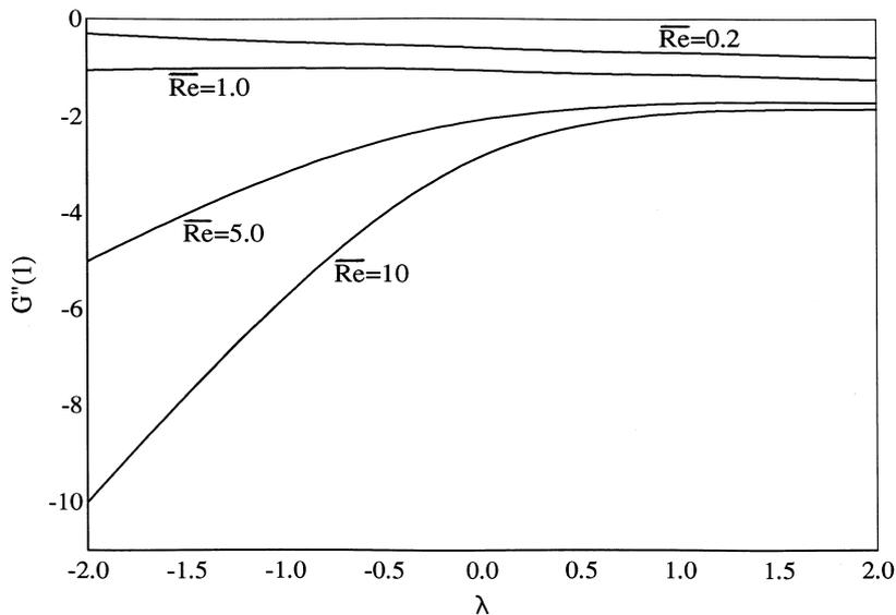
Fig. 12. Variation of the surface shear stress  $G''(1)$  with  $\lambda$  and  $\overline{Re}$ .
