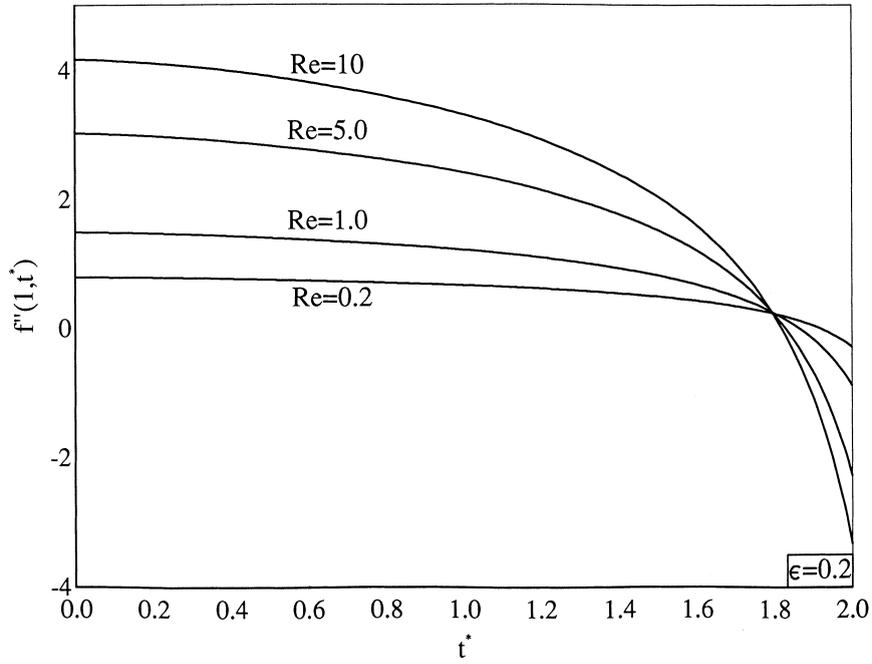
Fig. 4. Variation of the surface shear stress  $f''(1, t^*)$  with time  $t^*$  for  $\phi(t^*) = 1 - \epsilon t^{*2}$ ,  $\epsilon = 0.2$ ,  $Re = 0.2, 1.0, 5.0, 10.0$ .
