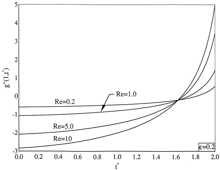
Fig. 5. Variation of the surface shear stress  $g''(1, t^*)$  with time  $t^*$  for  $\phi(t^*) = 1 - \epsilon t^{*2}$ ,  $\epsilon = 0.2$ ,  $Re = 0.2, 1.0, 5.0, 10.0$ .
