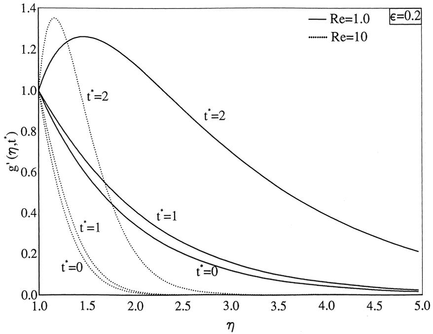
Fig. 9. Velocity profiles  $g'(\eta, t^*)$  for  $\phi(t^*) = 1 - \epsilon t^{*2}$ ,  $\epsilon = 0.2$ ,  $t^* = 0, 1, 2$ ,  $Re = 1.0, 10.0$ .
