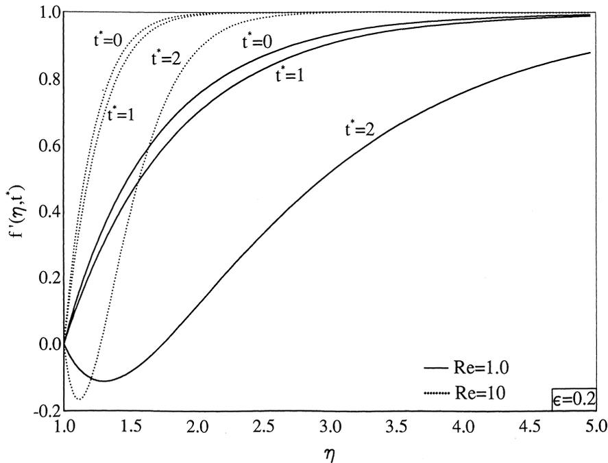
Fig. 8. Velocity profiles  $f'(\eta, t^*)$  for  $\phi(t^*) = 1 - \epsilon t^{*2}$ ,  $\epsilon = 0.2$ ,  $t^* = 0, 1, 2$ ,  $\text{Re} = 1.0, 10.0$ .
