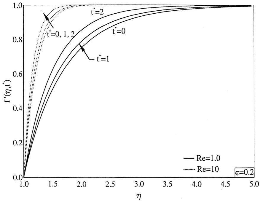
Fig. 6. Velocity profiles  $f'(\eta, t^*)$  for  $\phi(t^*) = 1 + \epsilon t^{*2}$ ,  $\epsilon = 0.2$ ,  $t^* = 0, 1, 2$ ,  $Re = 1.0, 10.0$ .
