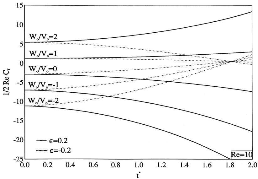
Fig. 10. Skin friction coefficient ( $2^{-1} Re_a C_f$ ) time history for  $\phi(t^*) = 1 + \epsilon t^{*2}$ ,  $\epsilon = \pm 0.2$ ,  $Re = 10.0$ ,  $W_0/V_0 = -2, -1, 0, 1, 2$ .
