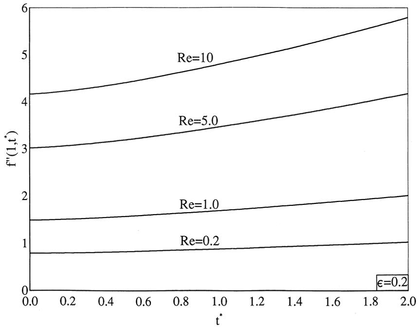
Fig. 2. Variation of the surface shear stress  $f''(1, t^*)$  with time  $t^*$  for  $\phi(t^*) = 1 + \epsilon t^{*2}$ ,  $\epsilon = 0.2$ ,  $Re = 0.2, 1.0, 5.0, 10.0$ .
