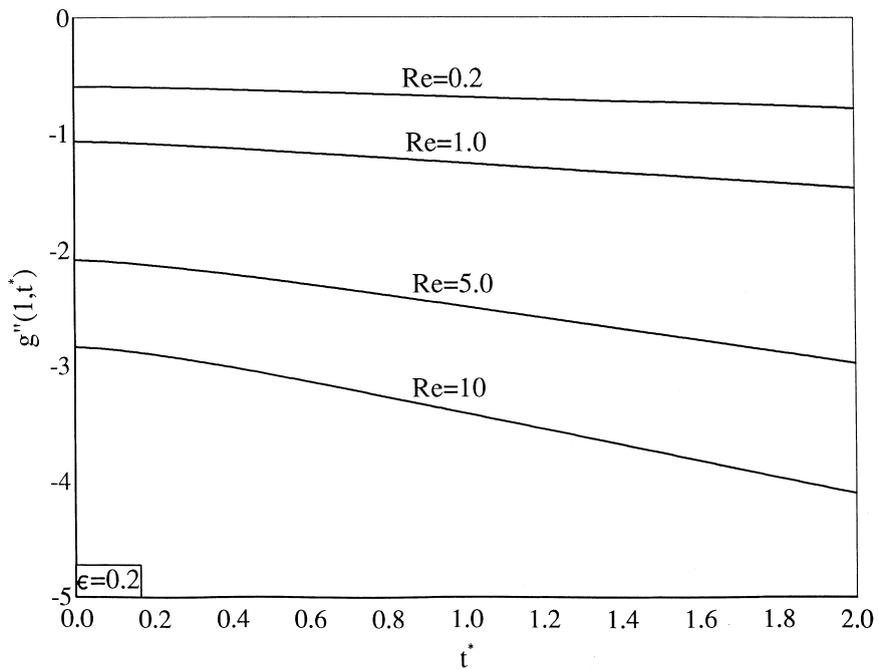
Fig. 3. Variation of the surface shear stress  $g''(1, t^*)$  with time  $t^*$  for  $\phi(t^*) = 1 + \epsilon t^{*2}$ ,  $\epsilon = 0.2$ ,  $Re = 0.2, 1.0, 5.0, 10.0$ .
