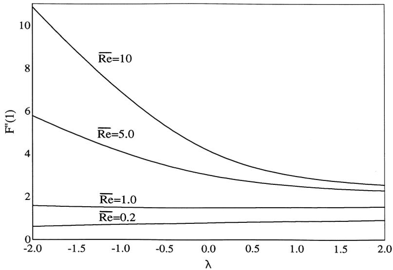
Fig. 11. Variation of the surface shear stress  $F''(1)$  with  $\lambda$  and  $\overline{Re}$ .
