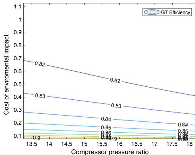
**Fig. 7** Effect of compressor compression coefficient change on cost of pollutant effects
