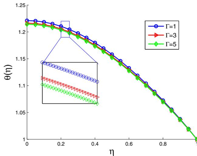
**Fig. 9.** The effect of fluid parameters on temperature profile when  $S = 5$ ,  $Ha = Pr = \gamma = 1$ ,  $Sc = Q = R = 0.1$  and  $\delta = 0.01$ .
