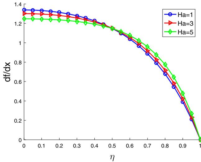
Fig. 4. The effect of Hartman numbers on velocity profiles when  $\Gamma = S = Pr = \gamma = 1$ ,  $Sc = R = Q = 0.1$  and  $\delta = 0.01$ .
