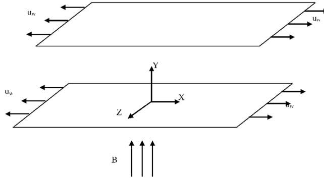
Fig. 1. The schematic of the problem, Eyring–Powell fluid between two walls.
