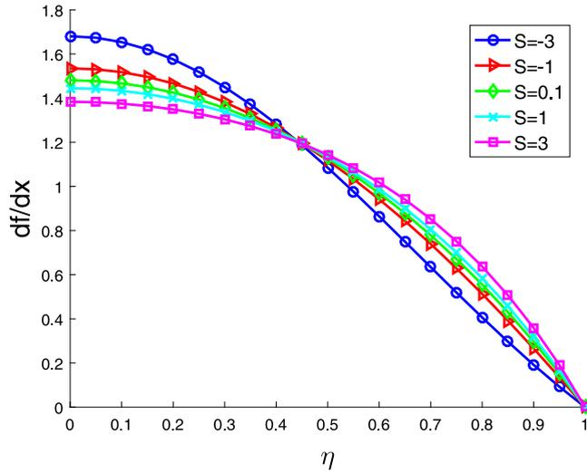
Fig. 3. The effect of squeezing parameters on velocity profiles, when  $\Gamma = S = Ha = Pr = \gamma = 1$ ,  $Sc = R = Q = 0.1$  and  $\delta = 0.01$ .
