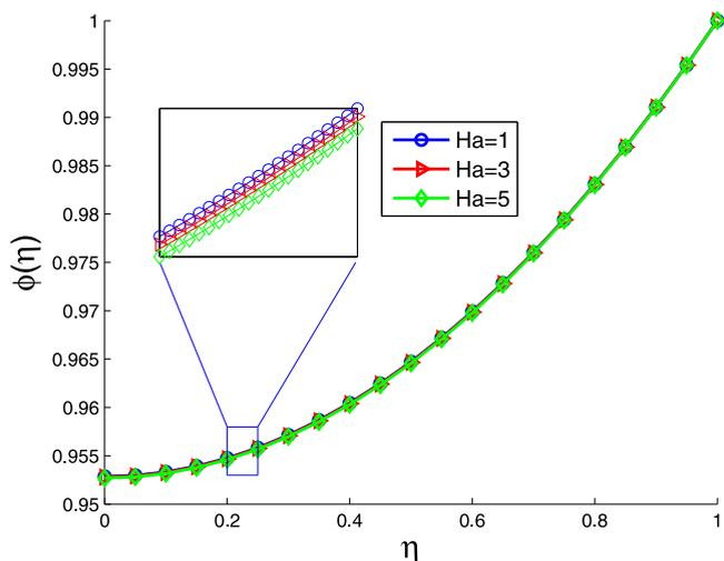
**Fig. 5.** The effect of Hartman numbers on the concentration profiles, when  $S = 5$ ,  $\Gamma = Pr = \gamma = 1$ ,  $Q = R = Sc = 0.1$  and  $\delta = 0.01$ .
