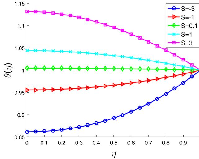
Fig. 2. The effect of squeezing parameter on the temperature profiles, when  $\Gamma = S = Ha = Pr = \gamma = 1$ ,  $Sc = R = Q = 0.1$  and  $\delta = 0.01$ .
