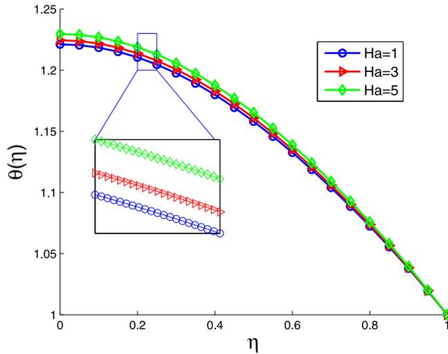
Fig. 10. The effect of Hartman numbers on temperature profile when  $S = 5$ ,  $\Gamma = Pr = \gamma = 1$ ,  $Sc = Q = R = 0.1$  and  $\delta = 0.01$ .
