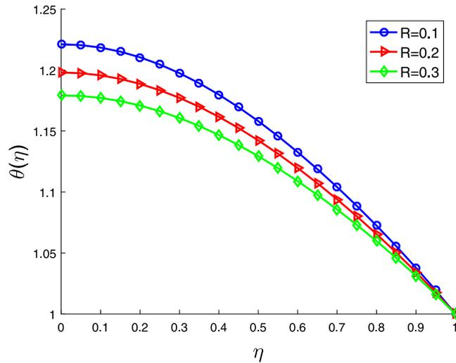
**Fig. 8.** The effect of radiation parameters on temperature profiles when  $S=5$ ,  $\Gamma = Ha = Pr = \gamma = 1$ ,  $Sc = Q = 0.1$  and  $\delta = 0.01$ .
